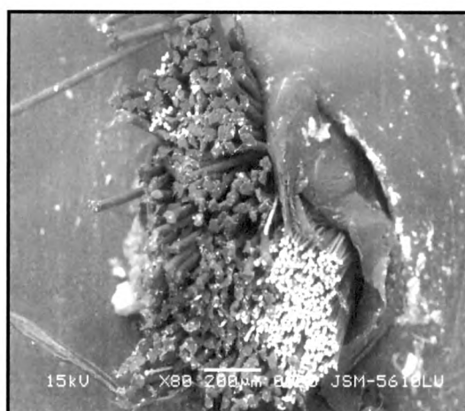
Fig. 5.12(c) SEM of hybrid yarn: Passage 2 (50 m/min, 6 bar)
