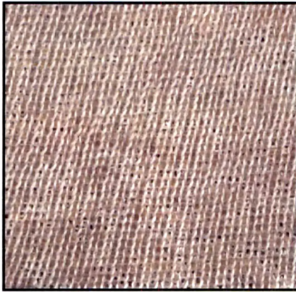
Fig. 7.12 (b) Laminates made from hybrid wrapped yarn with commingled core
