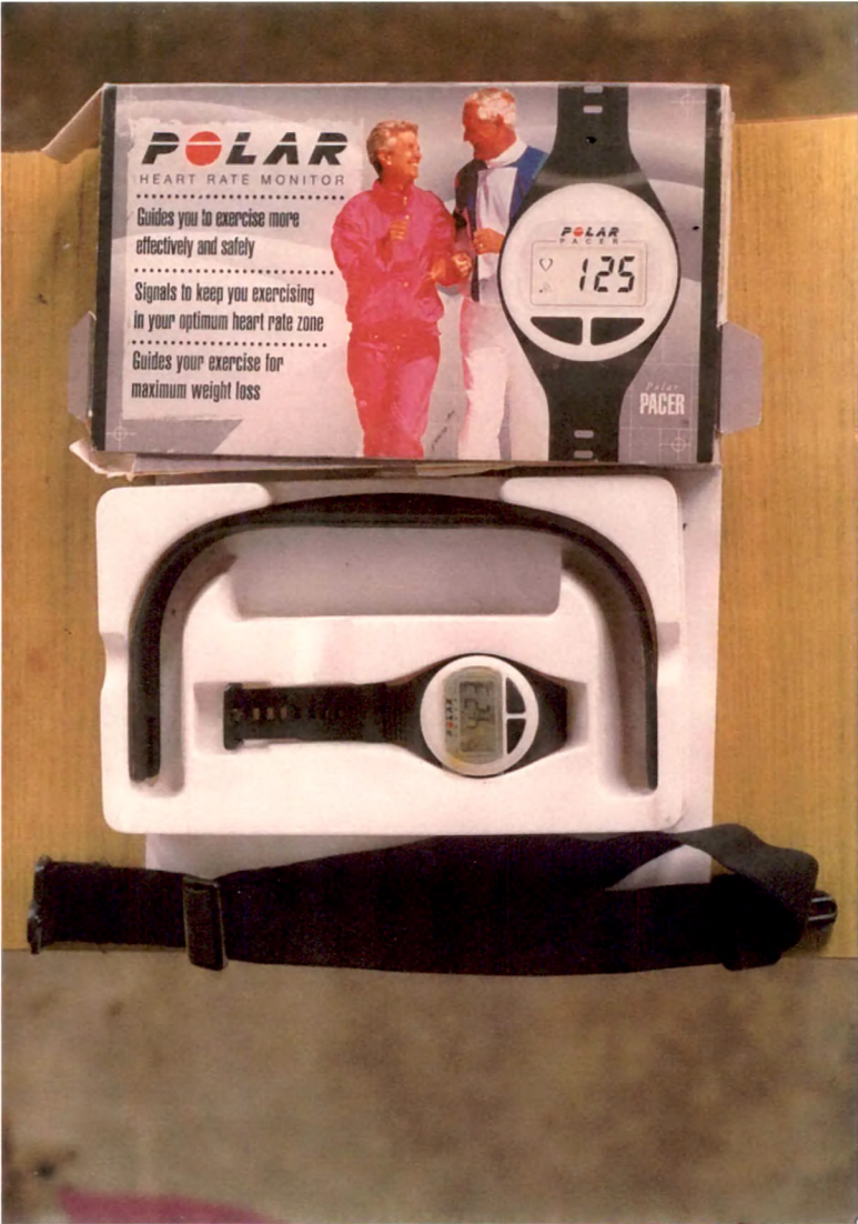
Fig 3.8 Polar Heart Rate Monitor used for Physiological Cost (Heart Rate, beats/min)
