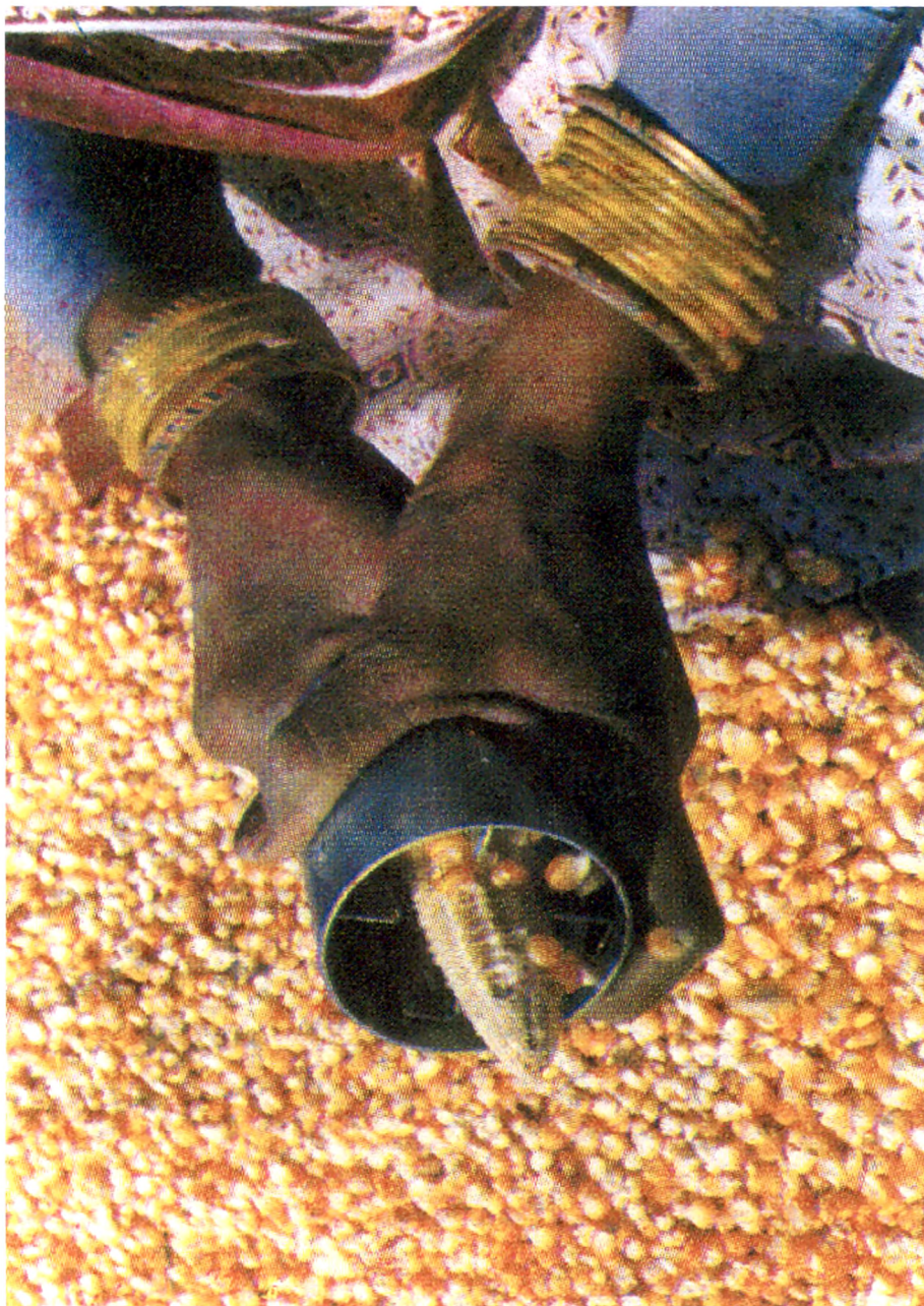
Fig 4.48 Modified Technology for Dehusking Grains (Tubular Maize Sheller) (Source: C.I.A.E., Product Catalogue 2002)
