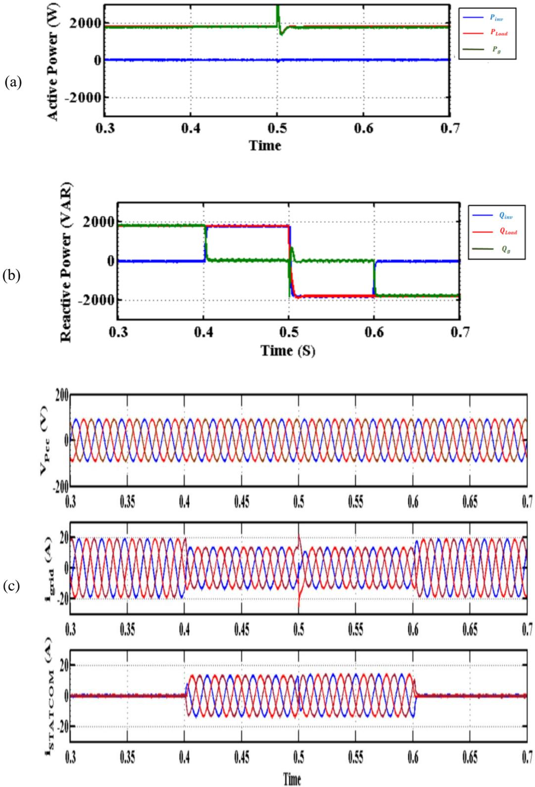
Figure 4- 10 : Dynamic performance of multipurpose single-stage PV system during Full-STATCOM mode
