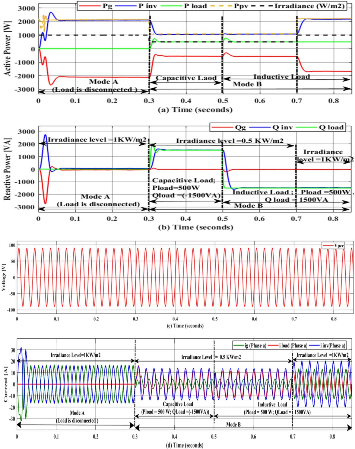
Figure 4- 13 : Simulation results of MODE A and MODE B(a)Active Power of  $P_g$ ,  $P_{inv}$  and Irrriandance ( $Irr, \frac{w}{m^2}$ ), (b) Reactive Power of  $Q_g$ ,  $Q_{inv}$ ,  $Q_{load}$  (c) PCC voltage (Phase a) and, (d)grid current, inverter current , load current.
