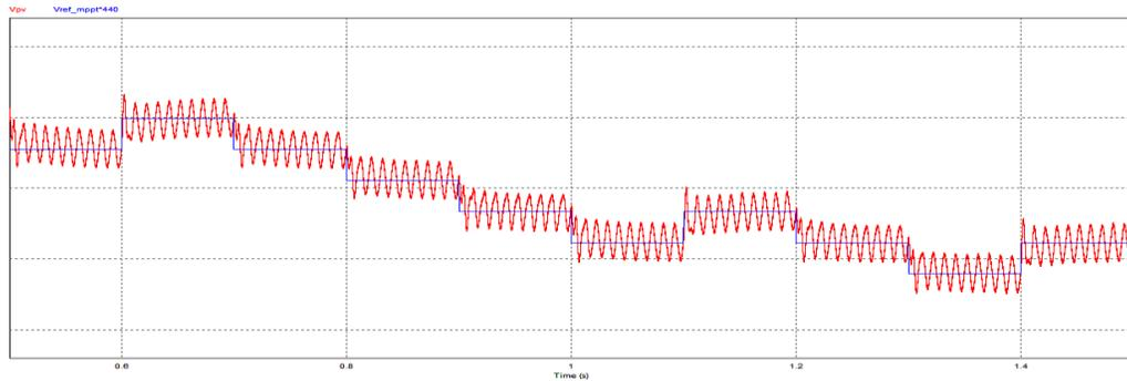
**Figure 4- 27 : Tracking the change in  $V_{pv}$  [Upper Trace: Voltage Generated by PV Array (Red): X axis: 1 Div. = 20 mSec, Y axis : 1 Div. = 5 V; Lower Trace: Reference Voltage Generated by MPPT Algorithm (Blue): X axis : 1 Div. = 20 mSec, Y axis : 1 Div. = 5 V]**
