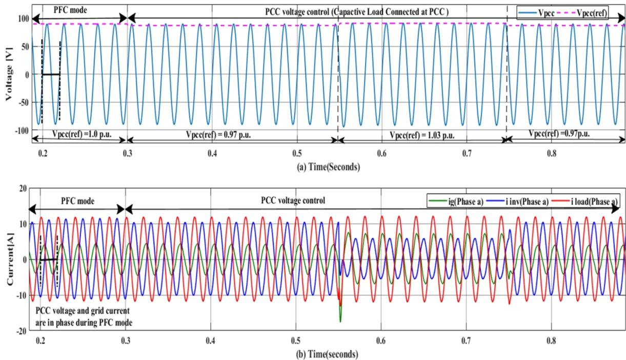
**Figure 4- 14 : Simulation result of Multipurpose PV system connected to capacitive load at PCC (a) PCC voltage(Phase A), and (b) grid current(Phase A),, inverter current(Phase A), and load current(Phase A).**
