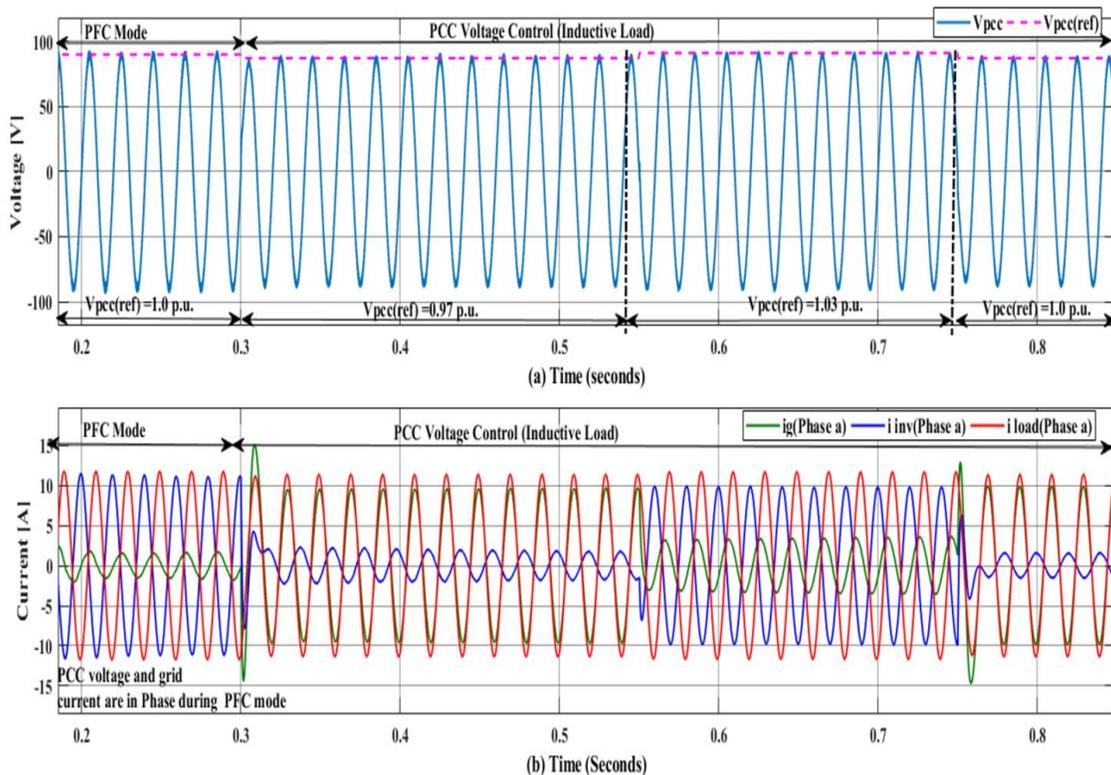
**Figure 4- 15 : Simulation result of Multipurpose PV system connected to inductive load at PCC (a) Phase A of PCC voltage, and (b)phase A of grid current, inverter current, and load current**
