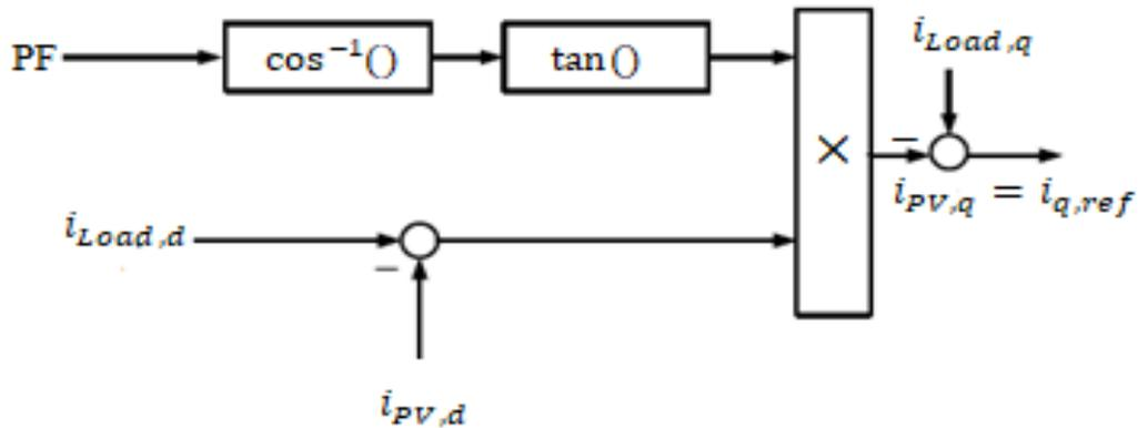
Figure 4- 5 : Block diagram for a Power factor correction
