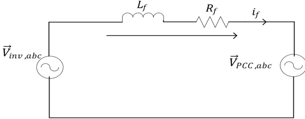
**Figure 4- 18 : Functional diagram of grid tied system**
