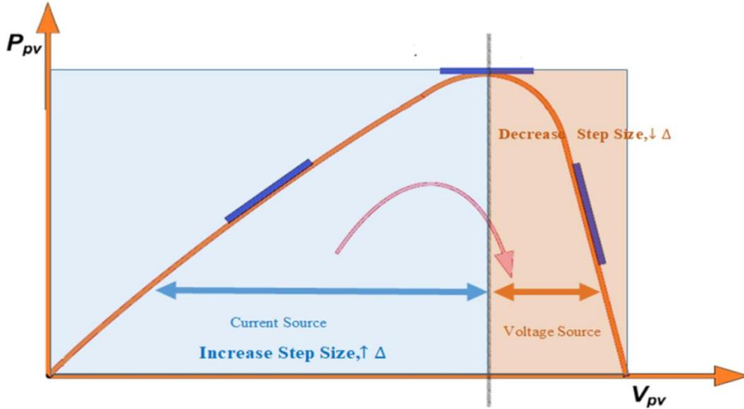
**Figure 4- 26 : Power curve for PV panel using modified dc current sensor-less MPPT**
