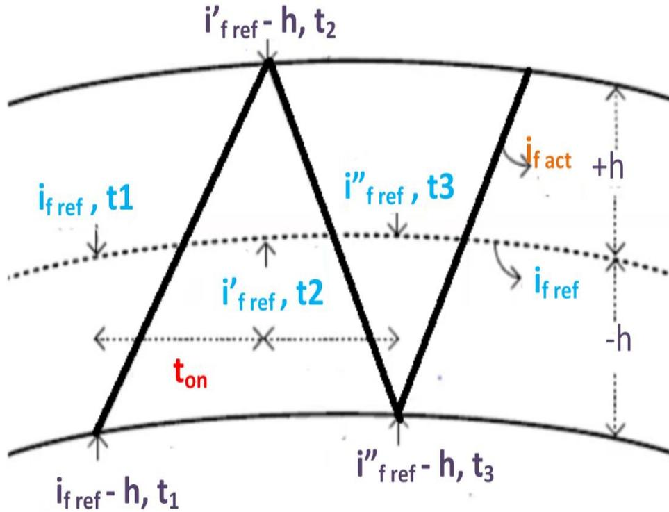
Figure 4- 17 : Hysteresis current control mechanisms
