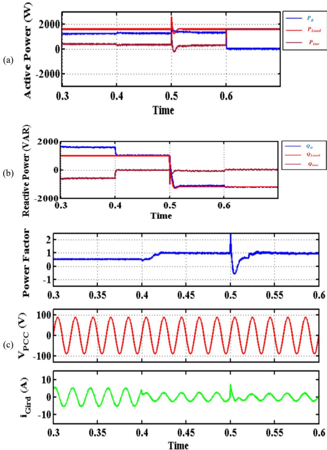
Figure 4- 11 : Dynamic performance of multipurpose single-stage PV system (PV-STATCOM) during power factor correction
