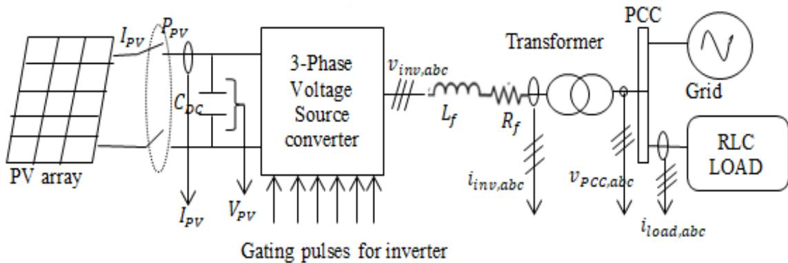
**Figure 4- 1 : A power circuit diagram of single stage grid tied PV system**
