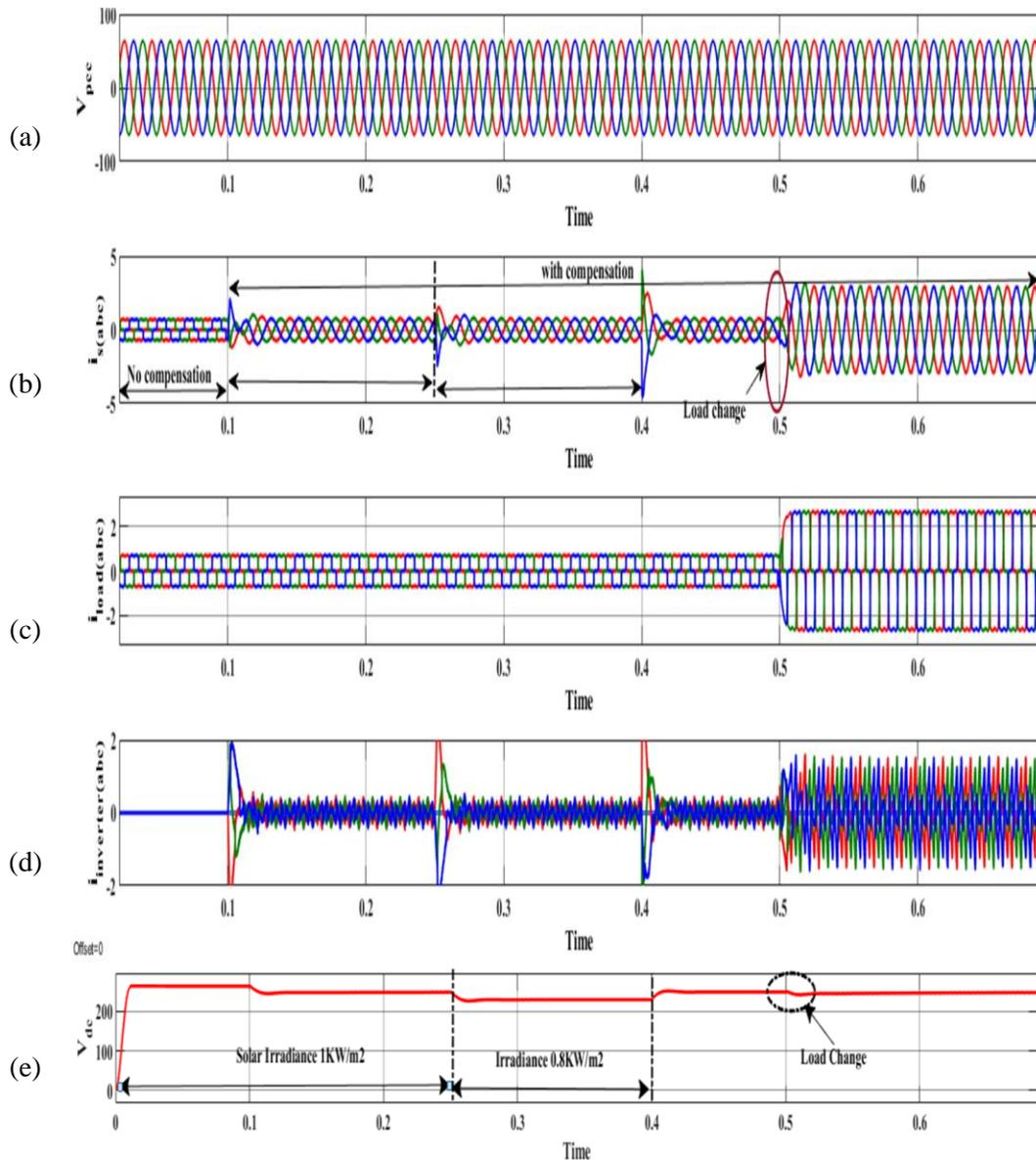
**Figure 4- 23 : Simulation result of Multipurpose PV system connected to non-linear load at PCC (a) PCC voltage, (b) grid currents, (c) inverter currents, (d) load currents, and (e) DC-bus voltage**
