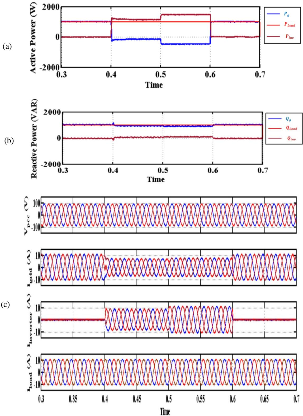
Figure 4- 7 : Dynamic performance of multipurpose single-stage PV system during full-PV mode (reverse power flow)
