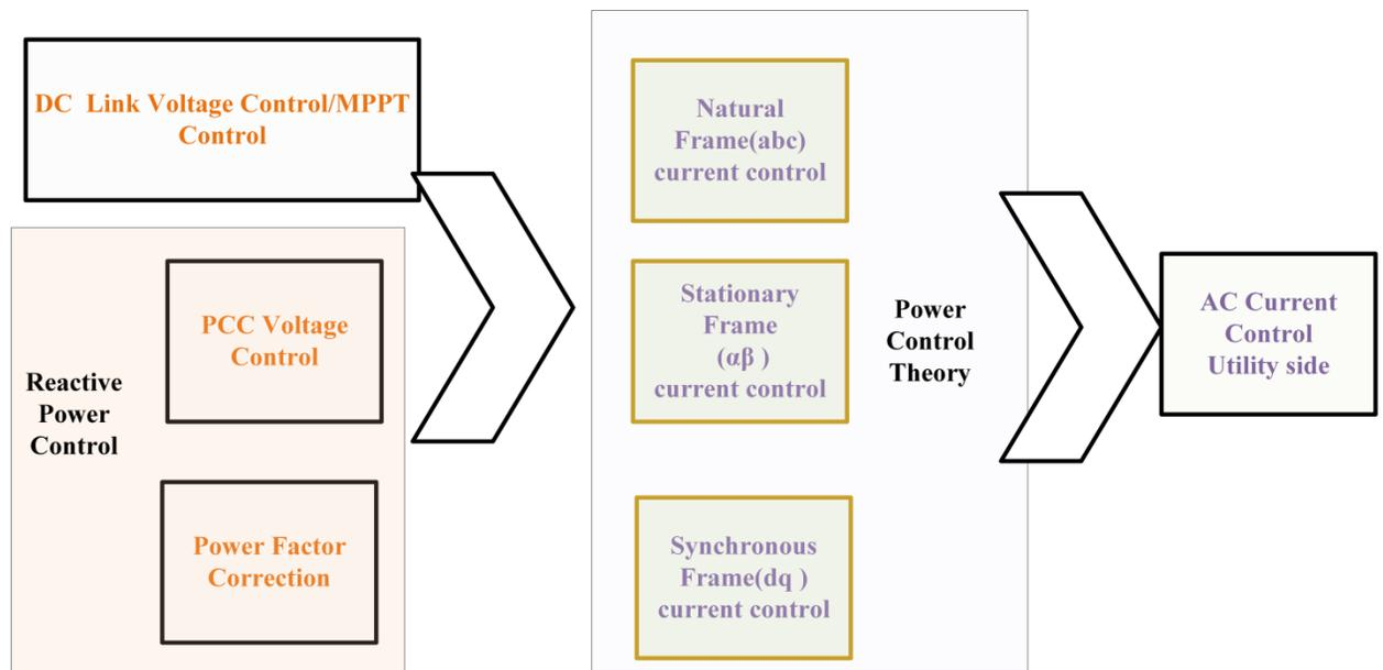
**Figure 4- 2 : Conceptual Power theory for grid tied PV system**
