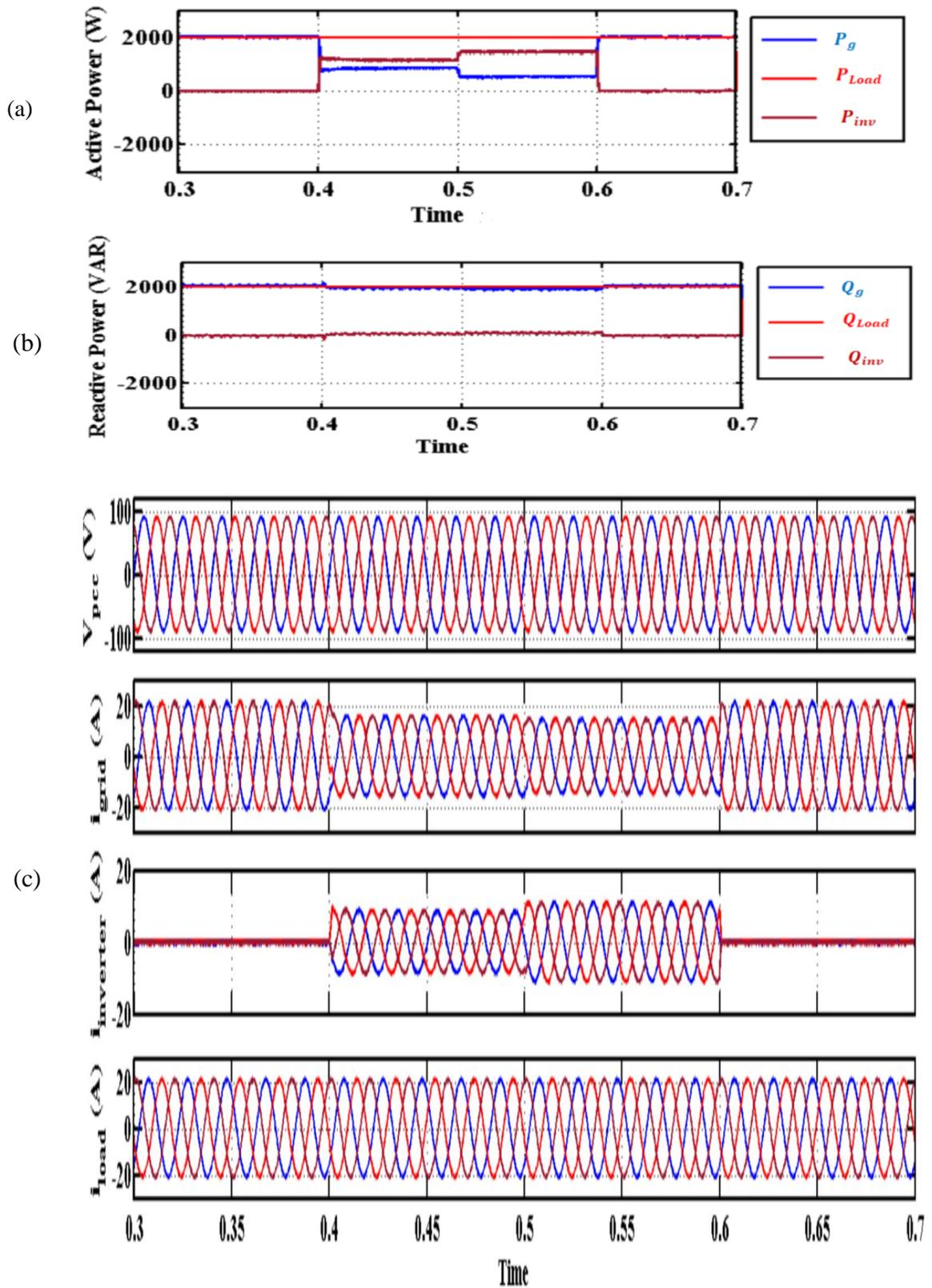
Figure 4- 8 : Dynamic performance of multipurpose single-stage PV system during full-PV mode (forward power flow)
