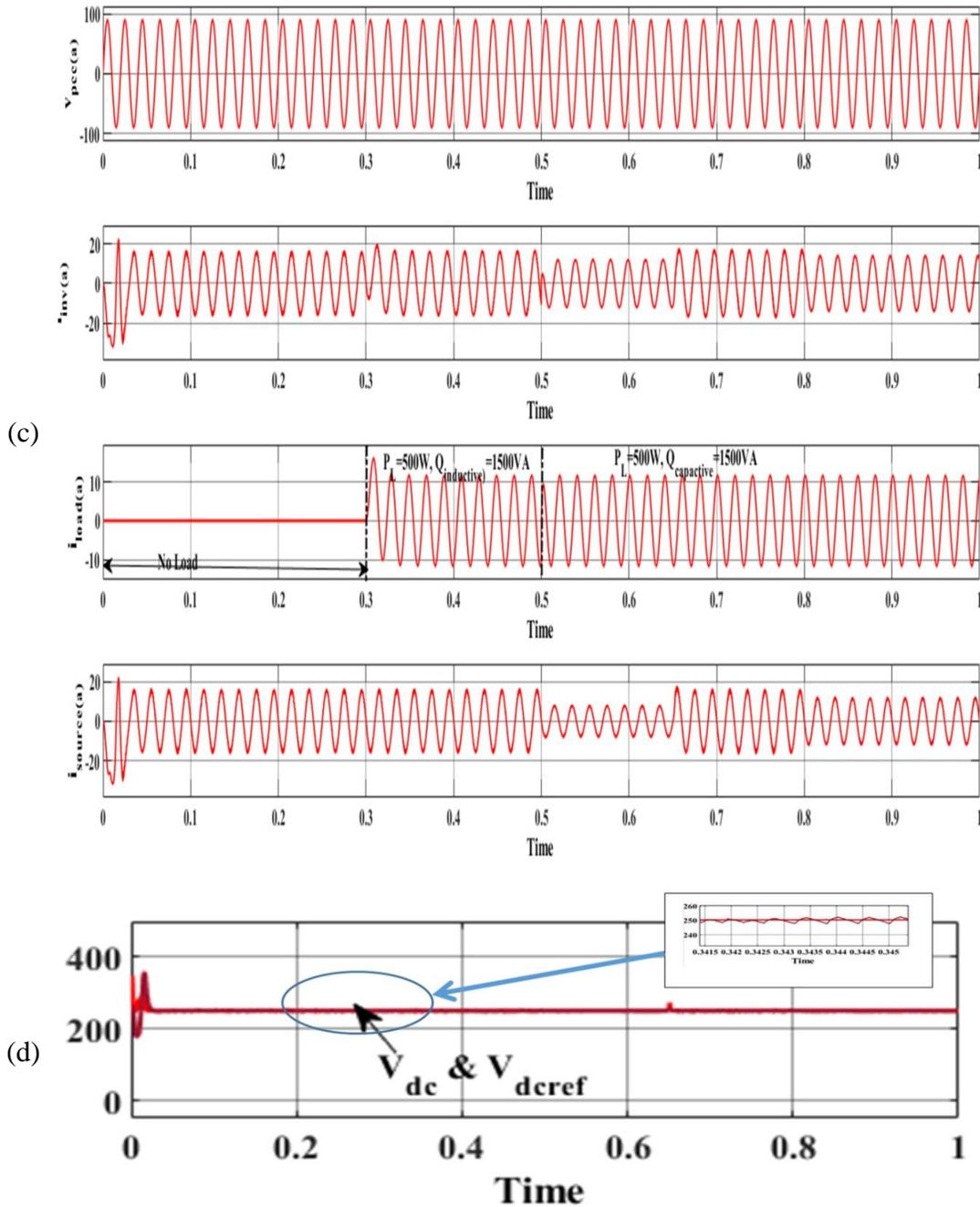
**Figure 4- 28 : Dynamic performance of Multipurpose PV system using a modified DC current sensor-less MPPT and synchronous frame current control**
