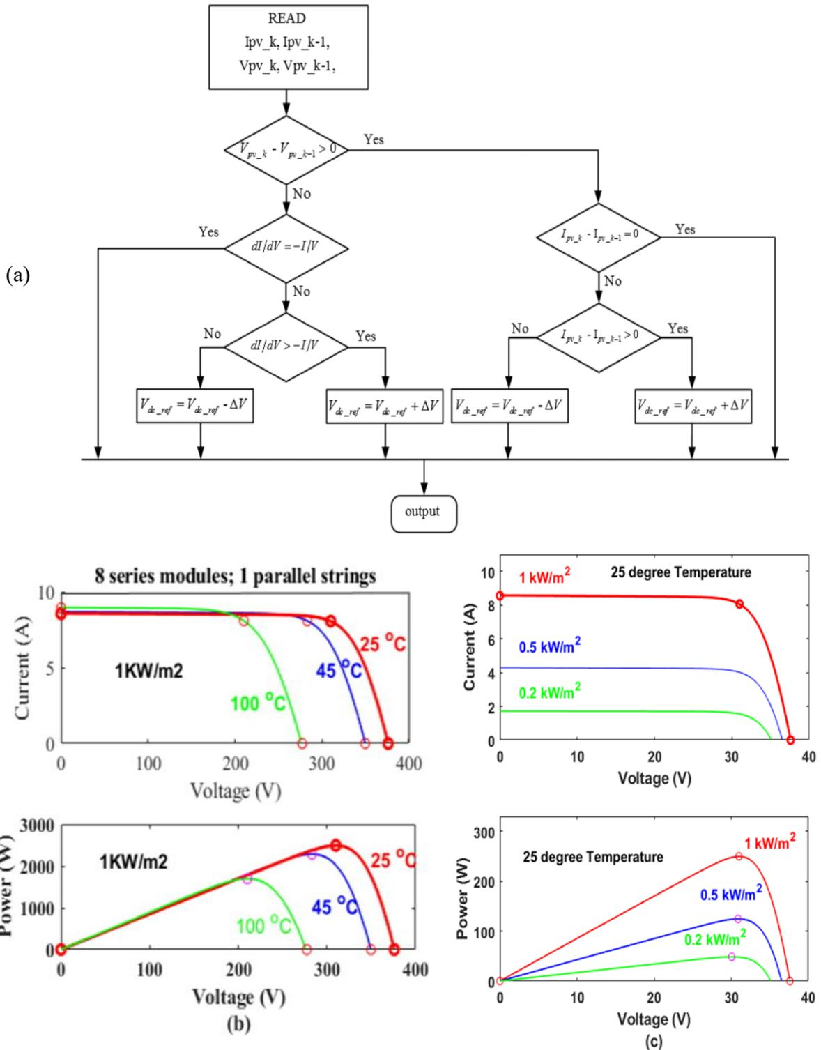
Figure 4- 4 : Flow-chart of Increment-conductance MPPT algorithm,(b) PV characteristic of PV panel with different temperature, and (c) PV characteristic of PV panel with different solar irradiance
