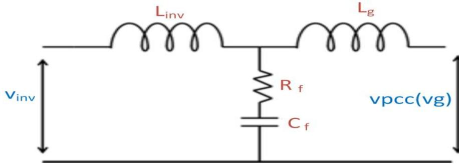
**Figure 4- 19 : Basic block schematic of LCL type filter**
