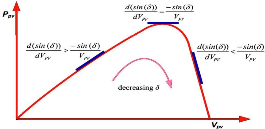
**Figure 4- 25 : Power curve for PV panel using sin angle based DC current sensor-less MPPT**
