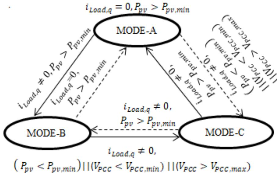
Figure 4- 6 : Control for mode of operation
