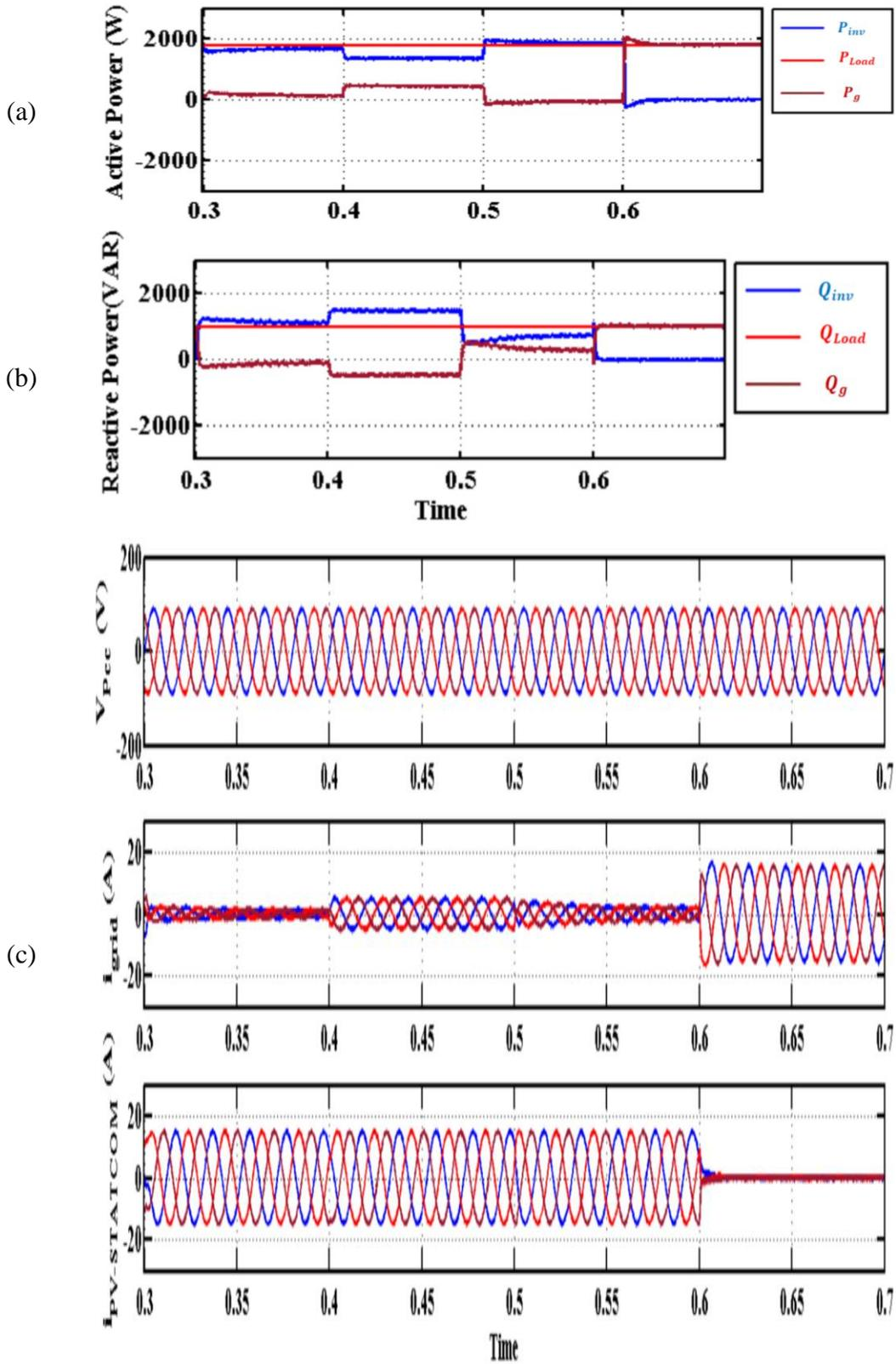
Figure 4- 9 : Dynamic performance of multipurpose single-stage PV system during Partial PV & Partial-STATCOM mode
