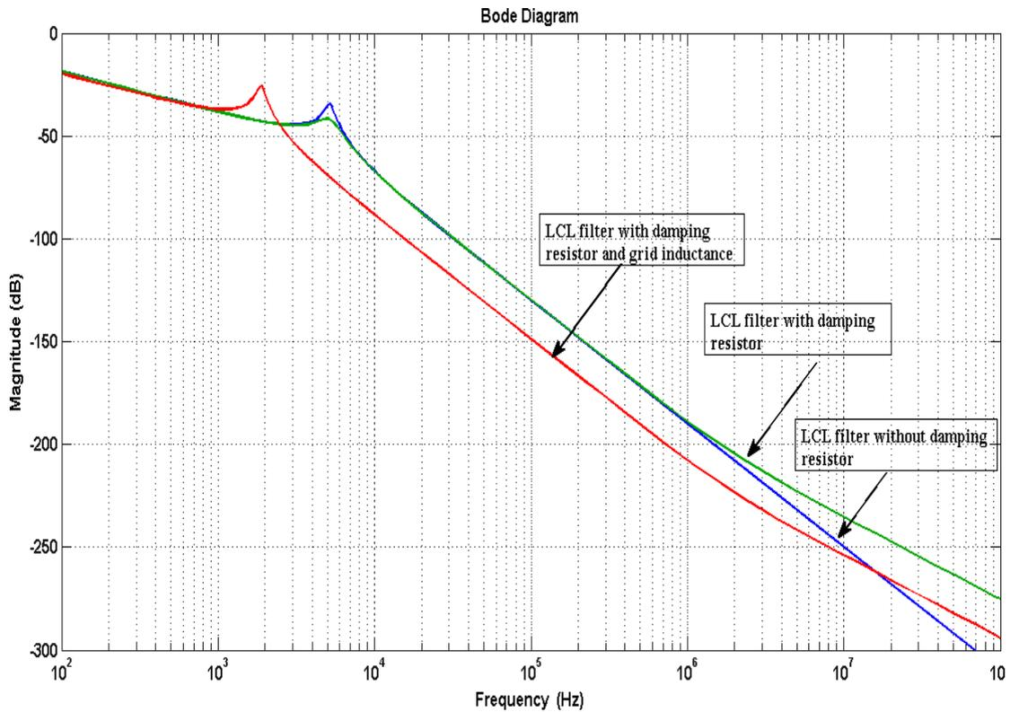
Figure 4- 21 : Bode plot for LCL type filter considering different conditions
