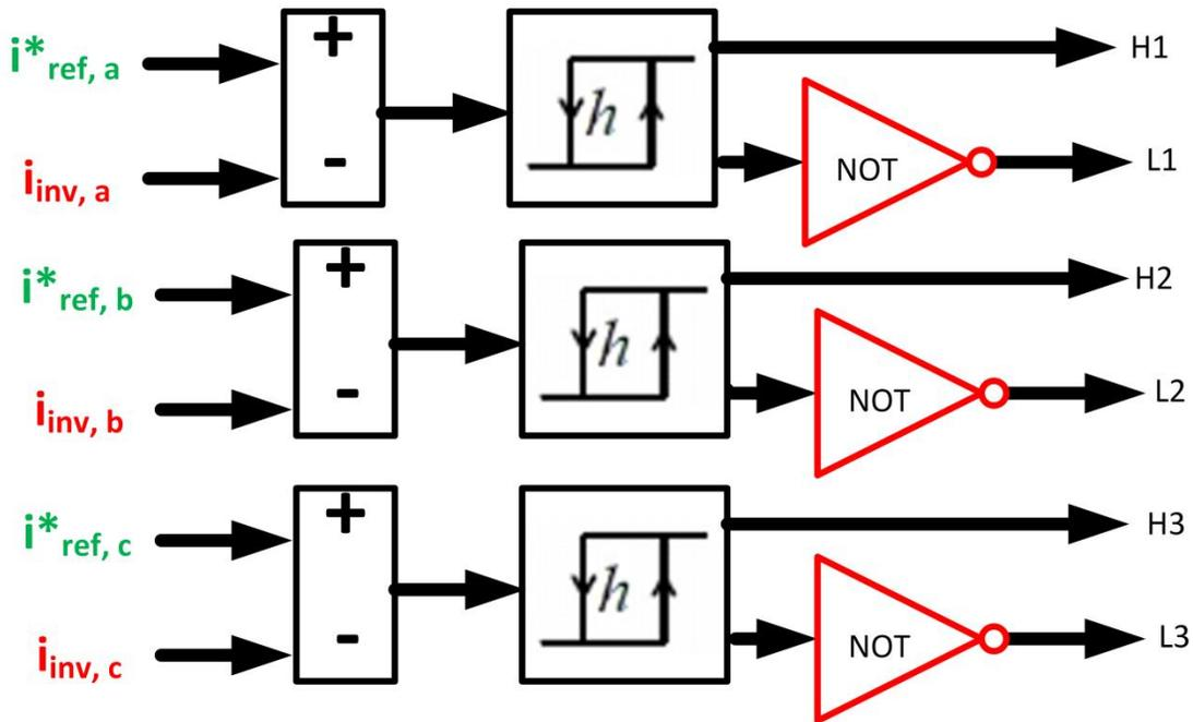
Figure 4- 16 : Functional diagram of Hysteresis current controller
