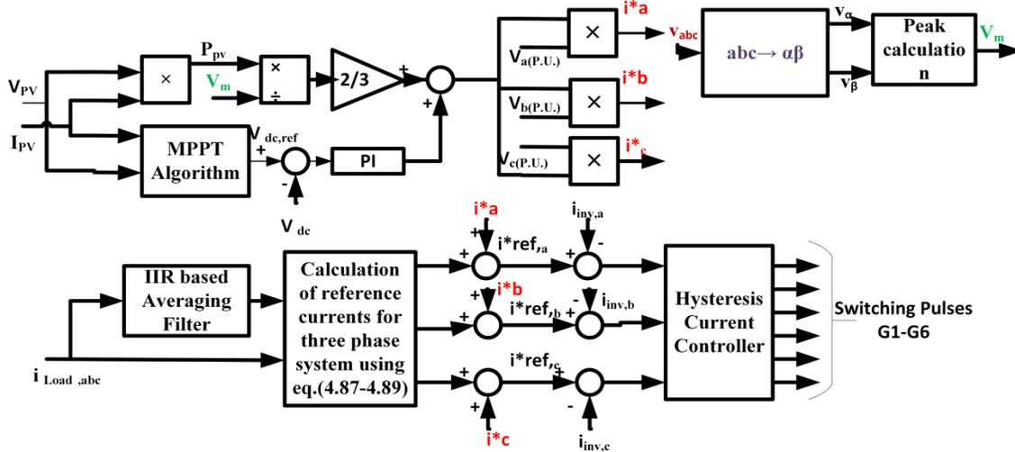
Figure 4- 22 : Control mechanism of single stage grid tied PV system in abc reference frame
