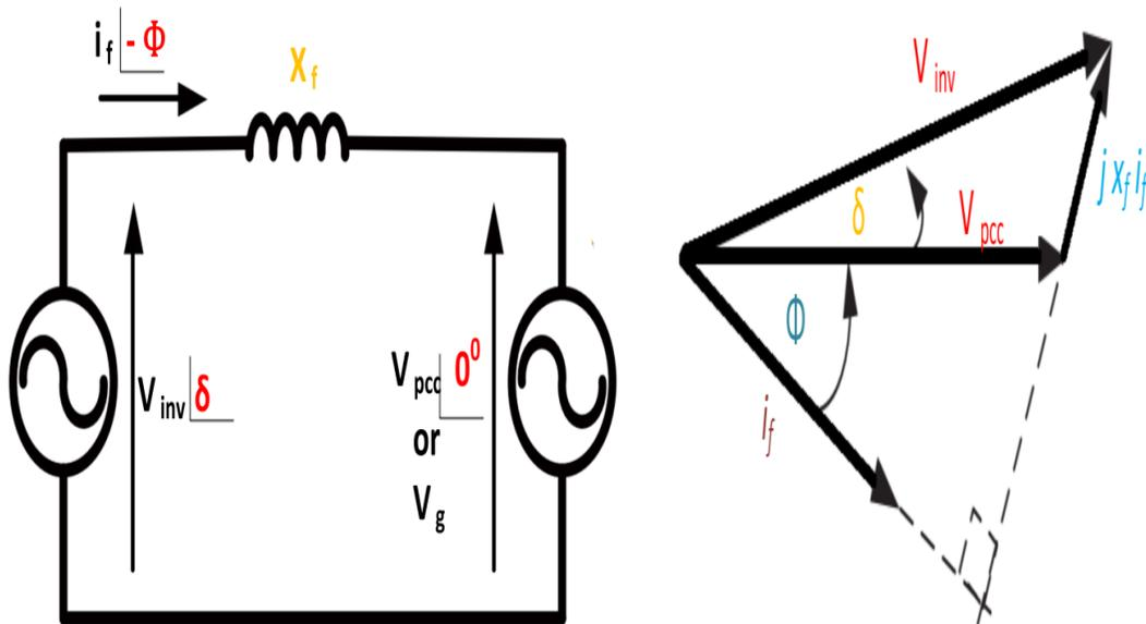
**Figure 4- 24 : Functional and Phasor diagram of grid tied PV system during power injection into a grid**
