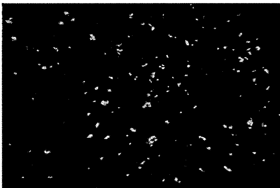
Figure 186 Photomicrograph of neat Gandhar crude oil at room tempeprature
