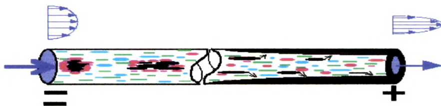
Figure: 14 Electrokinetic deposition in an isothermal-single phase pipeline flow
