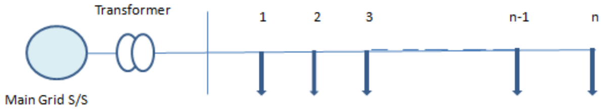
Figure 4.2: Single line diagram of radial distribution system.
