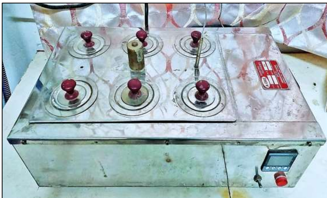
Figure 3.29: Electrical heater [A-ONE Scientific equipments, Volts: 230, Watts: 1500]
