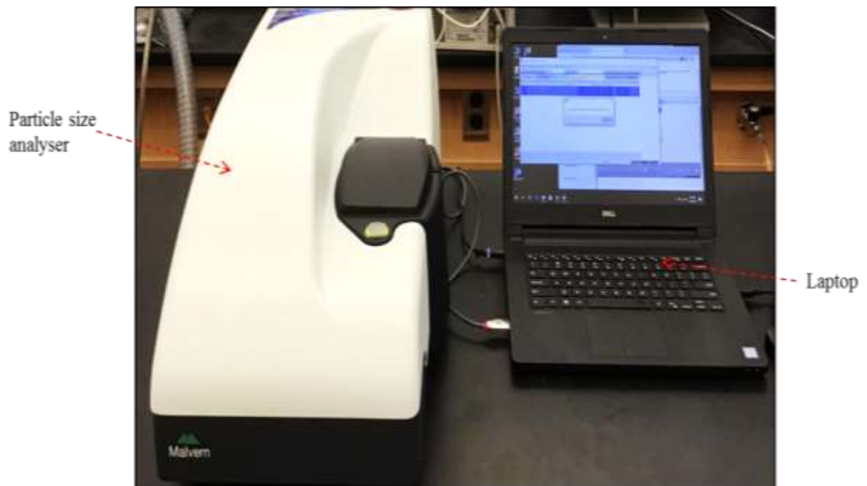
Figure 3.25: Particle size analyser, Model- Malvern Zetasizer Pro, Version 7.11
