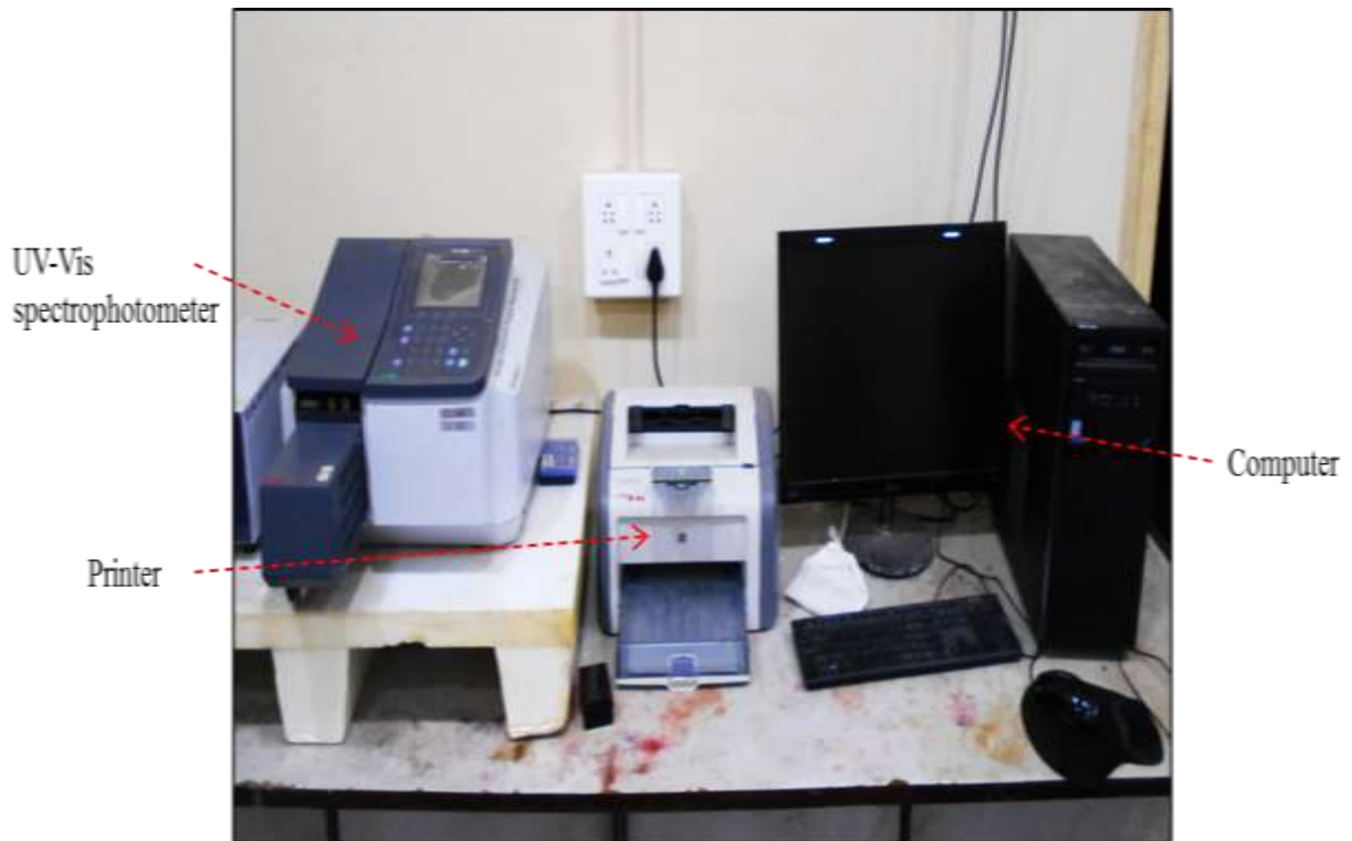
Figure 3.24: Shimadzu UV-Vis spectrophotometer, Model UV-1800
