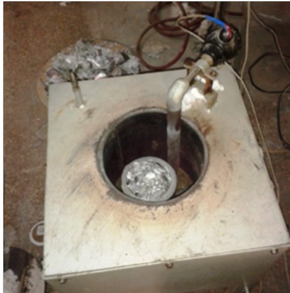
Figure 3.5: Placing and setting up the crucible filled with charge materials in the resistance heating furnace.
