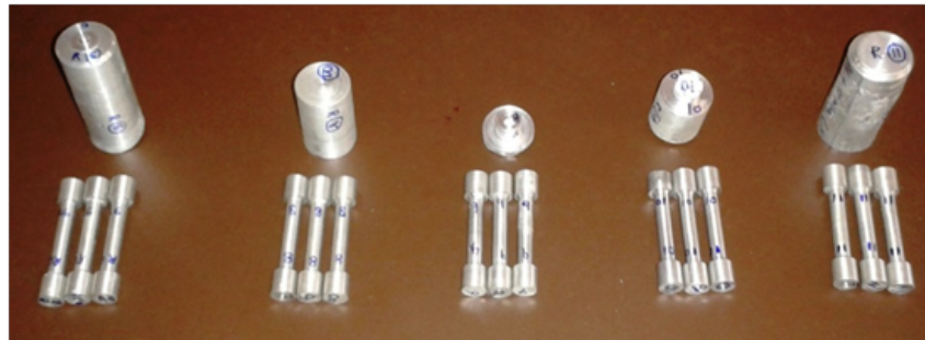
Figure 3.12: Preparation of tensile specimens.
