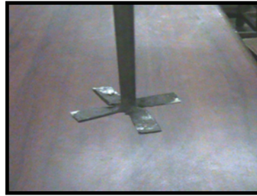
Figure 3.2: Four blade turbine type stainless steel stirrer used in present work.
