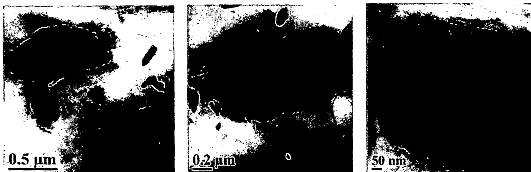
Fig. 5.9- TEM images of nanocomposite with 7 phr organoclay.
