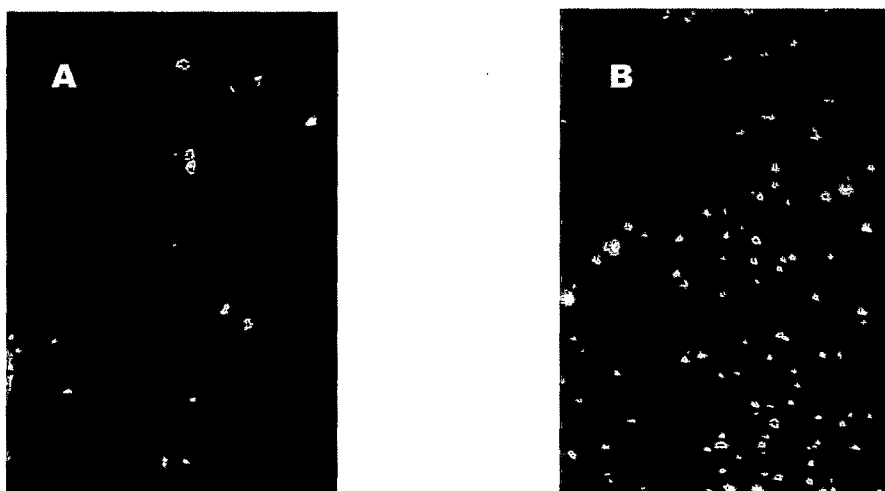
Fig. 5.10-(A) Organoclay-carbon black and (B) Organoclay-silica filler dispersion
