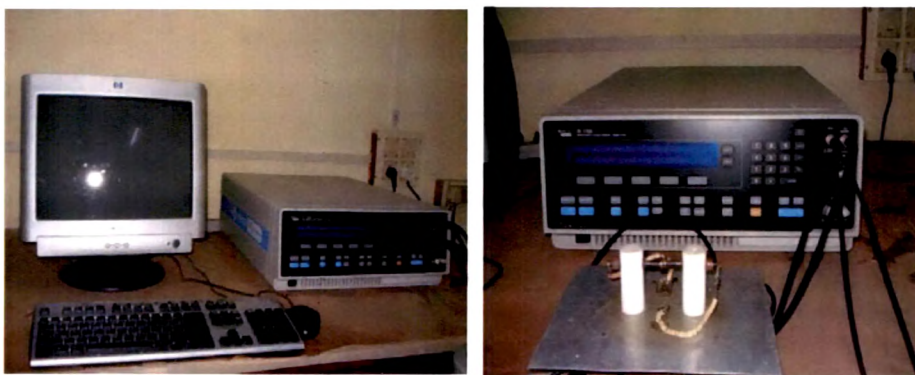
Fig. 2.5 Impedance gain/phase analyser (Solartron 1260)
