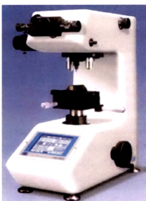
Fig. 2.7 Vicker's Microhardness Indenter Future Tech. (FM-700)
