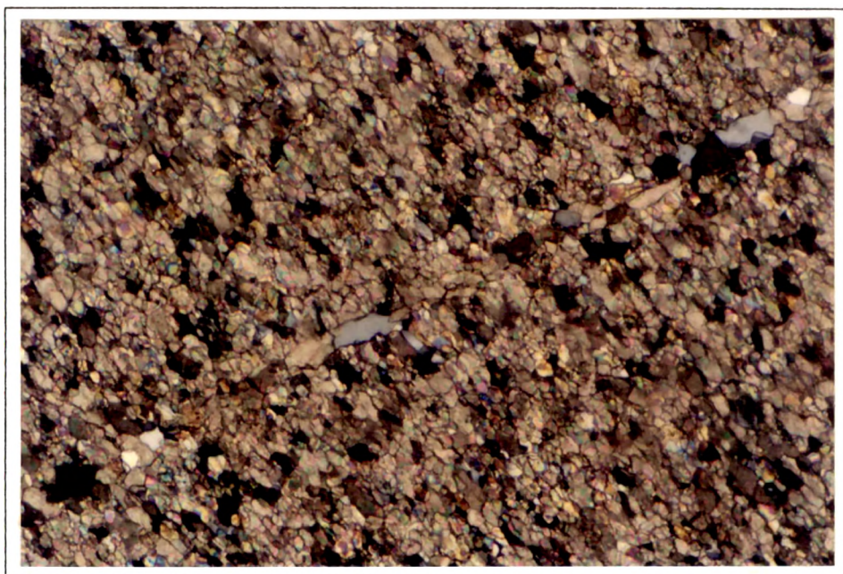
Fig. 3.4: Sample # KU92-26 was collected from near MCT. Grains are euhehedral equant and elongated. Schistosity has developed due to pressure. Quartz rich veins following the schistosity plane as well as cross-cutting are suggestive of later neomorphism giving a pseudo-marble. Magnification 40X, Cross Nicols.
