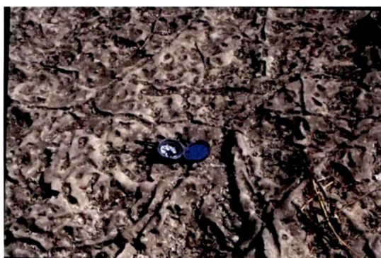
Figure 5.2 Orthogonal joints in the miliolite limestone in Rupen river bed near Chikhali. (Diameter of compass 8cm)
