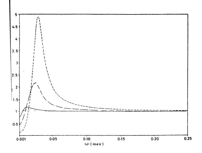
Fig. 3.2 The  $\sigma_R^L(\mathbf{q}, \mathbf{q}_z, \omega)/\sigma_d(\omega)$  (solid line curve for  $\mathbf{q}d=0.001$  and dash-dash curve for  $\mathbf{q}d=0.005$ ) and  $\sigma_R^T(\mathbf{q}, \mathbf{q}_z, \omega)/\sigma_d(\omega)$  (dot-dot curve for  $\mathbf{q}d=0.001$  and dash-dot curve for  $\mathbf{q}d=0.005$ ) plotted as a function of  $\omega$  at  $\gamma = 8.475 \times 10^{-3}$  meV,  $n_s = 10^{12}$  cm<sup>-2</sup> and  $\cos(\mathbf{q}_z d)=1$ .
