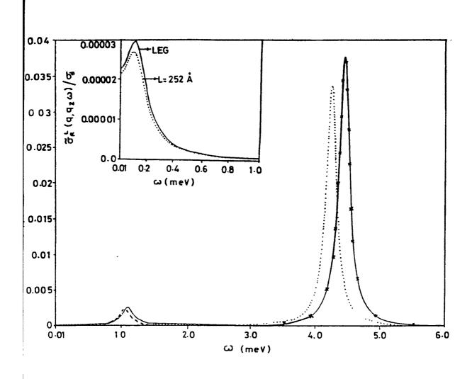
Fig. 3.4 The  $\vec{\sigma}_{R}^{L}(\mathbf{q},\mathbf{q}_{z},\omega)/\sigma_{d}$  is plotted as a function of  $\omega$  for qd=0.01 (inset curve) qd=0.1(dashed curve for L=252 Å and solid line curve for LEG) and qd=0.4 (dot-dot curve for L=252 Å and solid line curve with crosses for LEG) at  $\cos(q_{z}d)$ = -1, n<sub>s</sub>=7 3 x10<sup>11</sup> cm<sup>-2</sup> and  $\gamma$ =0.1meV.
