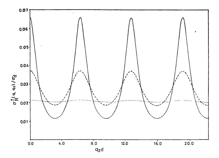
Fig. 3.3 A plot of  $\sigma_R^{\tau}(q,q_z)/\sigma_d$  versus  $q_z d$  for qd=1.0 (solid line curve), qd=2.0 (dash-dash curve) and qd=5.0 (dotted curve) at  $\cos(q_z d)=-1$ ,  $n_s=3.0 \times 10^{11}$  cm<sup>-2</sup> and  $\gamma=0.1$ meV
