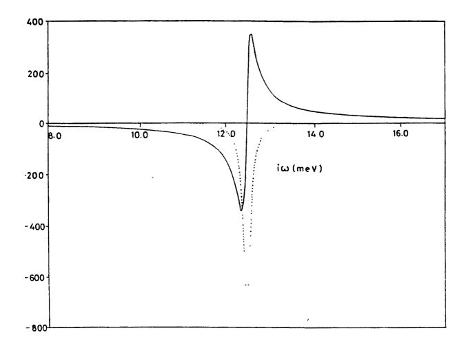
**Fig 3.5b** The  $\tilde{\sigma}_{R}^{T}(\mathbf{q},q_{z},\omega)/\sigma_{d}$  (solid line) and  $\tilde{\sigma}_{I}^{T}(\mathbf{q},q_{z},\omega)/\sigma_{d}$  (dotted curve) for  $\mathbf{q}d=0.1$ ,  $q_{z}d=0.1$  and  $\gamma=0.1$  meV are plotted as a function of  $i\omega$ .
