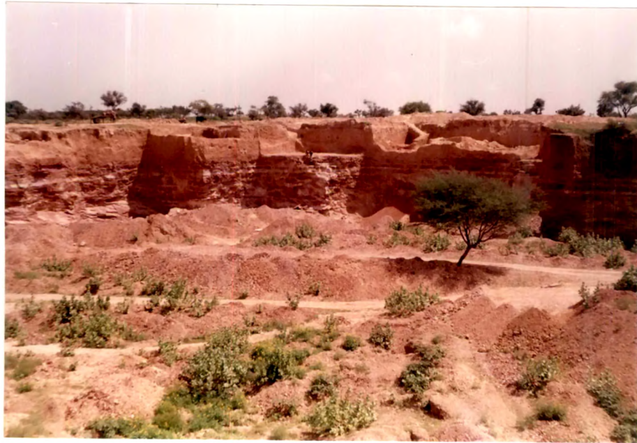
Plate II.1 A view of sandstone quarry belonging to Jodhpur Group of rocks, thick pedogenised aeolian silt is also seen overlying the sandstones. Location: Nimbi Jodhan
