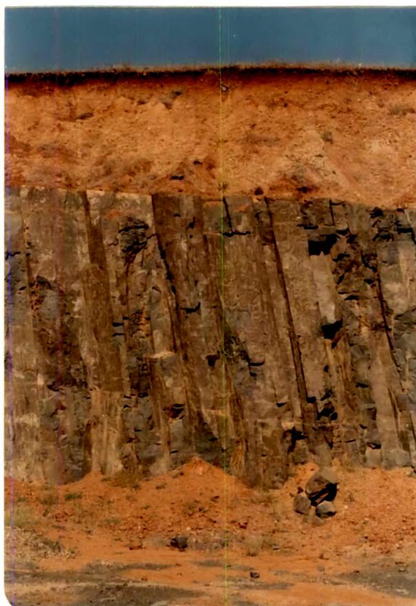
PLATE III.8 Columnar jointing in a quarry section in finegrained compact basalt. Location : Chikhli.
