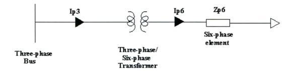
Fig. 6.2 A multi-phase (six-phase) element connected to three-phase bus bar
