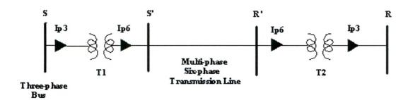
Fig 6.3 Schematic diagram of a multi-phase (six-phase) transmission Line
