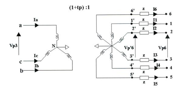
Fig. 6.1 A Wye / Star transformer of turns ratio (  $1 + t_p$ ) : 1
