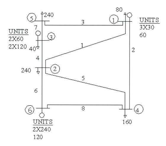
Fig. 6.4 Sample System having Three Phase Single and Double Circuits With Loads and Generations in MW
