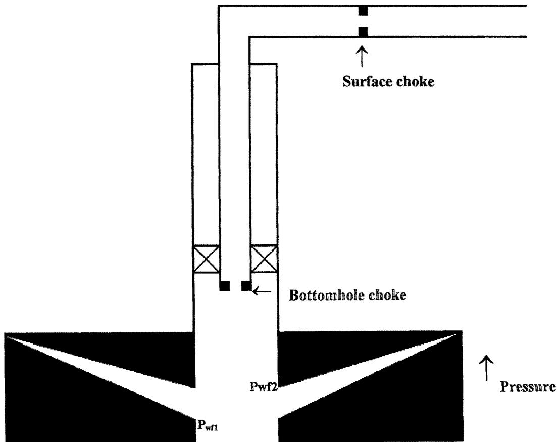
$P_{wf1}$  - Surface choke flowing bottomhole pressure
