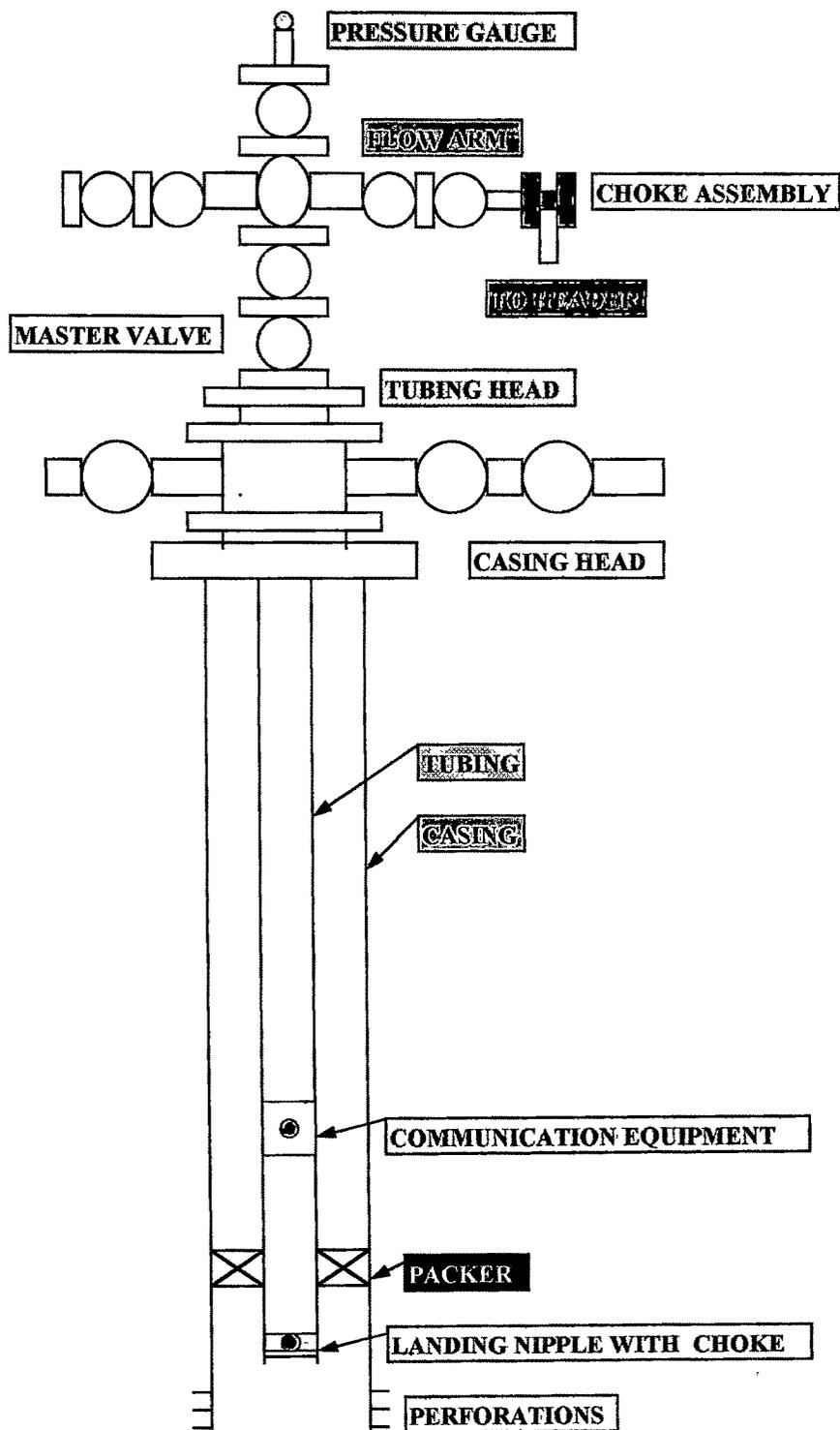
FIGURE - 5.1 DETAILS OF TYPICAL FIELD TRIAL SETUP ( BOTTOMHOLE CHOKE)
