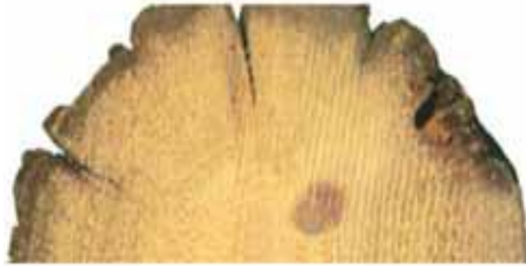
Fig. 3 Shallow depth of decayed wood by soft rot fungi (SRF) (Schwarze et al 2000)
