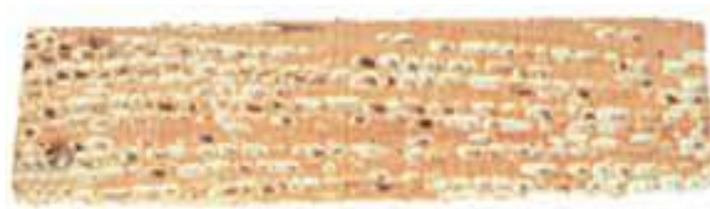
Fig. 7 Bleached appearance of wood due to decay caused by White rot fungi
