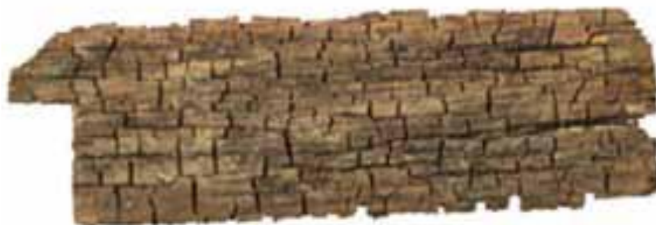
Fig. 5 Cubical checking and brown appearance of wood degrading by BRF (Schwarze et al 2000).
