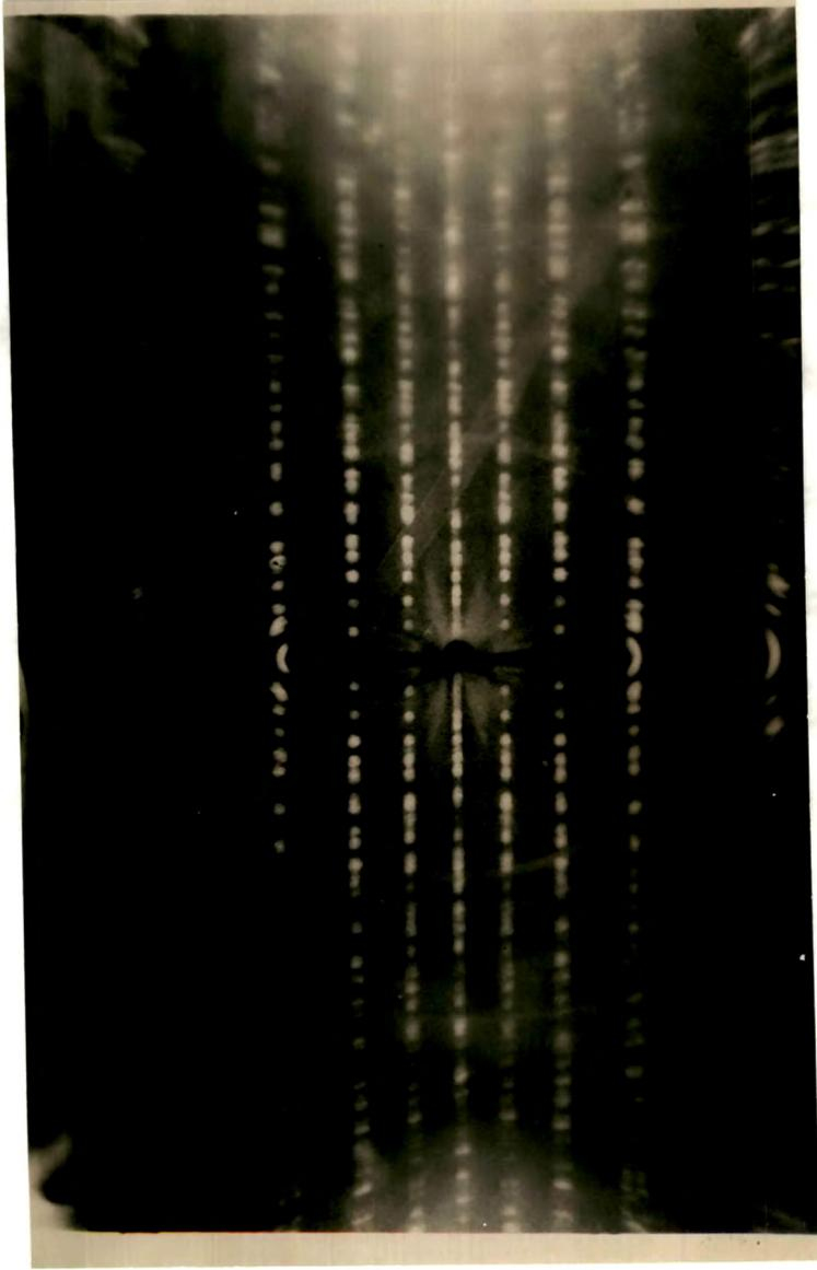
Fig. 5.6 -Single crystal rotation photograph of dAHT. CuK $\alpha$  radiation = 1.5418 Å
