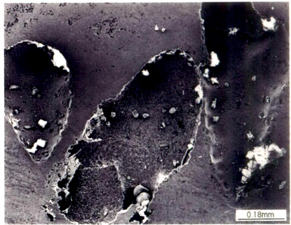
Figure - 5.8 : SEM Photomicrograph of SS 316 in 10% HCl
