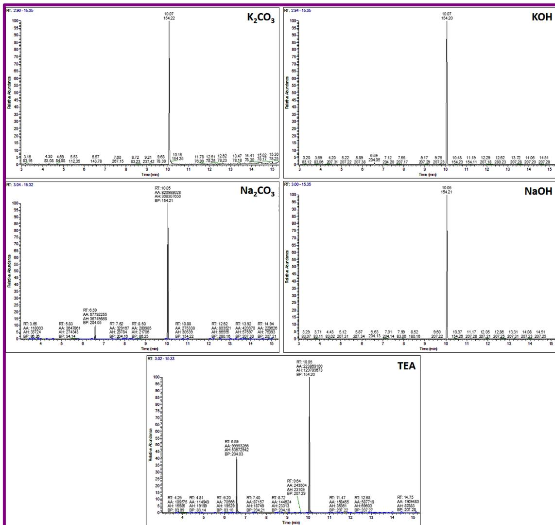
**Figure 6.A3:** GC-MS spectra of the product for Pd@IO-DTPA-DNA catalysed reaction between iodobenzene and phenylboronic acid performed using different bases and in Water as a solvent
