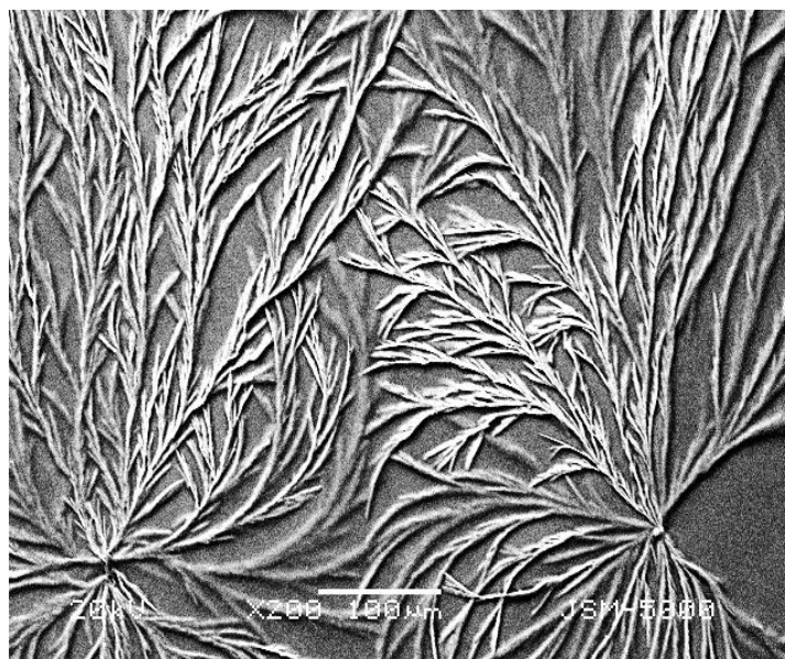
Figure 5.2: SEM analysis of the metallogel shows the presence of fibrous assembly.
