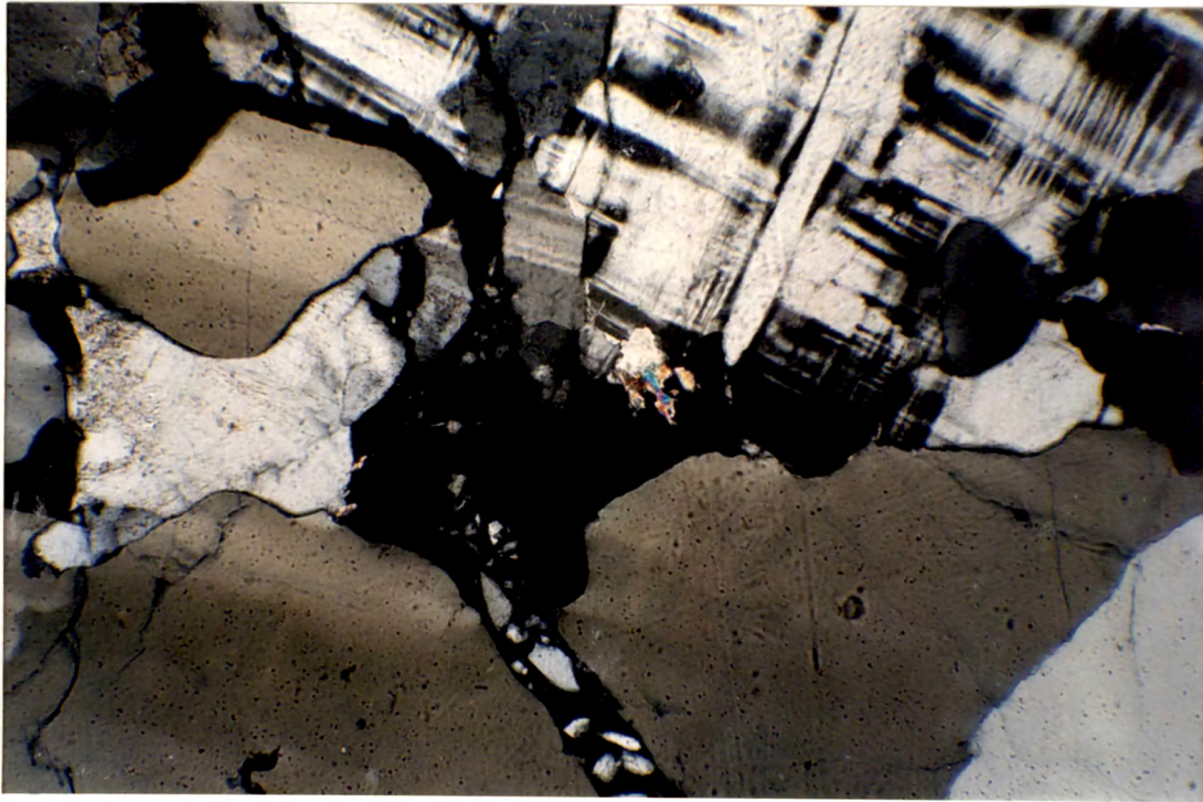
Plate IV.9 Photomicrograph showing squeezed quartz along microfractures (Crossed Nicols X 60)
