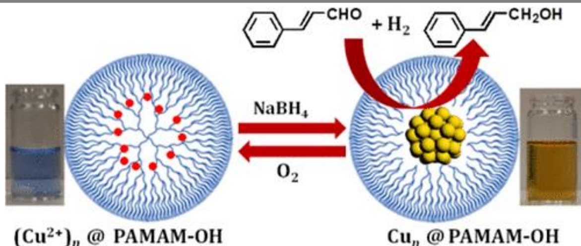
Figure 1.6: Schematic representation showing the copper nanoparticles encapsulated in poly(amidoamine) dendrimer with hydroxyl for hydrogenation of carbonyl and olefin group (Reproduced with permission from ACS Catal. 2013, 3, 2, 182–185, Copyright 2013, American Chemical Society.)[64]
