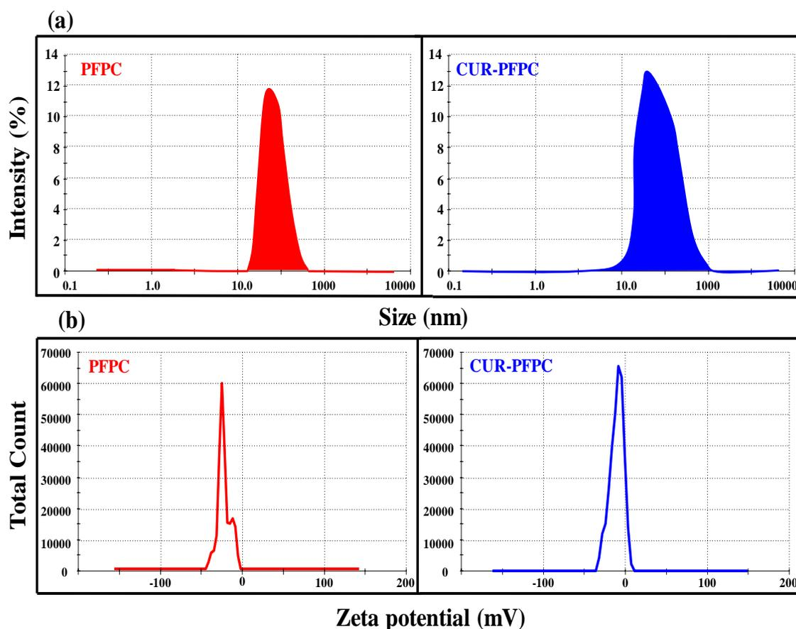
**Figure 4.4:** (a) Micellar size distribution, and (b) Zeta potential plots of optimized PFPC and CUR-PFPC formulations at  $30^{\circ}\pm 0.5^{\circ}$  C. Data are demonstrated as mean  $\pm$  S.D (n=3).
