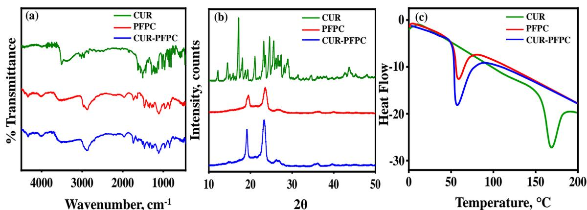
**Figure 4.6:** (a) FTIR spectrums, (b) XRD pattern, and (c) DSC thermograms of pure CUR, PFPC and CUR-PFPC formulations
