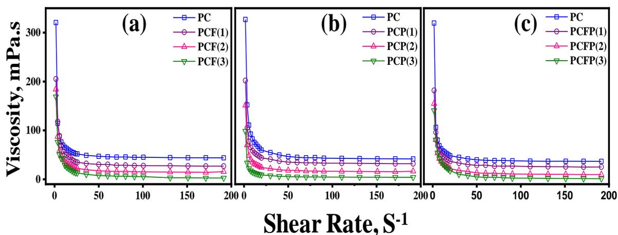
**Figure 5.3:** Variation of the shear viscosity as a function of shear rate for mixed (a) PCF, (b) PCP, and (c) PCFP micellar solutions (at  $30 \pm 0.5^\circ\text{C}$ ).
