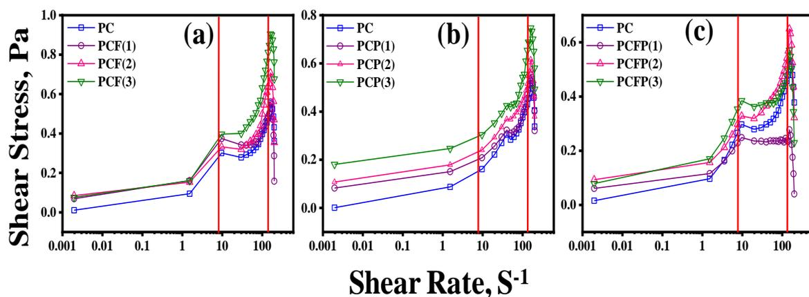
**Figure 5.5:** Variation of the shear stress ( $\tau$ ) as a function of shear rate ( $\gamma$ ) for mixed (a) PCF, (b) PCP, and (c) PCFP micellar solutions (at  $30\pm 0.5^{\circ}\text{C}$ ). [Fitting parameter was done using the selected range of data shown in-between the red-vertical lines].
