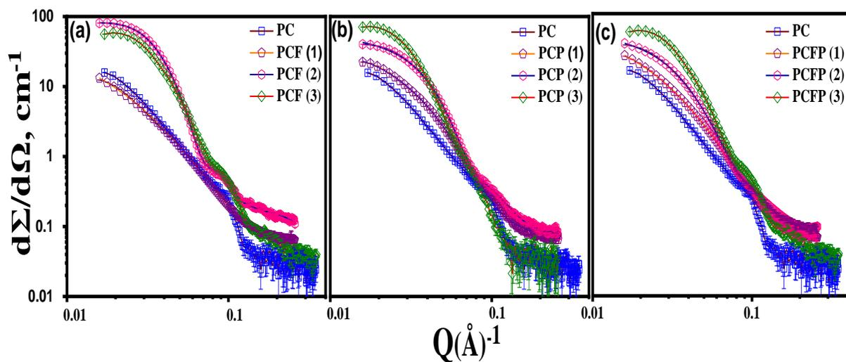
**Figure 5.2:** Experimental SANS pattern for mixed (a) PCFs (b) PCPs, and (c) PCFPs micellar solutions in D<sub>2</sub>O (at 30±0.5°C).
