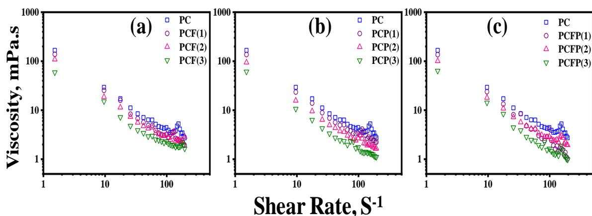
**Figure 5.4:** Variation of the shear viscosity as a function of shear rate for (a) PC and PCF (b) PCP and (c) PCFP micellar solutions at  $30^{\circ}\pm 0.5^{\circ}\text{C}$  for estimate the zero shear viscosity ( $\eta_0$ ) of the mixtures by extrapolating the viscosity data.
