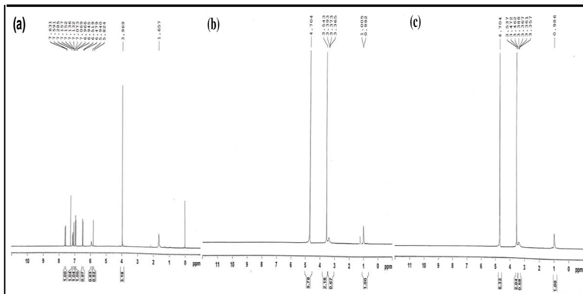
**Figure 5.8:** <sup>1</sup>H NMR spectra of (a) CUR in CDCl<sub>3</sub>, (b) blank mixed PCFP micellar system in D<sub>2</sub>O and (c) CUR-loaded mixed PCFP micellar system in D<sub>2</sub>O.
