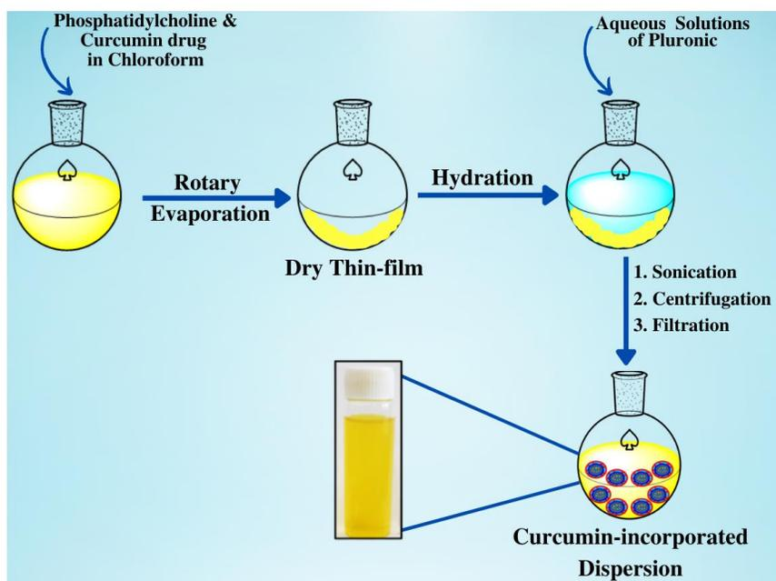
**Scheme 5.1:** Presentation of loading of CUR in the mixed micellar systems through thin film method.
