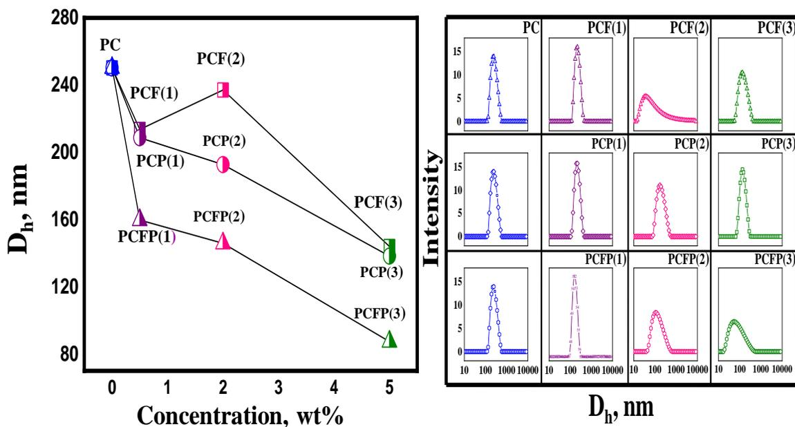
**Figure 5.1:** (a) Graph of  $D_h$  vs. concentration of PCF, PCP, and PCFP mixed micellar solutions (b) DLS stacks graph of PCF, PCP, and PCFP mixed micellar solutions (at  $30 \pm 0.5^\circ\text{C}$ ).
