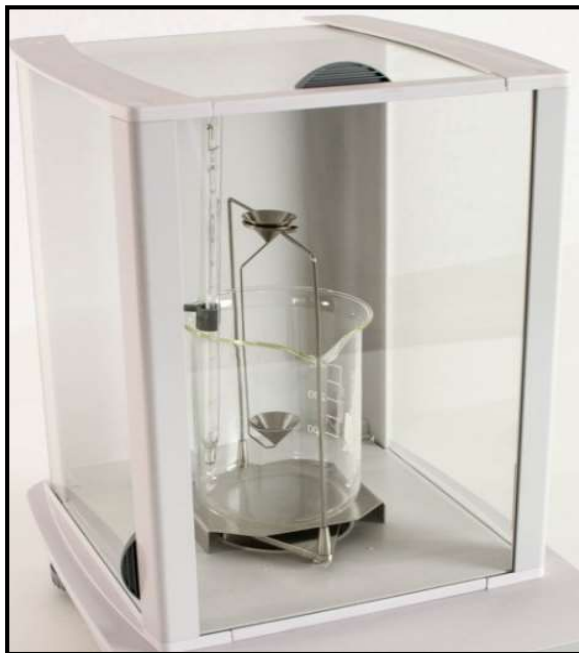
Figure 3.3: Density of Glass sample using Archimedes Principle.
