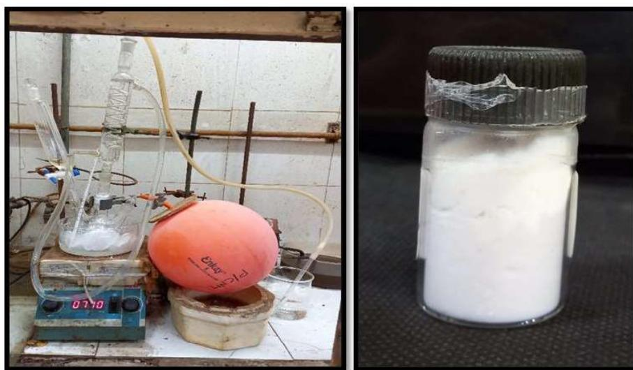
Fig 5.2 (A) Experimental Setup (B) Brominated Fumed Silica.
