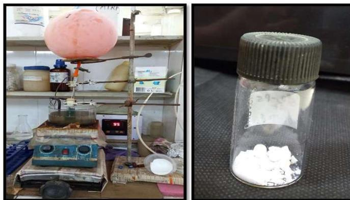
**Fig 5.3.** (A) Experimental Setup of ATRP Synthesis (B) Product ( $\text{SiO}_2\text{-g-PMMA}$ ).
