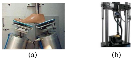
Figure 2.10: Prosthetic test frame (a) Fixed angle test frame (b) Test frame with a roller mechanism
