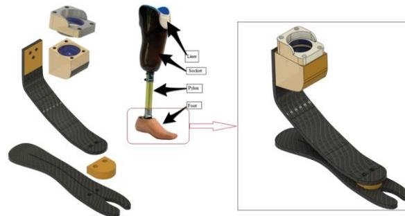
Figure 5.14: Prosthetic foot model 4
