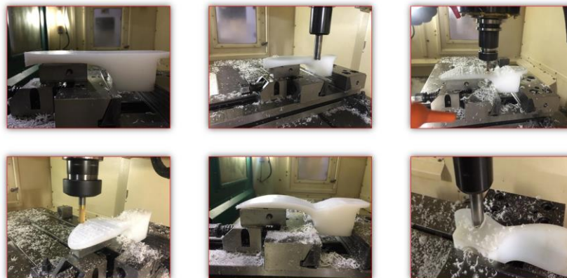
Figure 6.9: Machining process of prosthetic foot model
