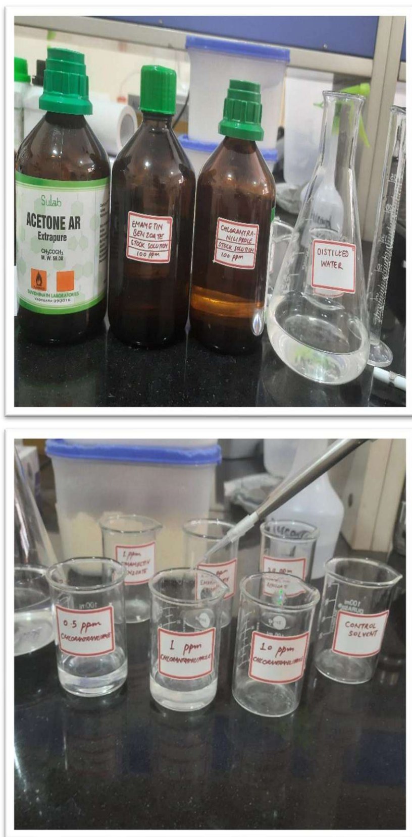
Figure 3.11: Stock solutions and preparing different concentrations of insecticide solutions.
