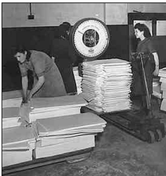
Figure 2.5 Sheet made of wood pulp (The Manufacturing Process for Viscose Rayon; Viscose Rayon Fibre Manufacturing Process: Summary)
