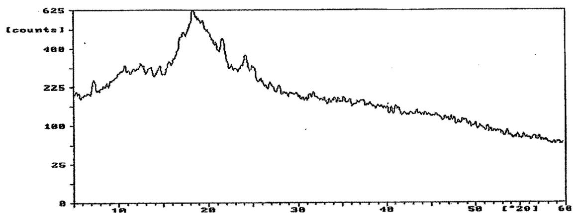
Figure 4.3.2.5.14. X-Ray diffraction pattern of HP-β-CD - Tadalafil Inclusion complex (3:1).
