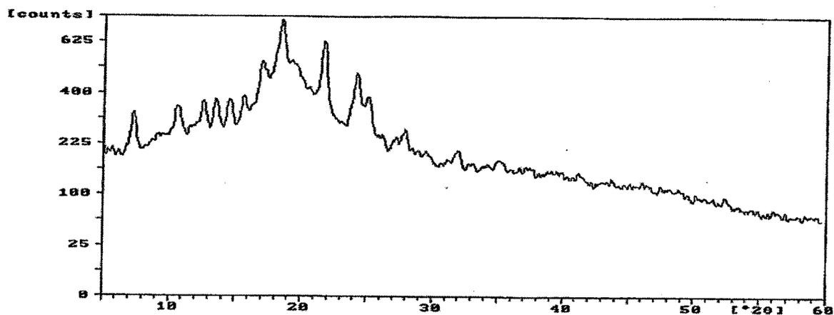
Figure 4.3.2.5.12. X-Ray diffraction pattern of HP-β-CD - Tadalafil physical mixture (3:1).
