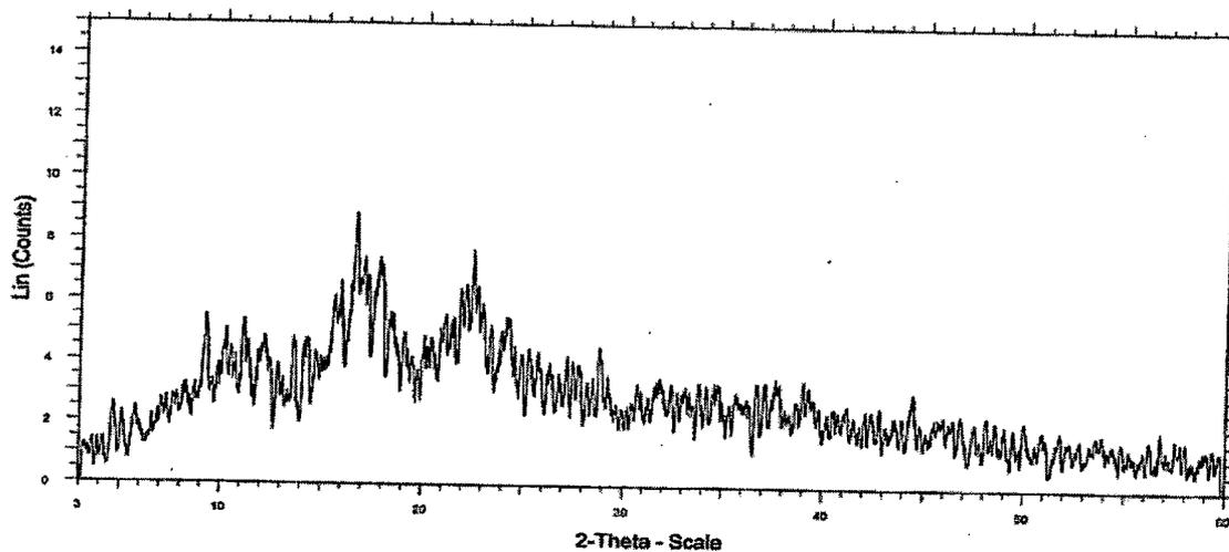
Figure 4.3.2.5.11. X-Ray diffraction pattern of  $\gamma$ -CD - Tadalafil Inclusion complex(3:1).
