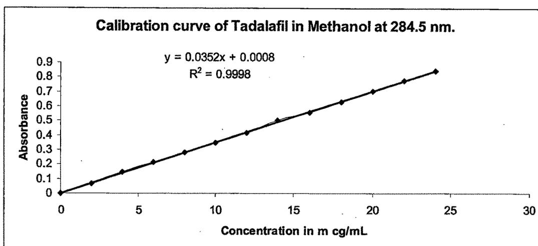
Figure 4.1.1.1. Calibration curve of Tadalafil in methanol at 284.5 nm
