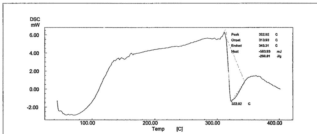
Figure 4.3.2.4.10. DSC thermogram of  $\gamma$ -CD-Tadalafil Inclusion complex by coprecipitation method (3:1)
