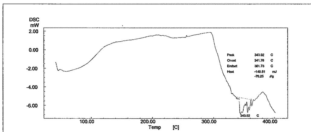
Figure 4.3.2.4.17. DSC thermogram of DM- $\beta$ -CD-Tadalafil Inclusion complex by kneading method (3:1)
