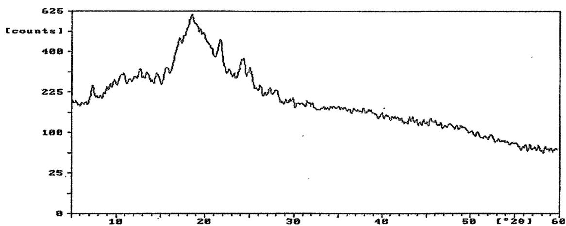
Figure 4.3.2.5.13. X-Ray diffraction pattern of HP-β-CD - Tadalafil Inclusion complex (2:1).
