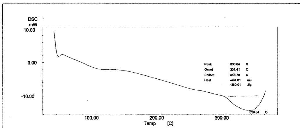
Figure 4.3.2.4.12. DSC thermogram of HP-β-CD-Tadalafil Physical mixture (3:1).
