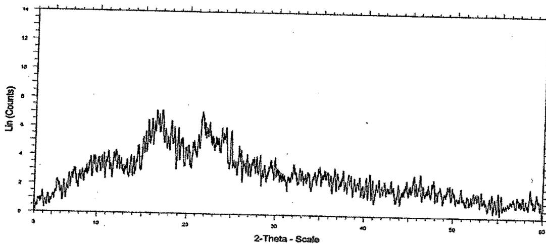
Figure 4.3.2.5.9. X-Ray diffraction pattern of  $\gamma$ -CD - Tadalafil physical mixture (3:1).
