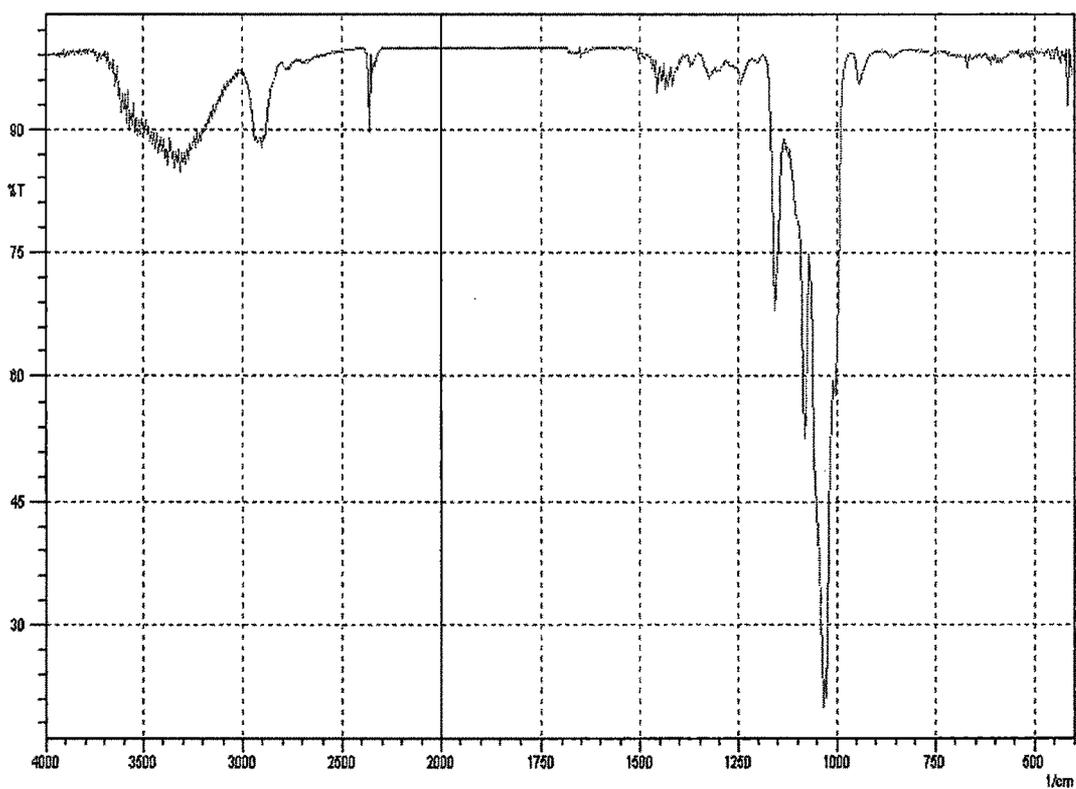
Figure 4.3.2.3.9. IR Spectrum of  $\gamma$ -CD-Tadalafil inclusion complex(3:1).
