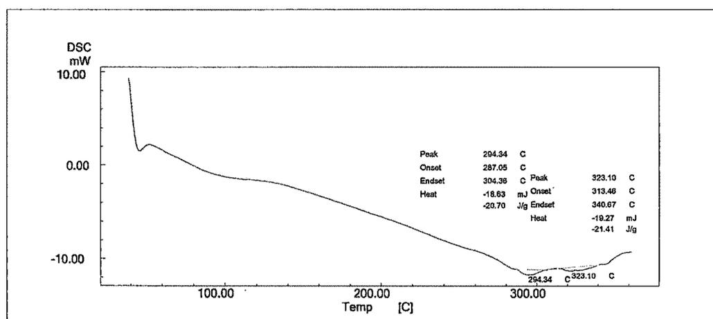
Figure 4.3.2.4.13. DSC thermogram of HP-β-CD-Tadalafil Inclusion complex by coprecipitation method (3:1)
