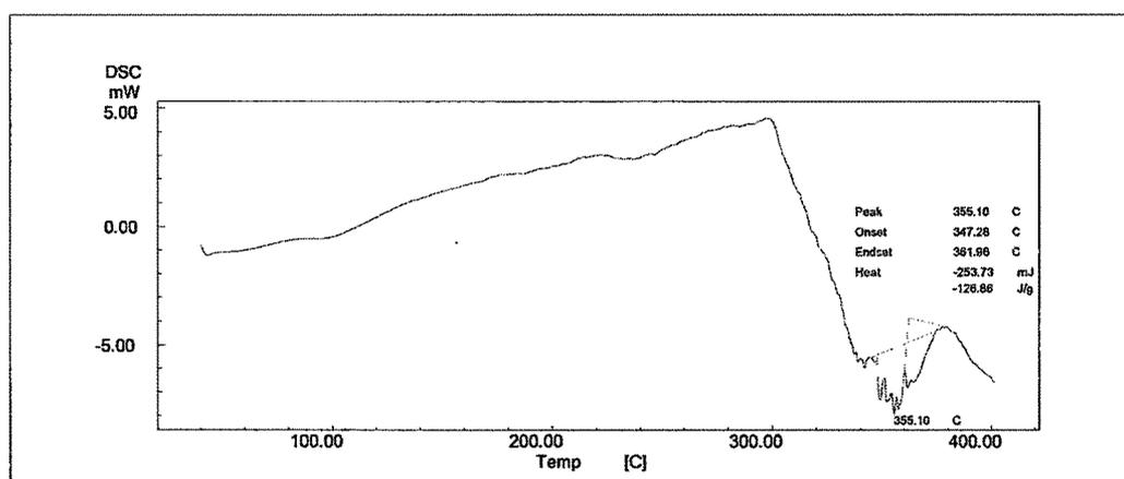
Figure 4.3.2.4.16. DSC thermogram of DM- $\beta$ -CD-Tadalafil Inclusion complex by coprecipitation method (3:1)
