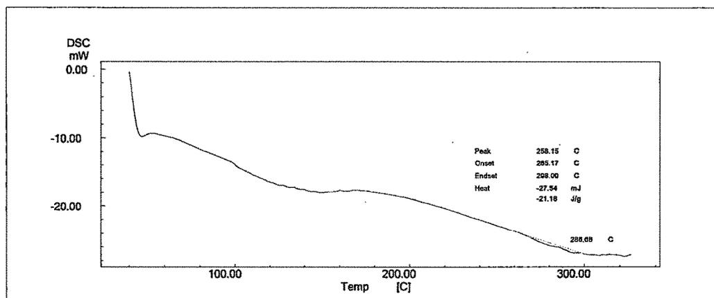
Figure 4.3.2.4.8. DSC thermogram of  $\beta$ -CD-Tadalafil Inclusion complex by kneading method (3:1)
