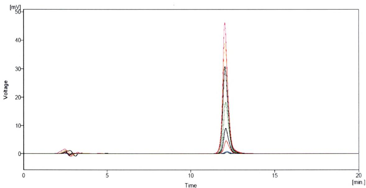
**Fig. 4.1.2.1 The overlain chromatograms of standard Tadalafil from 0.5 to 50.0μg/ml concentration in mobile phase**
