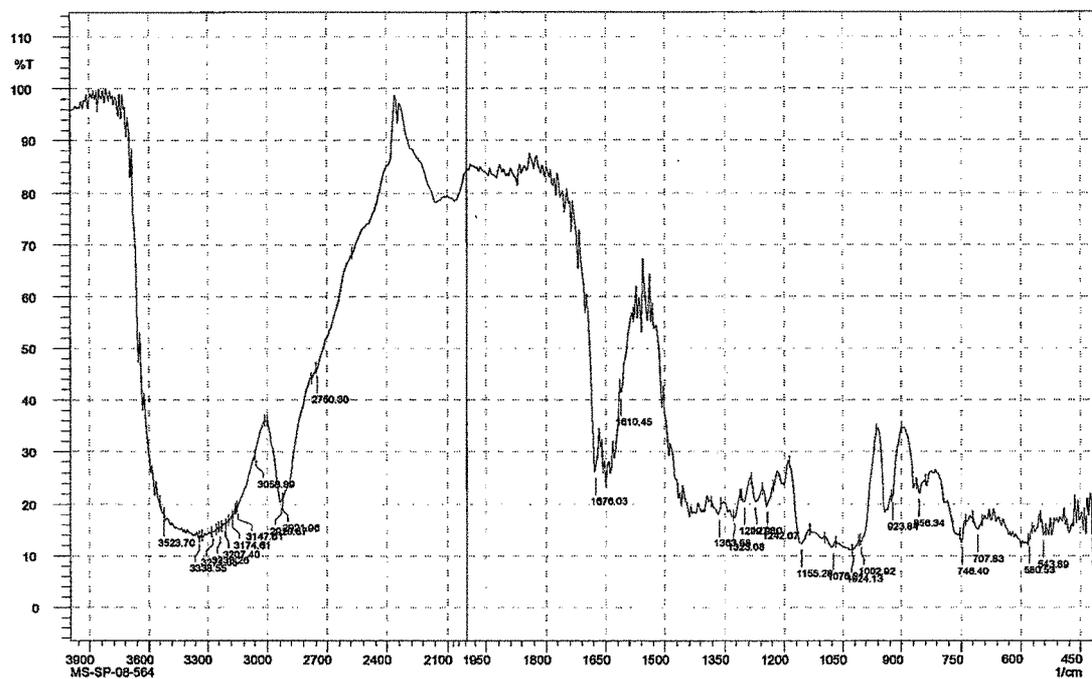
Figure 4.3.2.3.8. IR Spectrum of  $\gamma$ -CD-Tadalafil physical mixture(3:1).
