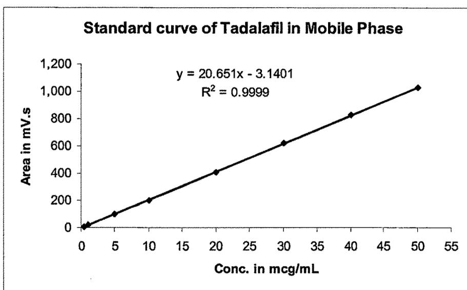
Fig. 4.1.2.2 Calibration curve for Tadalafil in mobile phase
