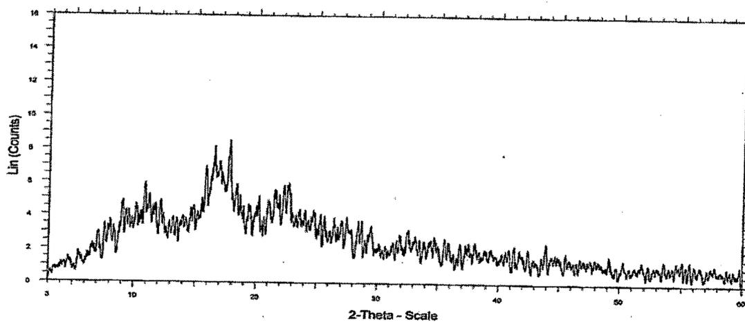
Figure 4.3.2.5.10. X-Ray diffraction pattern of  $\gamma$ -CD - Tadalafil Inclusion complex(2:1).
