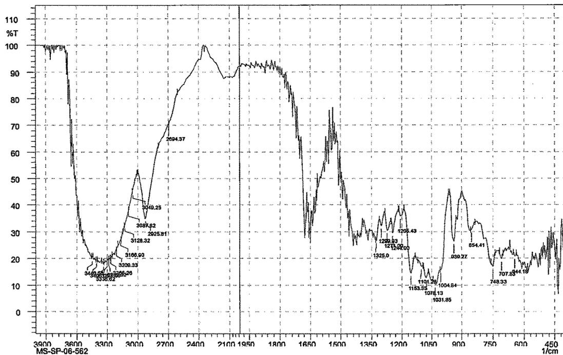
Figure 4.3.2.3.6. IR Spectrum of  $\beta$ -CD-Tadalafil physical mixture(3:1).
