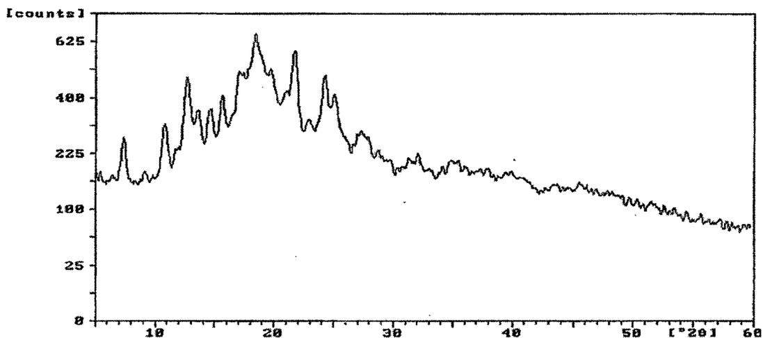
Figure 4.3.2.5.6. X-Ray diffraction pattern of  $\beta$ -CD - Tadalafil physical mixture (3:1).
