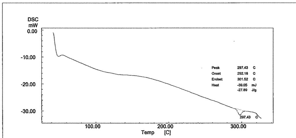
Figure 4.3.2.4.6. DSC thermogram of  $\beta$ -CD-Tadalafil Physical mixture (3:1).
