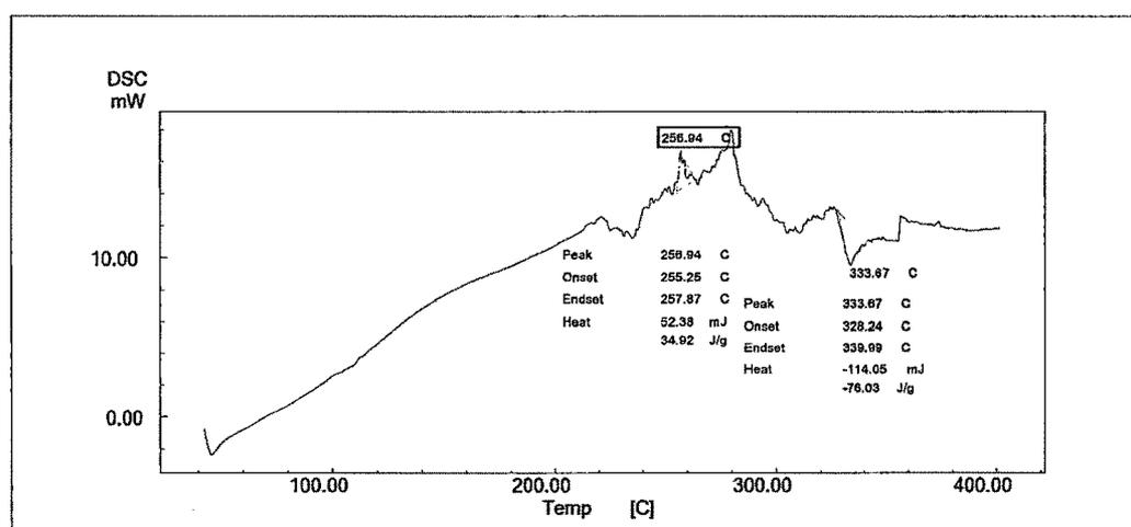
Figure 4.3.2.4.11. DSC thermogram of  $\gamma$ -CD-Tadalafil Inclusion complex by kneading method (3:1)
