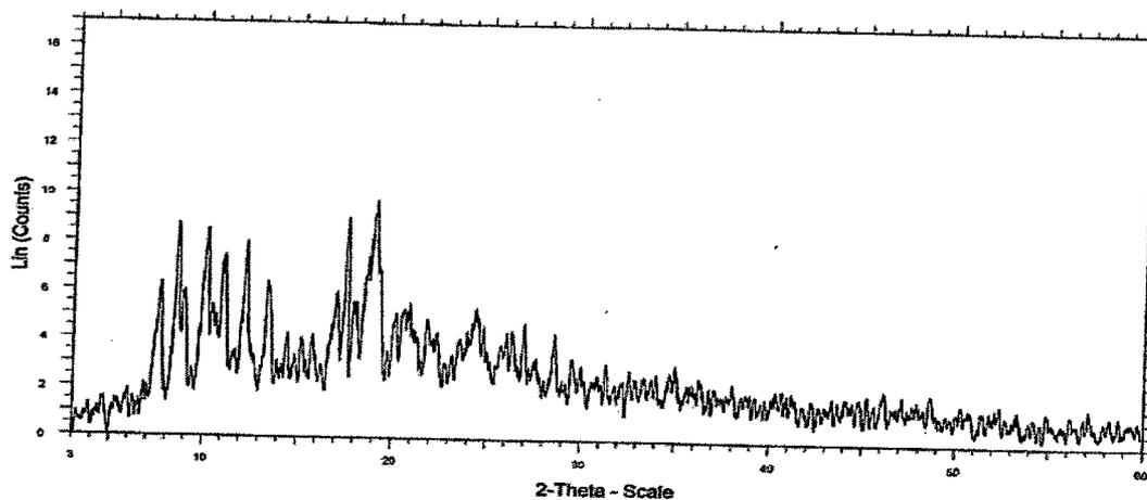
**Figure 4.3.2.5.17. X-Ray diffraction pattern of DM- $\beta$ -CD - Tadalafil Inclusion complex (3:1).**
