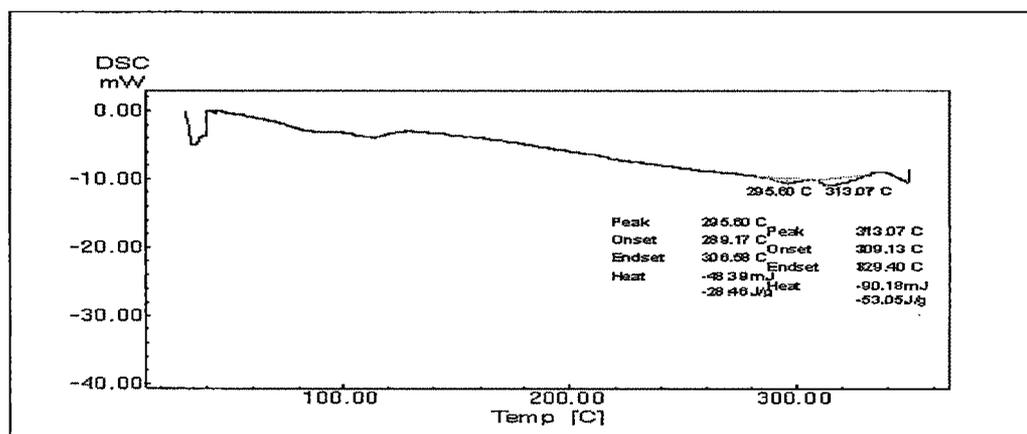
Figure 4.3.2.4.7. DSC thermogram of  $\beta$ -CD-Tadalafil Inclusion complex by coprecipitation method (3:1)
