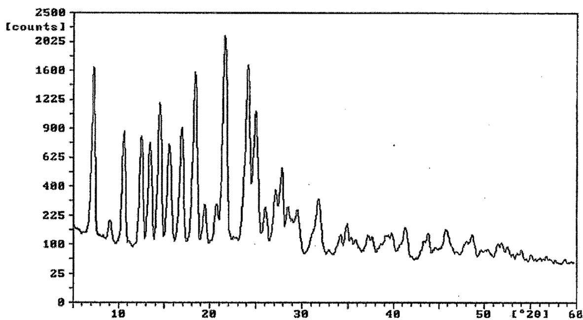
Figure 4.3.2.5.5. X-Ray diffraction pattern of Tadalafil.
