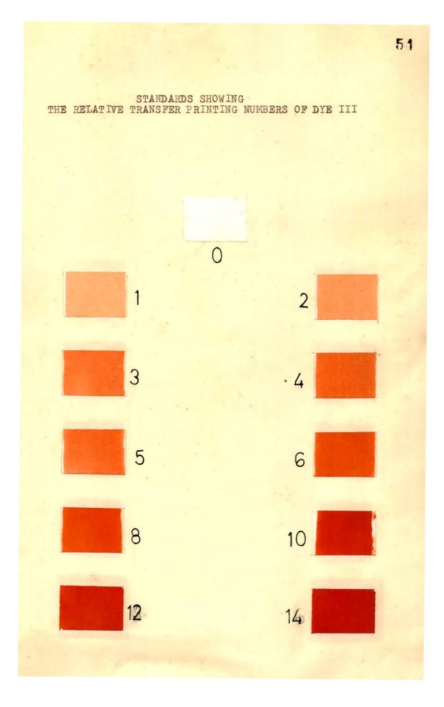
In dye I the relative transfer printing numbers given to the standards prepared were according to the concentration of the dye solution used i.e. No. 2 was given to the standards prepared by using 2% dye solution and so on.
