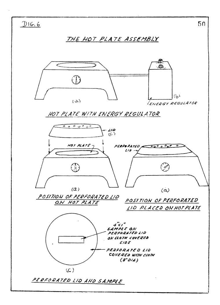
When the temperature reached to 200<sup>b</sup><sub>1</sub>C on the hot plate and maintained by the energy regulator, the perforated lid along with the sample was inverted onto the hot plate and a weight of two kg was placed on the lid and kept for 2 minutes for transfer printing. The lid was lifted and the sample was removed from the lid.
