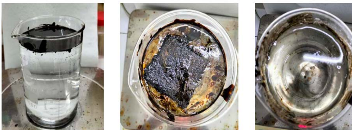
Plate 4.14: Oil sorption testing in oil-layer system of Non-woven in HvCo
