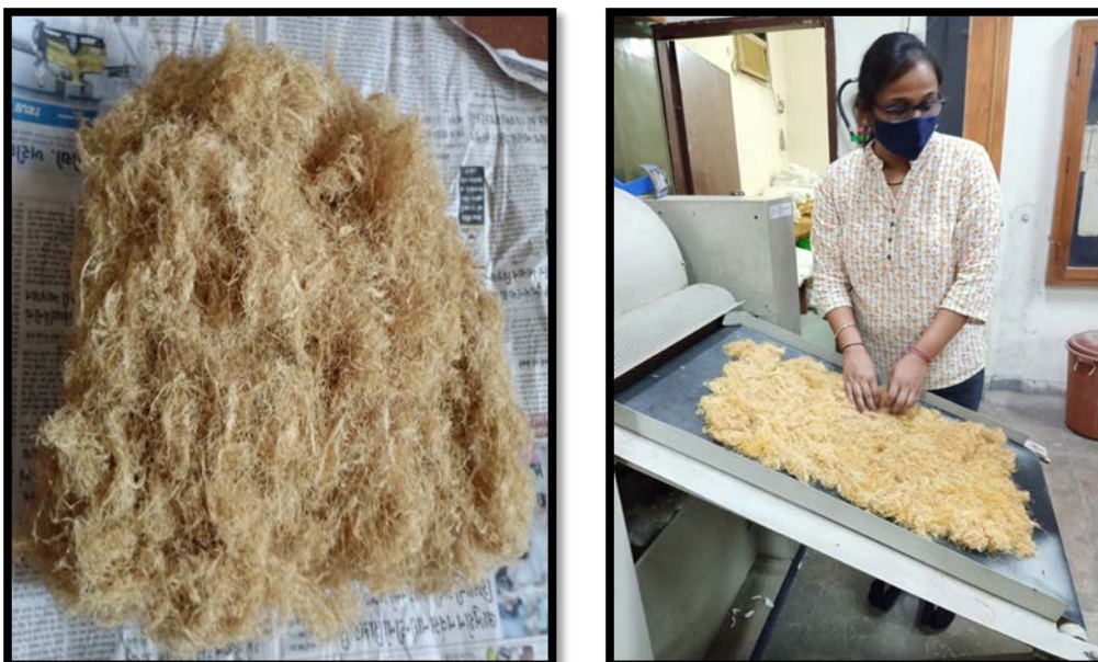
Plate 4.8: Laying of hand-opened carded fibres and web formation
