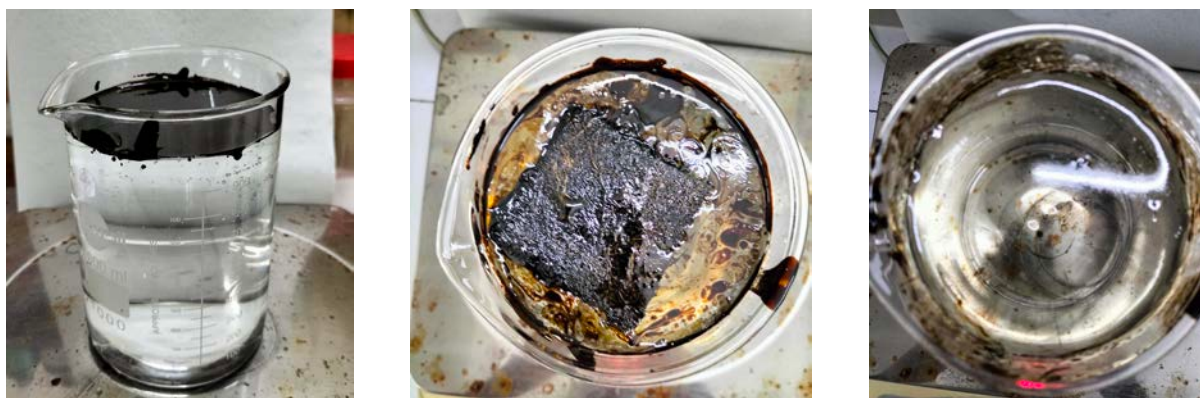
Fig.4.16. Oil sorption testing of Nonwoven in Heavy viscosity crude oil
