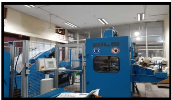
Fig.4.13. Manufacturing of Non-woven through DILO-Needle Punching machine
