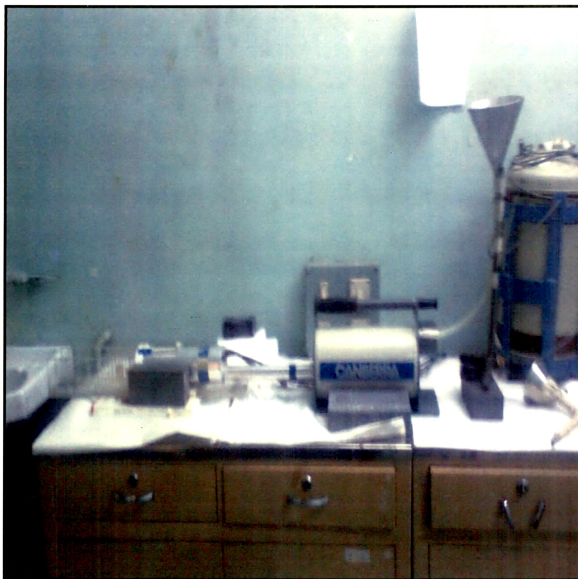
Fig. 4.4 High Purity Germanium (HPGe) Detector at RCD lab, TIFR, Mumbai
