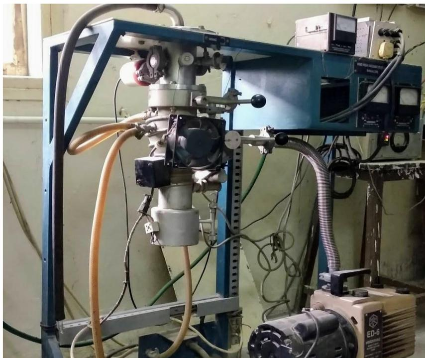
*Figure 2.1:* Vacuum sealing unit for evacuating the ampoules at pressure  $> 10^{-5}$  Torr.
