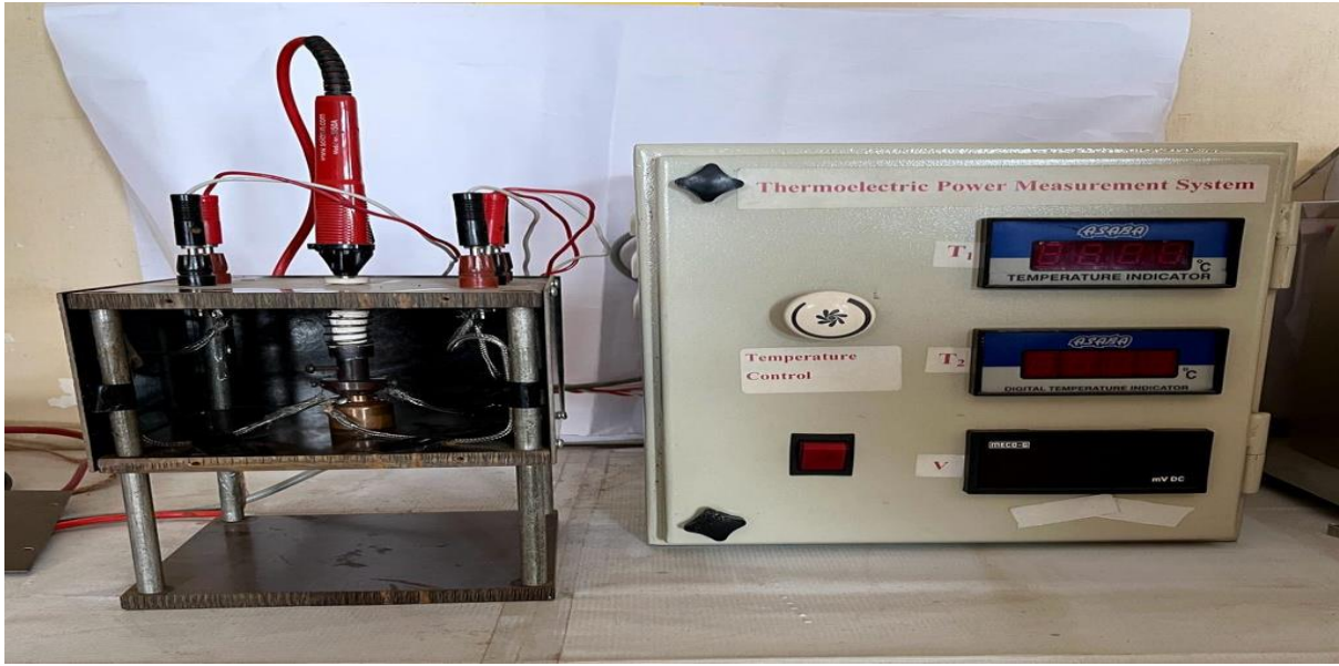
Figure 2.10: Thermoelectric power measurement set up
