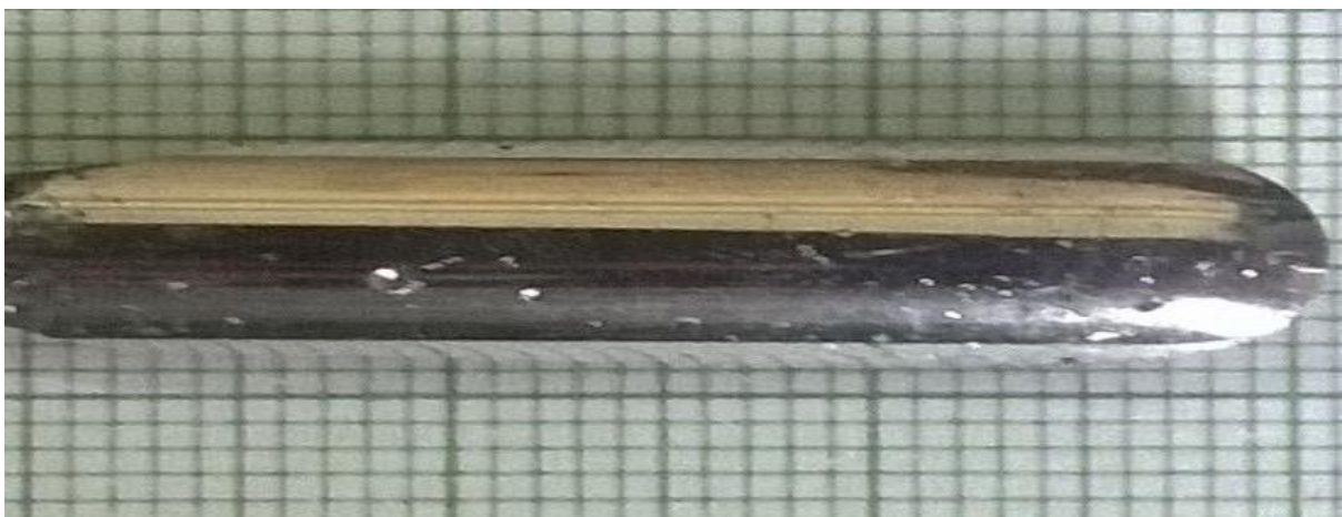
Figure 3.3: As grown crystal of \text{InBi}_{0.90}\text{Te}_{0.10}
