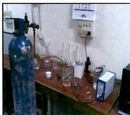
**Fig 3.15 Experimental Setup for EPR test. Fig 3.16 Argon purging**
