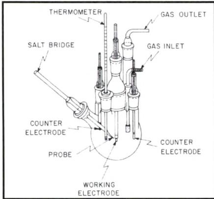
Fig. 3.11 Corrosion cell
