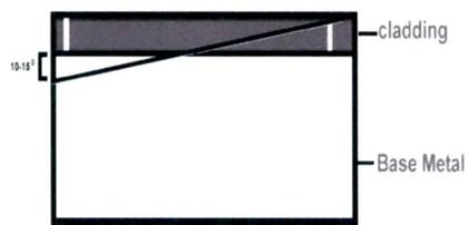
Fig. 3.5 Taper grinding of cladded samples
