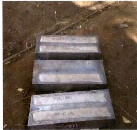
**Fig 3.4 weld overlay developed by ESSC Process**
