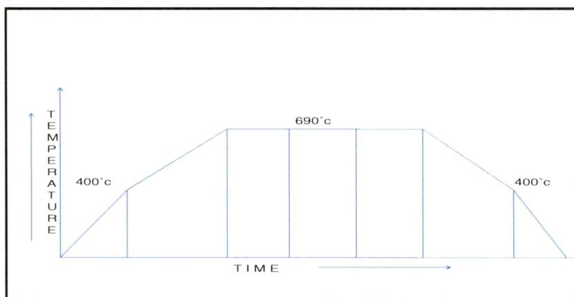
Fig 3.8 PWHT cycle for both weld overlays
