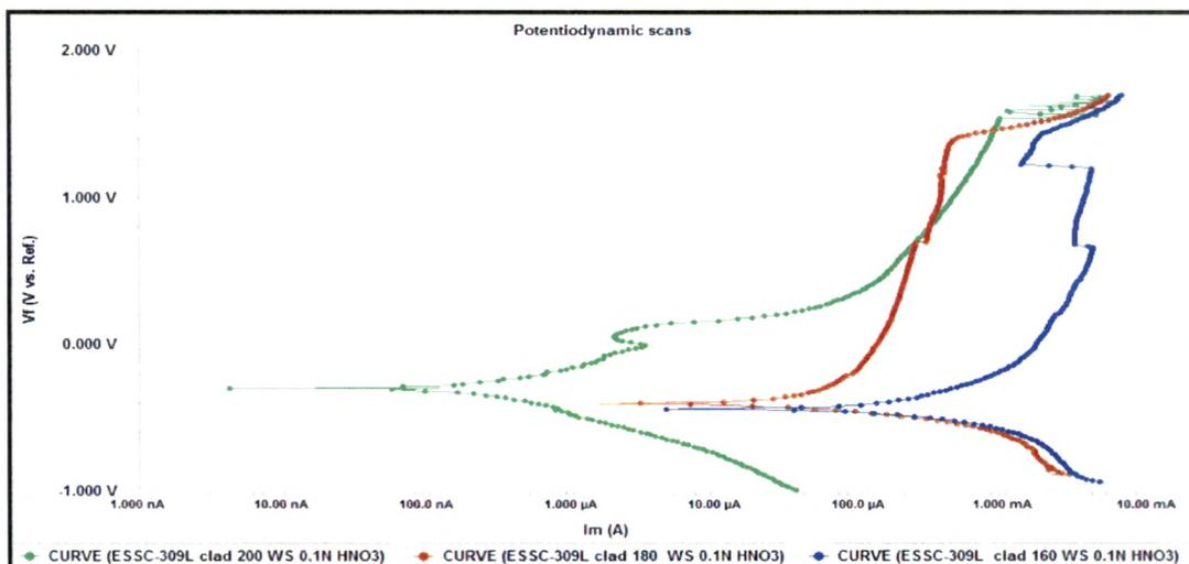
Fig. 4.59 : Potentiodynamic scans of 309L clad weld overlays at different welding speed in 0.1N HNO<sub>3</sub> solution
