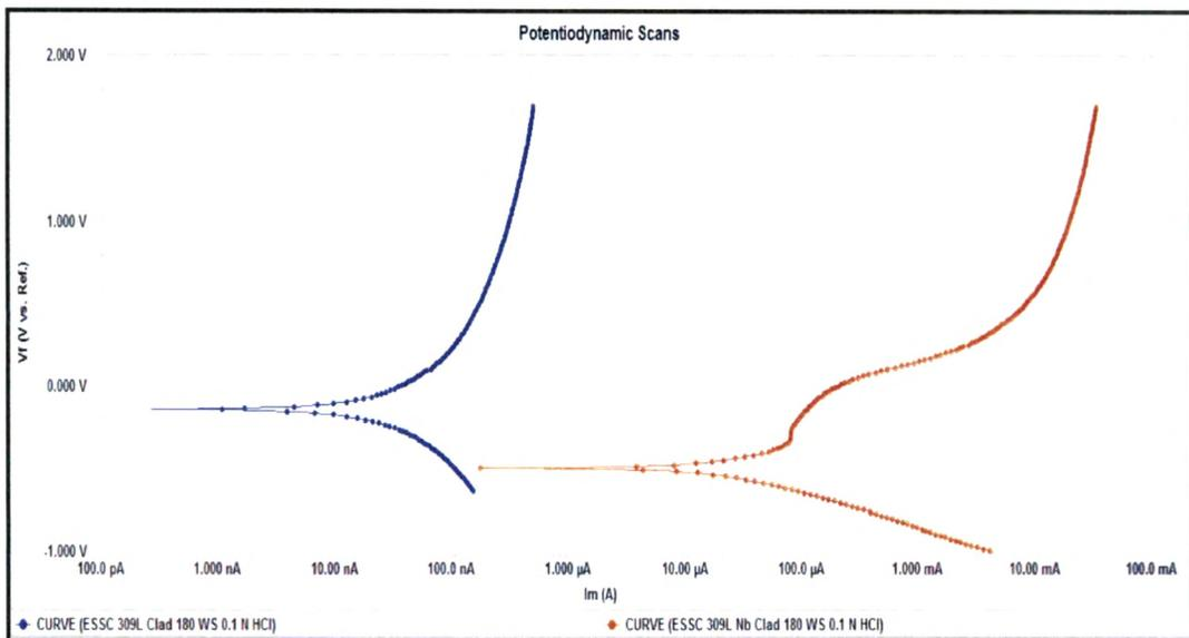
**Fig. 4.106 : Potentiodynamic scans of cladded region of 309 L & 309 L Nb cladded weld overlay develop with 180 mm / min. welding speed in 0.1 N HCl solution**
