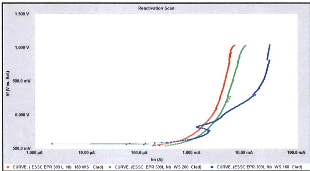
Fig. 4.85 EPR scans of 309LNb cladded weld overlays at different welding speed in 0.1 H<sub>2</sub>SO<sub>4</sub> + 0.01 M NaCl Solution
