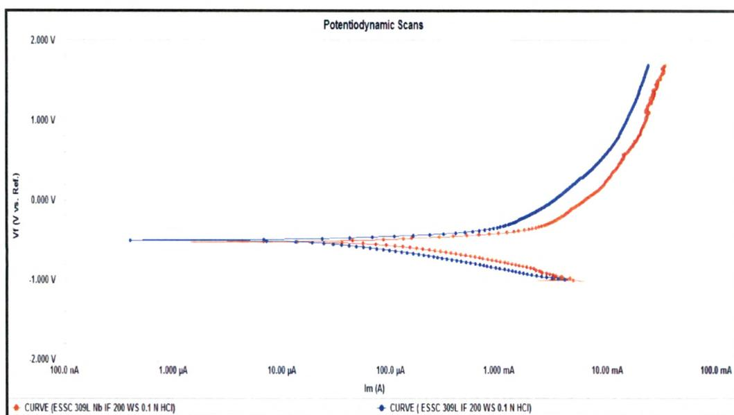
Fig.4.110 Potentiodynamic scans of Interface region of 309 L & 309 L Nb cladded weld overlay develop with 200 mm / min. welding speed in 0.1 N HCl solution
