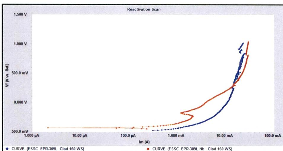
Fig. 4.129 : EPR scans of cladded region of 309 L & 309 L Nb cladded weld overlays developed with 160 mm / min. welding speed in 0.1 H<sub>2</sub>SO<sub>4</sub> + 0.01 M NaCl Solution
