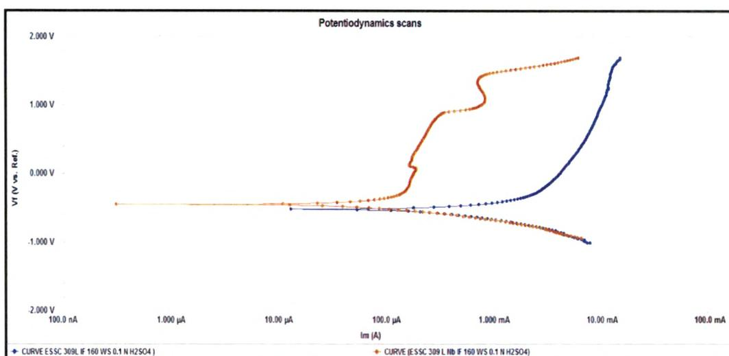
Fig. 4.102 : Potentiodynamic scans of Interface region of 309 L & 309 L Nb cladded weld overlay develop with 160 mm / min. welding speed in 0.1 N H<sub>2</sub>SO<sub>4</sub> solution
