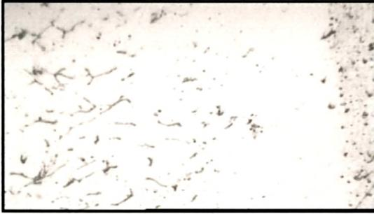
**Fig.4.152 (a) Cladded region of 309 L Nb Clad at 200 WS as welded condition**
