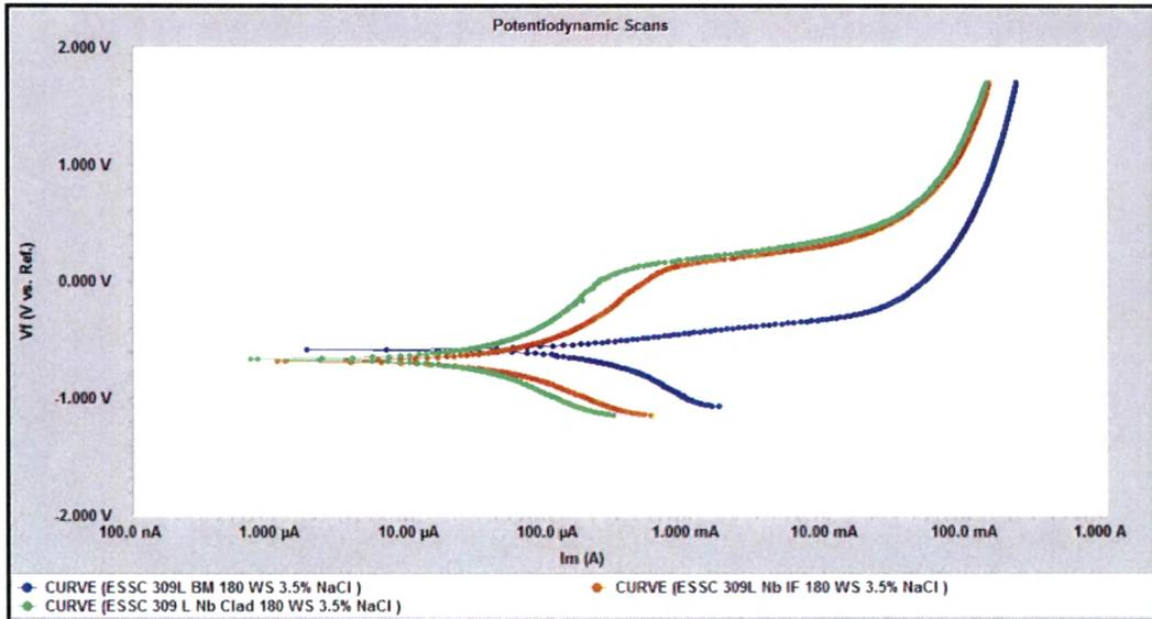
**Fig. 4.23: Potentiodynamic scans of 309 L Nb cladded weld overlay develop with 180mm / min. welding speed at different location in 3.5 % NaCl Solution**
