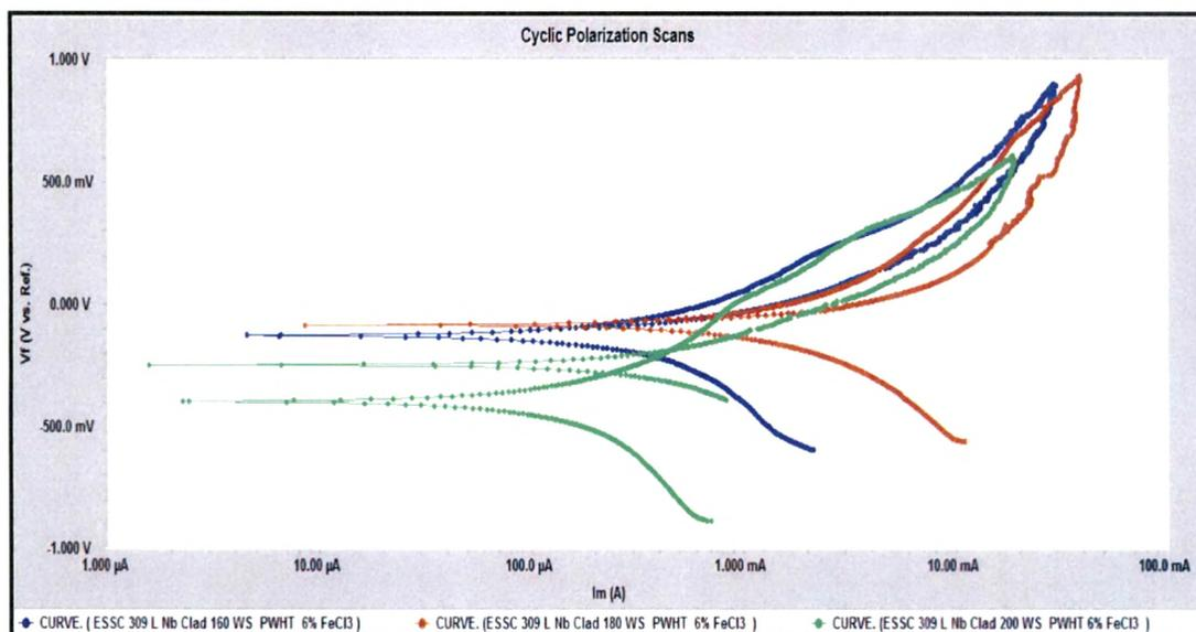
Fig. 4.155 : Cyclic polarization scans of clad region of 309L Nb Cladded weld overlays at different welding speed after PWHT in 6% FeCl<sub>3</sub> Solution
