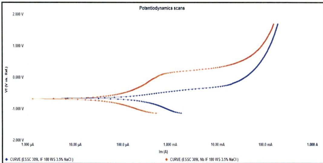
**Fig. 4.115 : Potentiodynamic scans of Interface region of 309 L & 309 L Nb cladded weld overlay develop with 180 mm / min. welding speed in 3.5 % NaCl solution**
