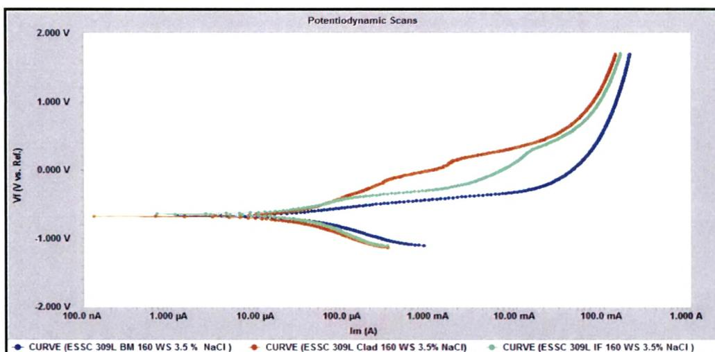
Fig. 4.19: Potentiodynamic scans of 309 L cladded weld overlay develop with 160mm / min. welding speed at different location in 3.5 % NaCl Solution
