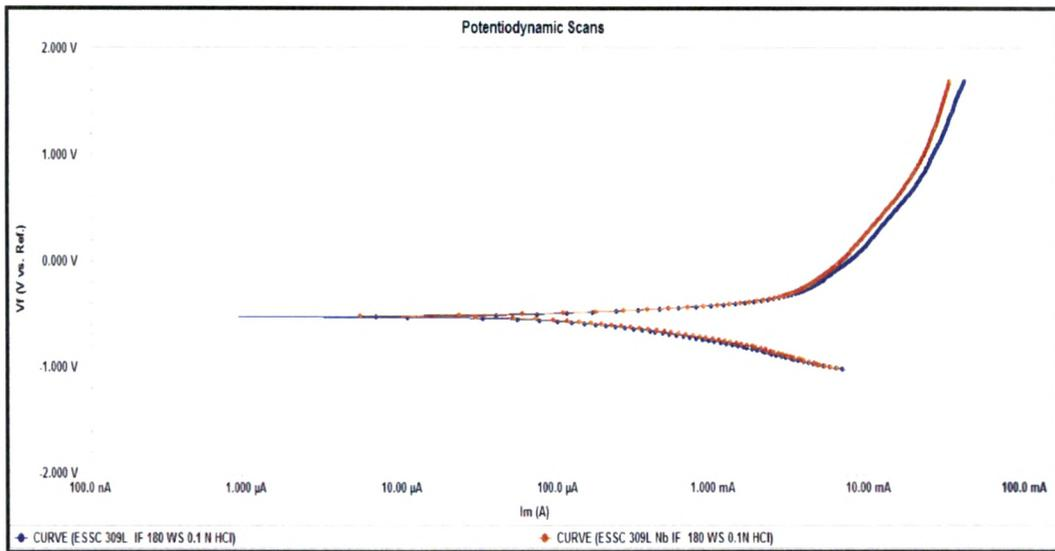
**Fig. 4.109 Potentiodynamic scans of Interface region of 309 L & 309 L Nb cladded weld overlay develop with 180 mm / min. welding speed in 0.1 N HCl solution**
