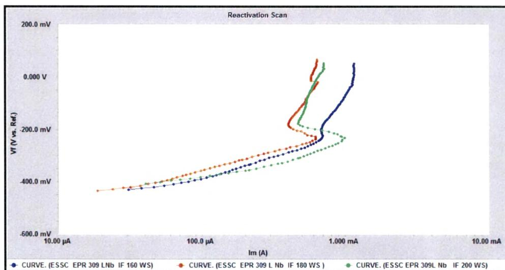
Fig. 4.86 EPR scans of interface of 309LNb cladded weld overlays at different welding speed in 0.1 H<sub>2</sub>SO<sub>4</sub> + 0.01 M NaCl Solution
