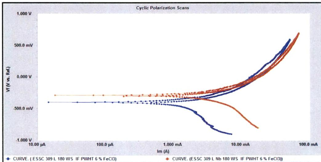
**Fig. 4.127 : Cyclic polarization scans of 309 L & 309 L Nb cladded weld overlay develop with 180 mm / min. welding speed at interface region after PWHT in 6 % FeCl<sub>3</sub> Solution**
