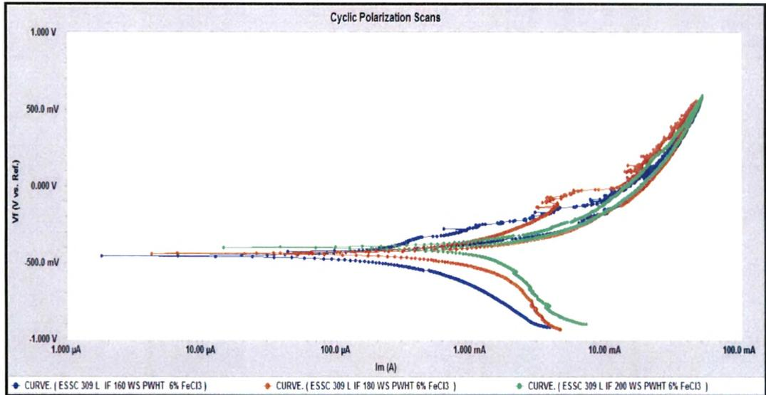
Fig. 4.156 : Cyclic polarization scans of interface region 309L cladded weld overlays at different welding speed after PWHT in 6% FeCl<sub>3</sub> Solution
