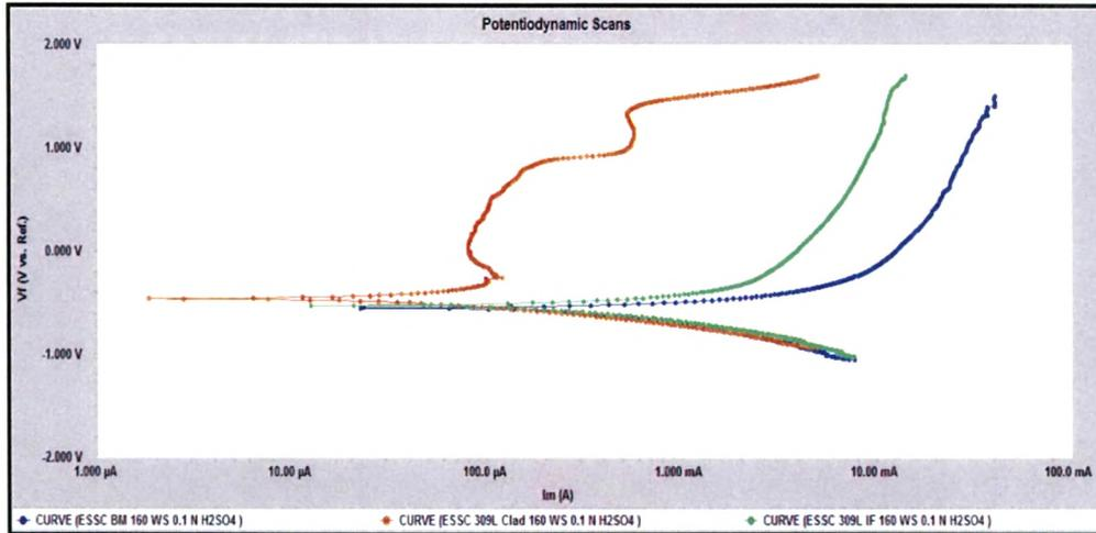
Fig. 4.13: Potentiodynamic scans of 309 L cladded weld overlay develop with 160mm / min. welding speed at different location in 0.1 N H<sub>2</sub>SO<sub>4</sub> Solution
