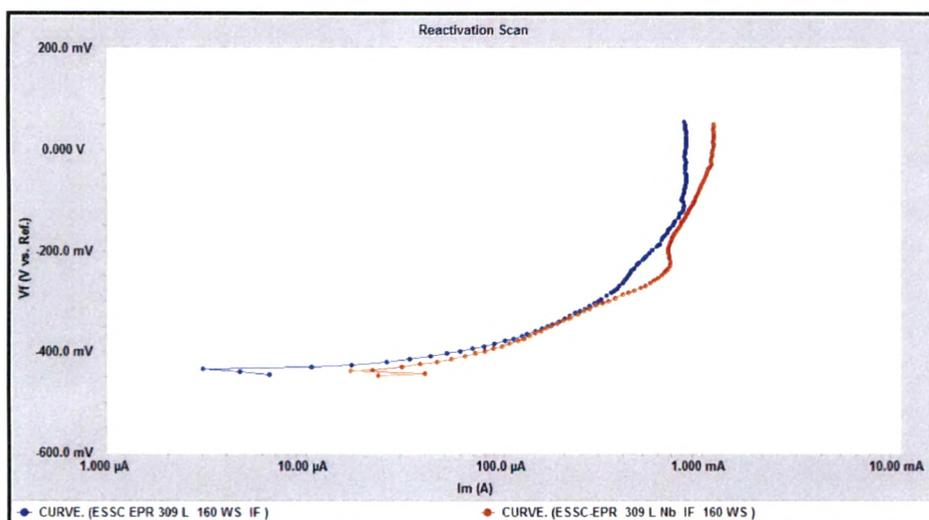
Fig. 4.132 : EPR scans of interface region of 309 L & 309 L Nb cladded weld overlays developed with 160 mm / min. welding speed in 0.1 H<sub>2</sub>SO<sub>4</sub> + 0.01 M NaCl Solution
