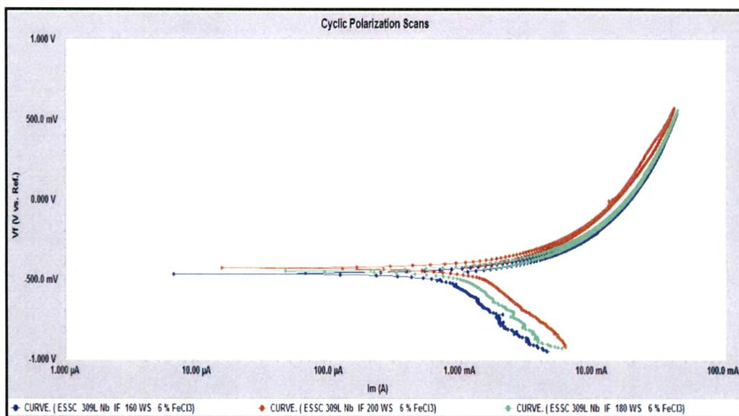
Fig. 4.157 : Cyclic polarization scans of interface region of 309LNb Cladded weld overlays at different welding speed in 6% FeCl<sub>3</sub> Solution
