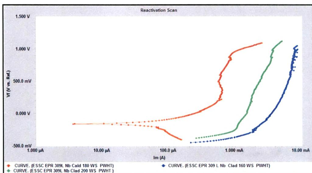
Fig. 4.159 : EPR scans of clad region of 309LNb cladded weld overlays at after PWHT at different welding speed in 0.1 H<sub>2</sub>SO<sub>4</sub> + 0.01 M NaCl Solution
