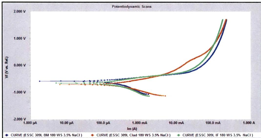
Fig.4. 20: Potentiodynamic scans of 309 L cladded weld overlay develop with 180mm / min. welding speed at different location in .5 % NaCl Solution
