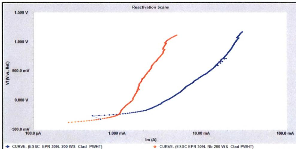
**Fig. 4.137 : EPR scans of cladded region of 309 L & 309 L Nb cladded weld overlay developed with 200 mm / min. welding speed in 0.1 H<sub>2</sub>SO<sub>4</sub> + 0.01 M NaCl Solution after PWHT**
