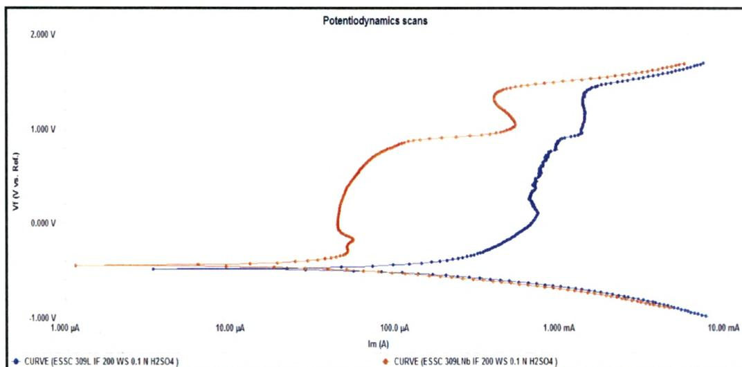
**Fig. 4.104 : Potentiodynamic scans of Interface region of 309 L & 309 L Nb cladded weld overlay develop with 200 mm / min. welding speed in 0.1 N H<sub>2</sub>SO<sub>4</sub> solution**
