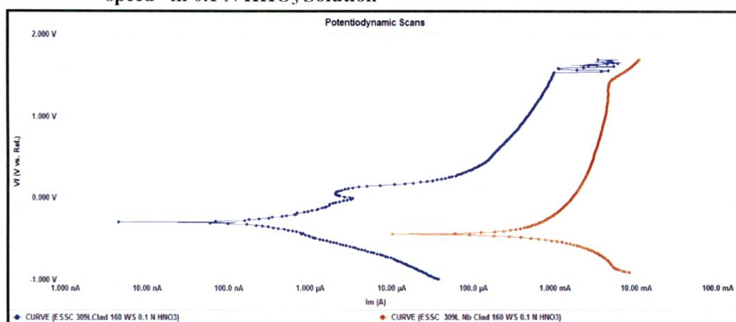
Fig.4.93 Potentiodynamic scans of clad region of 309 L & 309 L Nb clad weld overlay develop with 160 mm / min. welding speed in 0.1 N HHO<sub>3</sub> Solution
