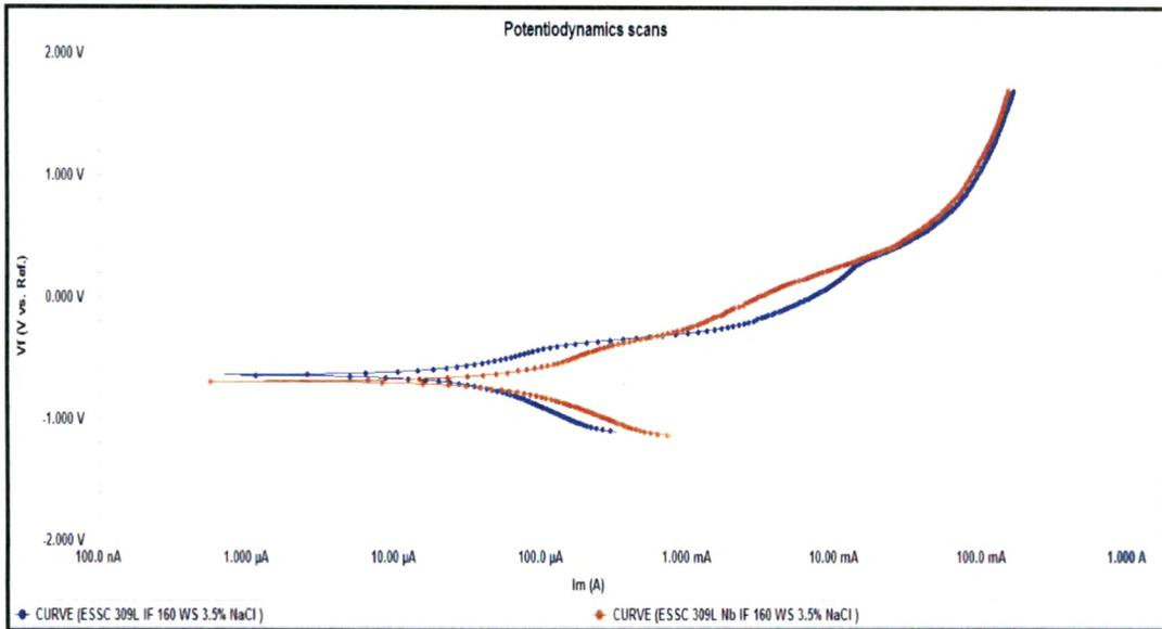
Fig. 4.114 : Potentiodynamic scans of Interface region of 309 L & 309 L Nb cladded weld overlay develop with 160 mm / min. welding speed in 3.5 % NaCl solution
