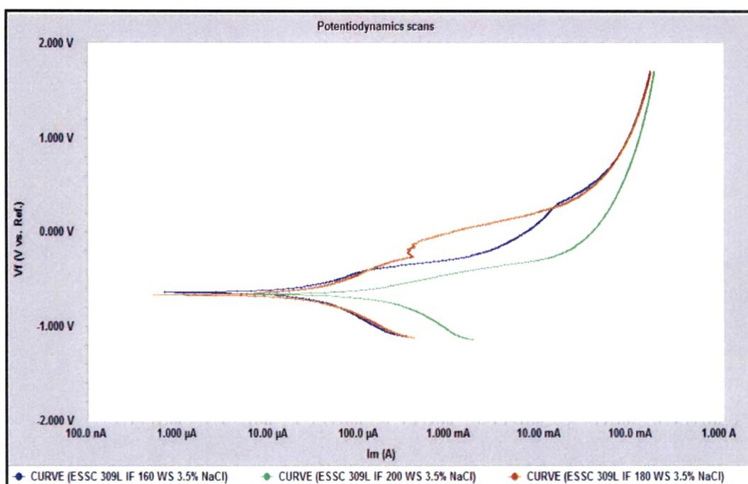
Fig. 4.75: Potentiodynamic scans of interface of 309L cladded weld overlays at different welding speed in 3.5 % NaCl solution
