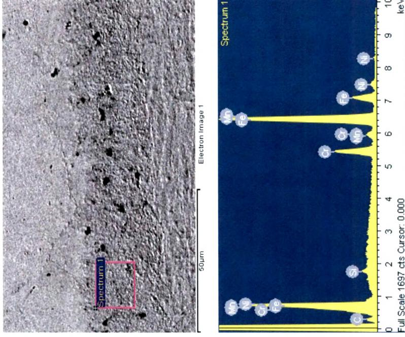
Fig. 4.49 EDAX analysis at interface of 309 L cladded weld overlay developed with 180 mm/ min welding speed
