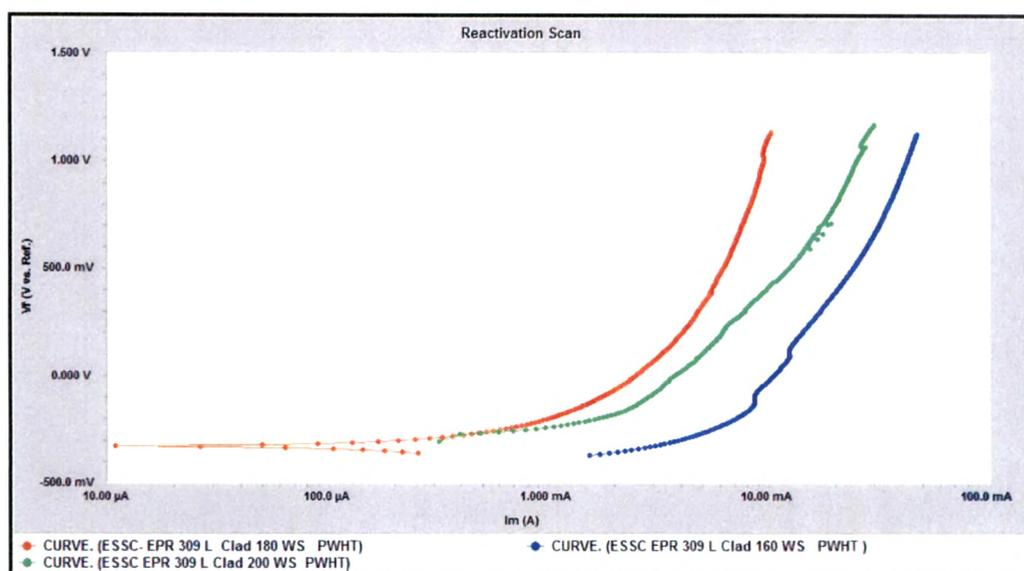
Fig. 4.158 : EPR scans of clad region of 309L cladded weld overlays after PWHT at different welding speed in 0.1 H<sub>2</sub>SO<sub>4</sub> + 0.01 M NaCl Solution
