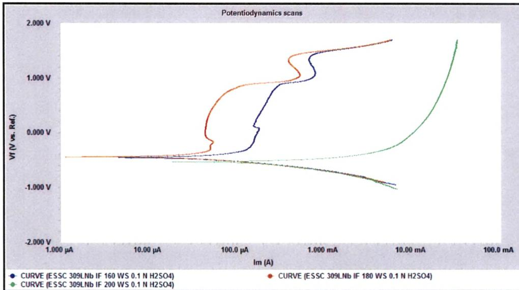
**Fig. 4.72: Potentiodynamic scans of interface of 309L Nb cladded weld overlays at different welding speed in 0.1N H<sub>2</sub>S0<sub>4</sub> solution**
