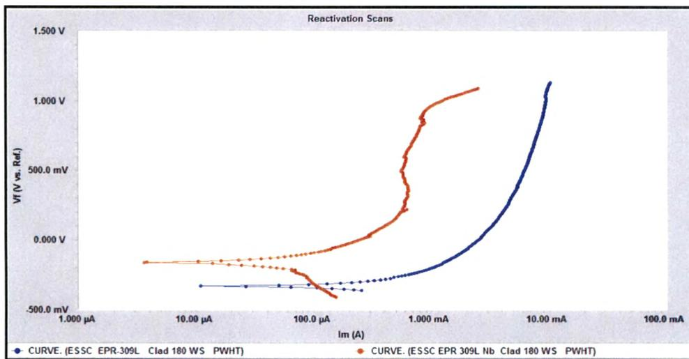
**Fig. 4.136 EPR scans of cladded region of 309 L & 309 L Nb cladded weld overlay developed with 180 mm / min. welding speed in 0.1 H<sub>2</sub>SO<sub>4</sub> + 0.01 M NaCl Solution after PWHT**
