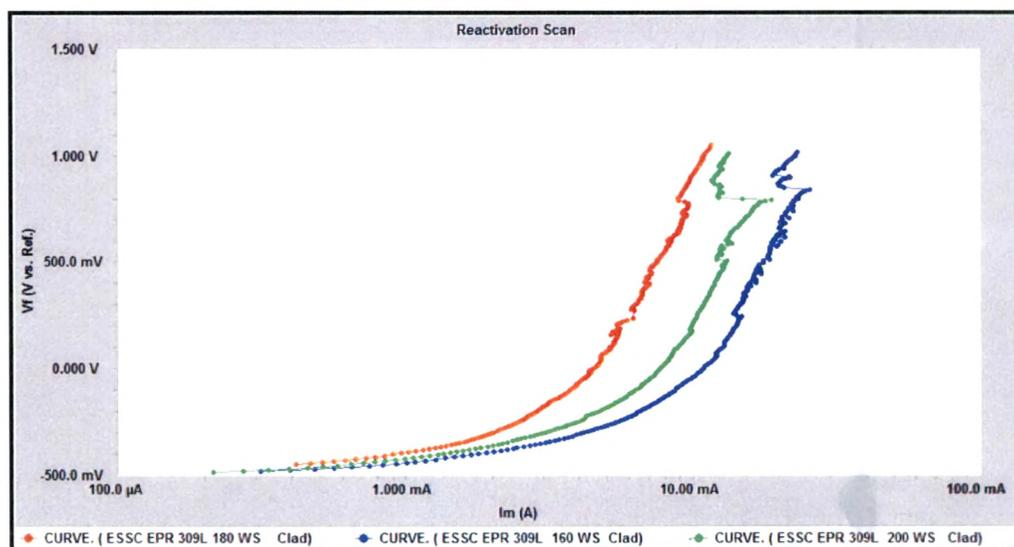
Fig. 4.83 EPR scans of 309L cladded weld overlays at different welding speed in 0.1 H<sub>2</sub>SO<sub>4</sub> + 0.01 M NaCl Solution
