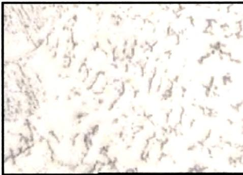
**Fig.4.29 (a) clad region of 309 L Clad 200 WS**
