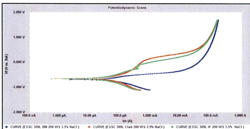
Fig.4.21: Potentiodynamic scans of 309 L cladded weld overlay develop with 200 mm / min. welding speed at different location in 3.5 % NaCl Solution
