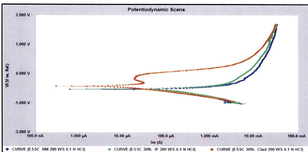
**Fig. 4.9 Potentiodynamic scans of 309 L cladded weld overlay develop with 200 mm / min. welding speed at different location in 0.1 N HCl Solution**
