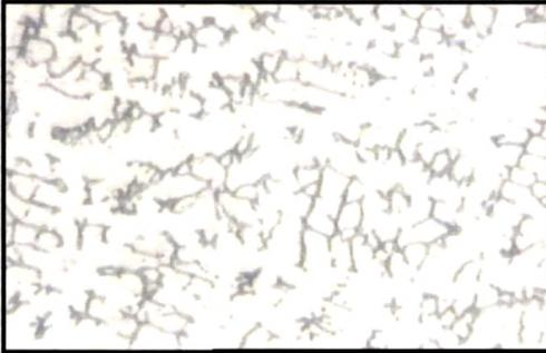
Fig. 4.88 (a) Cladded region of 309 L Clad 180 WS
