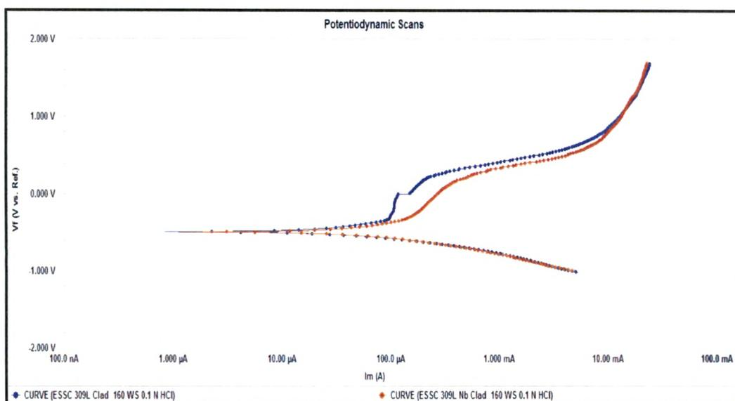
**Fig.4.105 : Potentiodynamic scans of cladded region of 309 L & 309 L Nb cladded weld overlay develop with 160 mm / min. welding speed in 0.1 N HCl solution**
