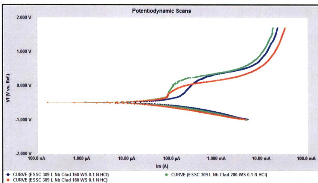
Fig. 4.66 Potentiodynamic scans of 309L Nb cladded weld overlays at different WS in 0.1N HCl Solution
