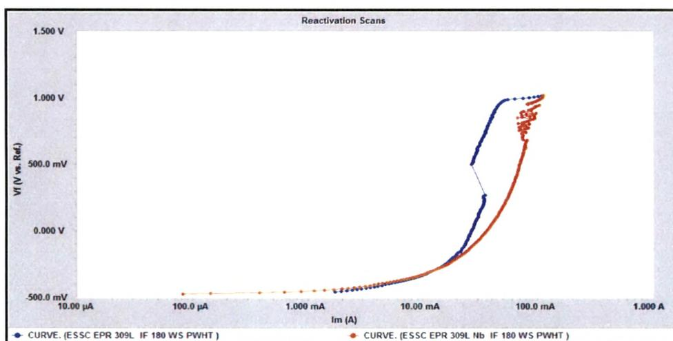
Fig. 4.139 : EPR scans of interface region of 309 L & 309 L Nb cladded weld overlay developed with 180 mm / min. welding speed in 0.1 H<sub>2</sub>SO<sub>4</sub> + 0.01 M NaCl Solution after PWHT
