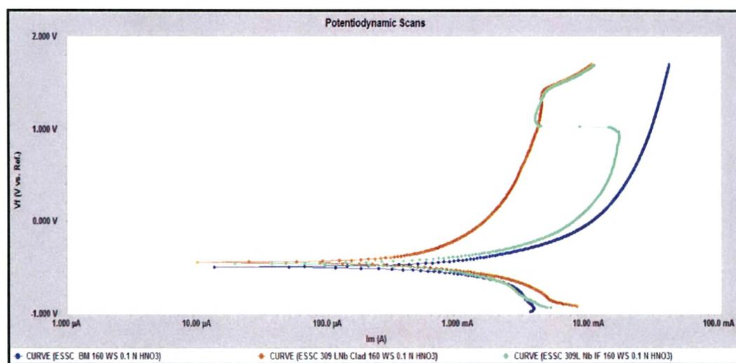
Fig. 4.4: Potentiodynamic scans of 309 L Nb cladded weld overlay develop with 160mm / min. welding speed at different location in 0.1 N HHO<sub>3</sub>Solution
