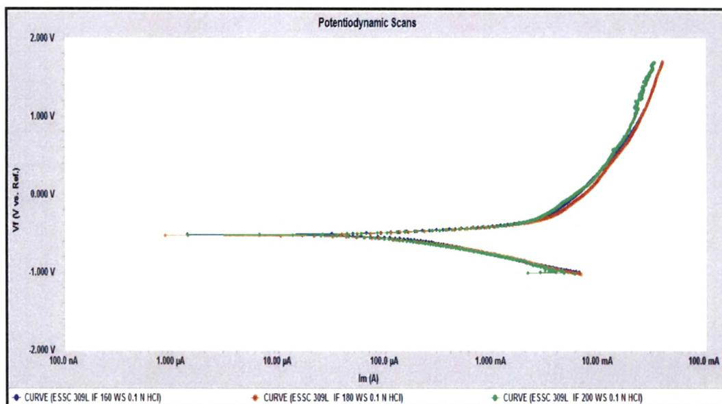
Fig. 4.65 Potentiodynamic scans of interface of 309L cladded weld overlays at different welding speed in 0.1N HCl solution
