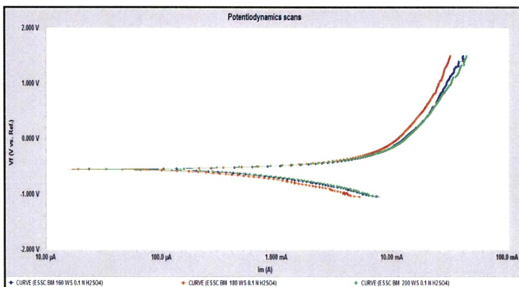
Fig. 4.68 : Potentiodynamic scans of Base Metal at different WS in 0.1N H<sub>2</sub>SO<sub>4</sub> solution
