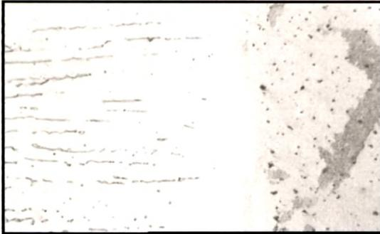
**Fig.4.149 (a)** Cladded region of 309 L Clad at 200 WS as welded condition
