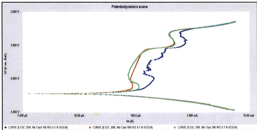
Fig. 4.71: Potentiodynamic scans of 309L Nb cladded weld overlays at different welding speed in 0.1N H<sub>2</sub>SO<sub>4</sub> solution
