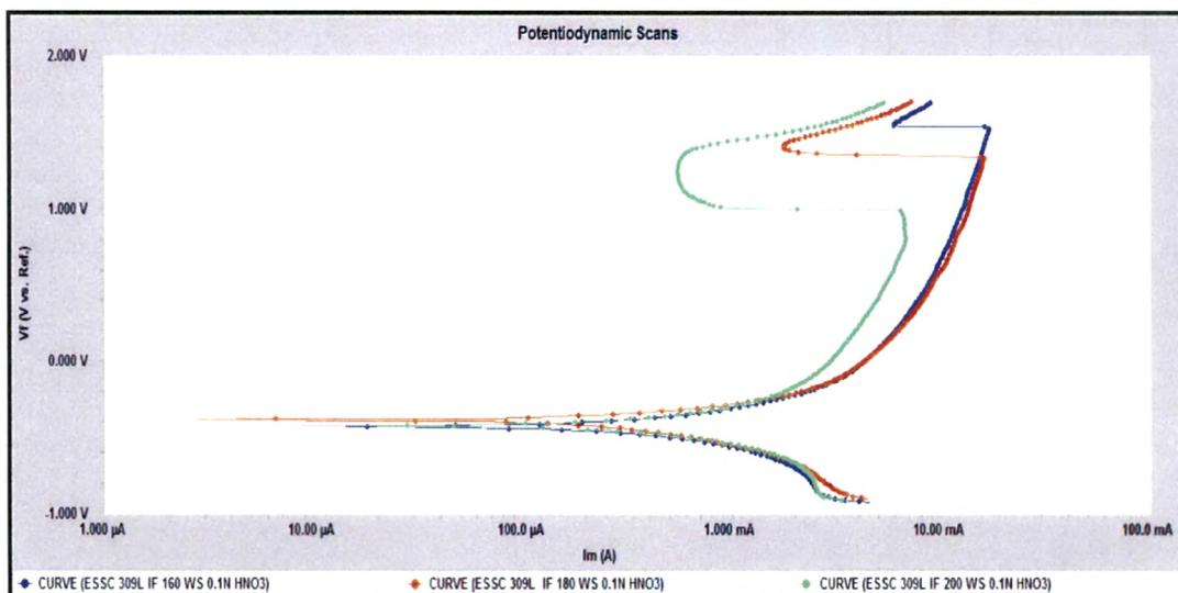
Fig. 4.60: Potentiodynamic scans of interface of 309L cladded weld overlays at different welding speed in 0.1N HNO<sub>3</sub> solution
