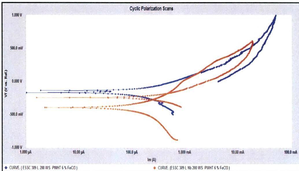
Fig. 4.125 : Cyclic polarization scans of 309 L & 309 L Nb cladded weld overlay develop with 200 mm / min. welding speed at cladded region after PWHT in 6 % FeCl<sub>3</sub> Solution
