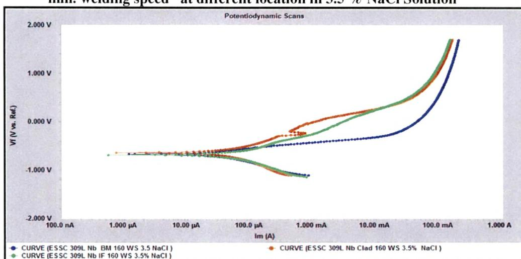
**Fig. 4.22: Potentiodynamic scans of 309 L Nb cladded weld overlay develop with 160mm / min. welding speed at different location in .5 % NaCl Solution**
