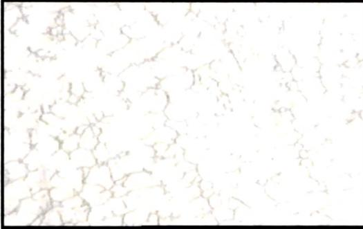
Fig.4.141 (a) Cladded region of 309 L Clad at 160 WS as welded condition
