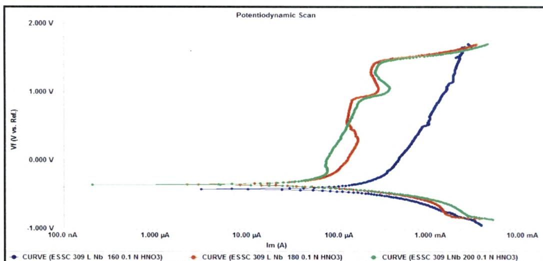
Fig. 4.61: Potentiodynamic scans of 309L Nb cladded weld overlays at different welding speed in 0.1N HNO<sub>3</sub> solution
