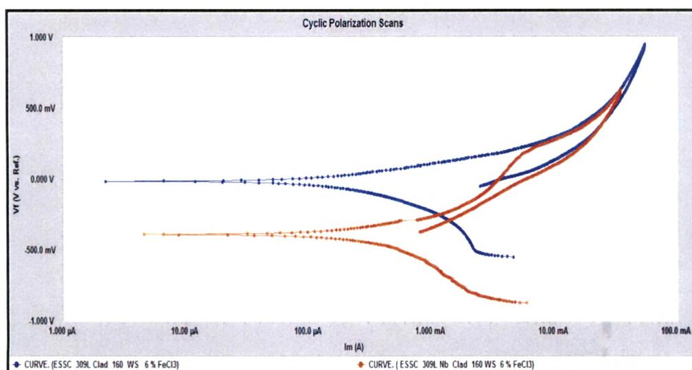
Fig. 4.117 : Cyclic polarization scans of 309 L & 309 L Nb cladded weld overlay develop with 160 mm / min. welding speed at cladded region in 6 % FeCl<sub>3</sub> Solution
