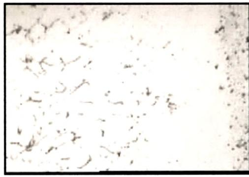
**Fig.4.32 (b) Interface region of 309 L Nb Clad 200 WS**
