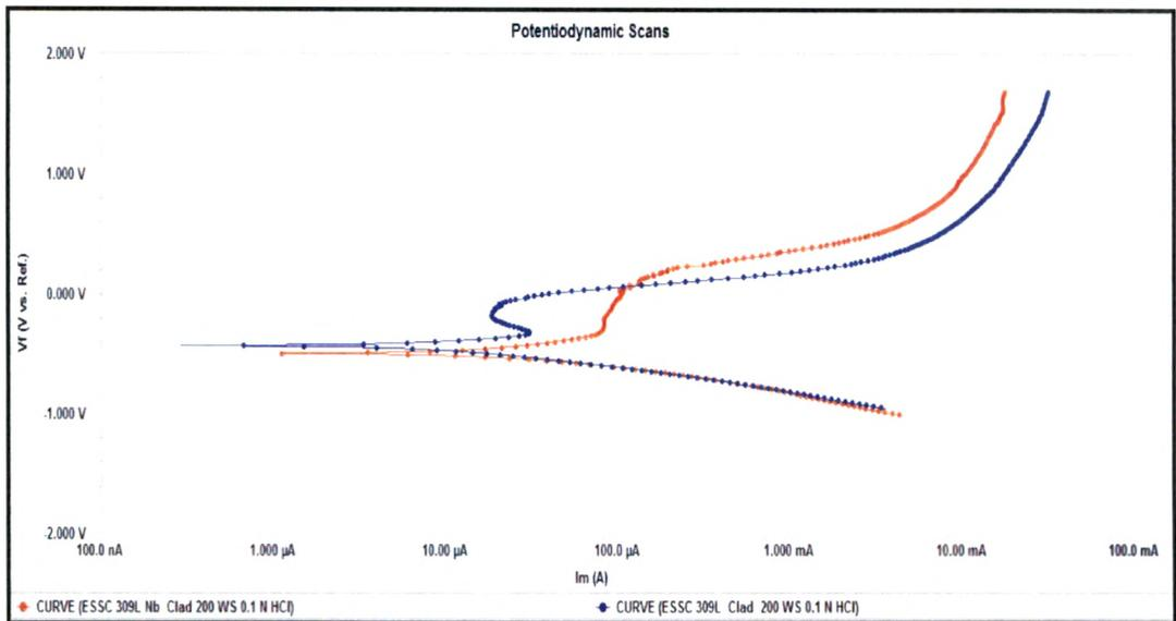
**Fig. 4.107 : Potentiodynamic scans of cladded region of 309 L & 309 L Nb cladded weld overlay develop with 200 mm / min. welding speed in 0.1 N HCl solution**
