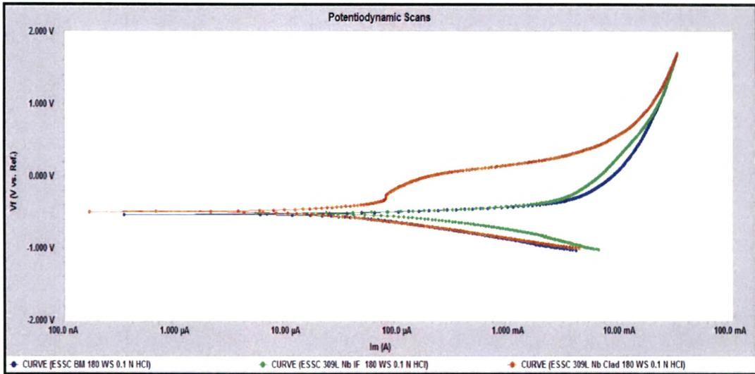
**Fig. 4.11: Potentiodynamic scans of 309 L Nb cladded weld overlay develop with 180mm / min. welding speed at different location in 0.1 N HCl Solution**
