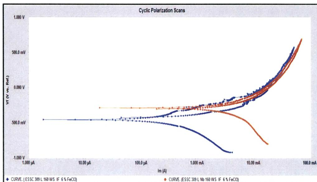
**Fig. 4.126 : Cyclic polarization scans of 309 L & 309 L Nb cladded weld overlay develop with 160 mm / min. welding speed at interface region after PWHT in 6 % FeCl<sub>3</sub> Solution**
