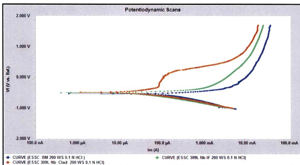
Fig. 4.12: Potentiodynamic scans of 309 L Nb cladded weld overlay develop with 200 mm / min. welding speed at different location in 0.1 N HCl Solution
