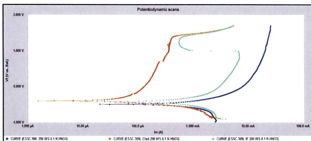
Fig. 4.3: Potentiodynamic scans of 309 L cladded weld overlay develop with 200 mm / min. welding speed at different location in 0.1 N HHO<sub>3</sub> Solution
