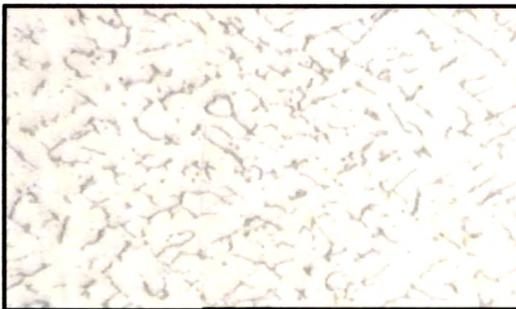
**Fig.4.146 (a) Cladded region of 309 L Nb Clad 200 WS**
