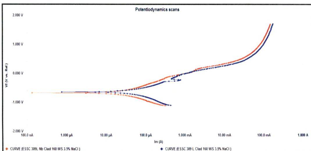
Fig. 4.111: Potentiodynamic scans of cladded region of 309 L & 309 L Nb cladded weld overlay develop with 160 mm / min. welding speed in 3.5 % NaCl solution
