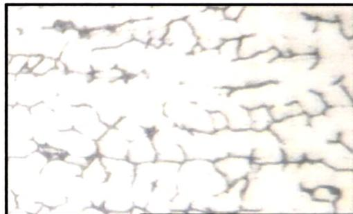
**Fig.4.146 (b) Cladded region of 309 L Nb Clad at 200 WS after PWHT**
