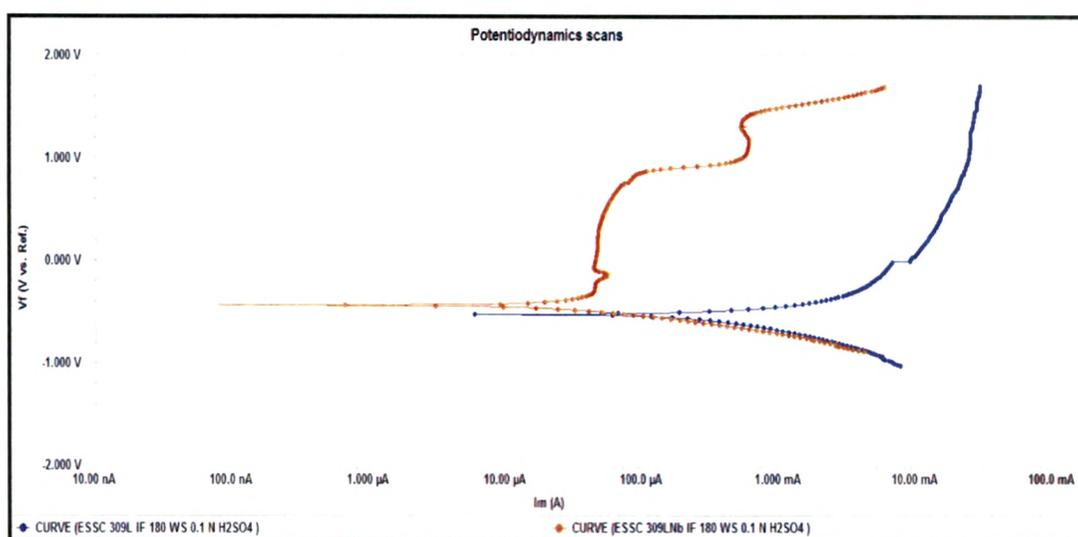
Fig. 4.103 : Potentiodynamic scans of Interface region of 309 L & 309 L Nb clad weld overlay develop with 180 mm / min. welding speed in 0.1 N H<sub>2</sub>SO<sub>4</sub> solution
