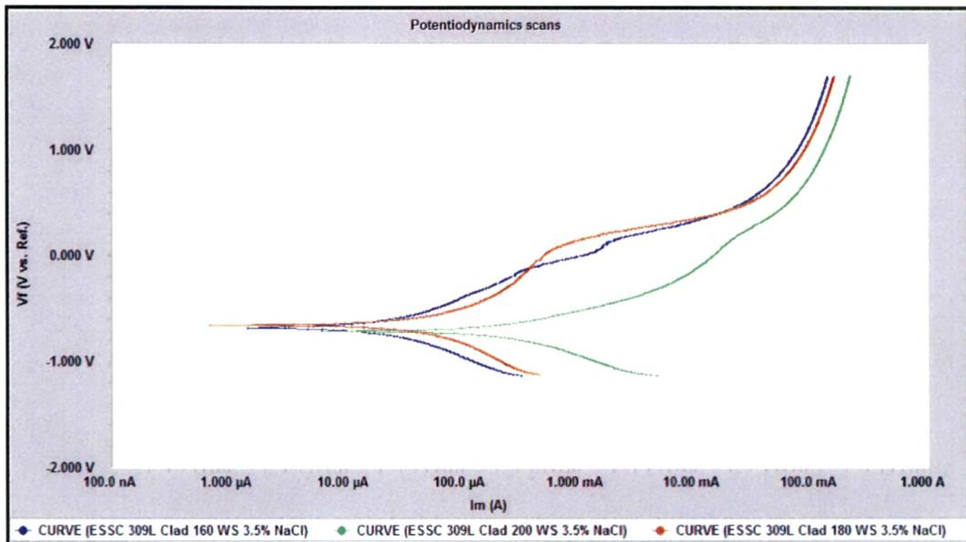
**Fig. 4.74 : Potentiodynamic scans of 309L cladded weld overlays at different welding speed in 3.5 % NaCl solution**
