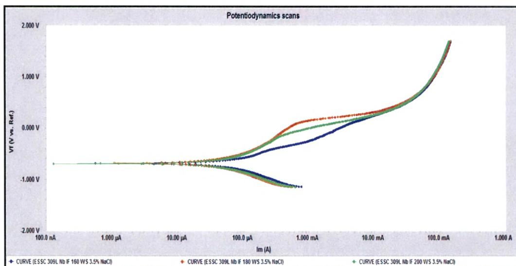
Fig. 4.77: Potentiodynamic scans of interface of 309L Nb cladded weld overlays at different welding speed in 3.5 % NaCl solution
