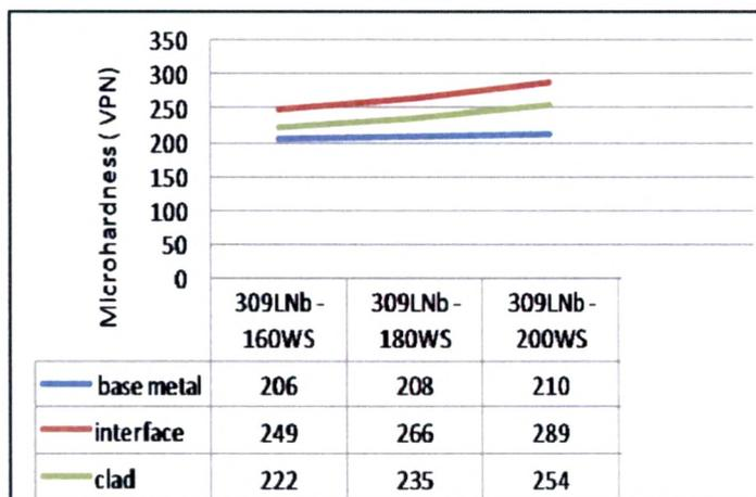
Fig-4.57 Effect of welding speed on Hardness Value of 309 L Nb cladded weld overlay
