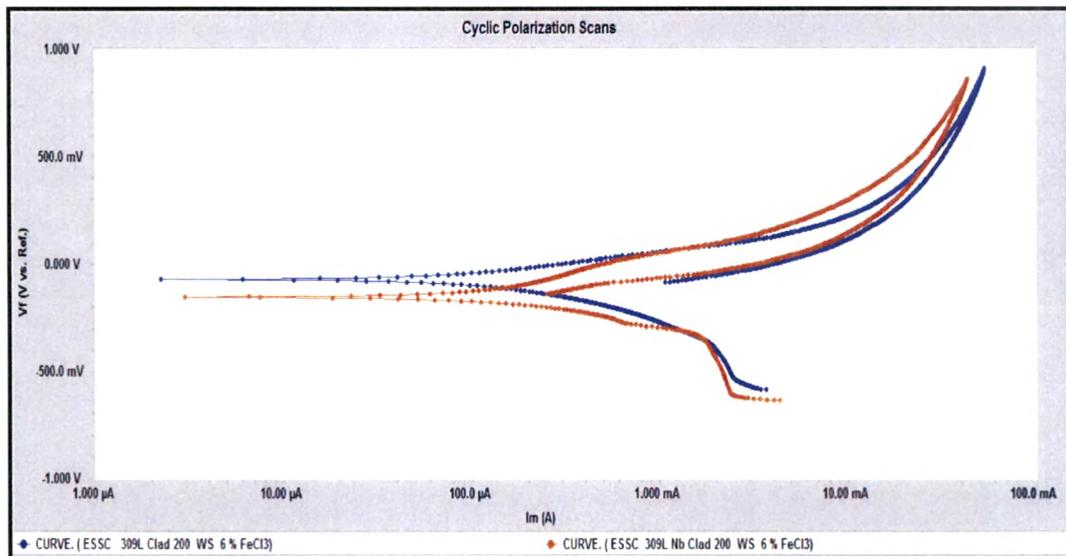
**Fig. 4.119 : Cyclic polarization scans of 309 L & 309 L Nb cladded weld overlay develop with 200 mm / min. welding speed at cladded region in 6 % FeCl<sub>3</sub> Solution**
