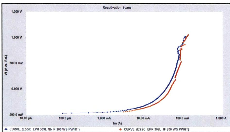
Fig. 4.140 : EPR scans of interface region of 309 L & 309 L Nb cladded weld overlay developed with 200 mm / min. welding speed in 0.1 H<sub>2</sub>SO<sub>4</sub> + 0.01 M NaCl Solution after PWHT
