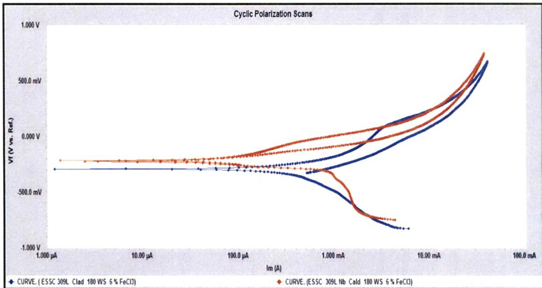
Fig.4.118 Cyclic polarization scans of 309 L & 309 L Nb cladded weld overlay develop with 180 mm / min. welding speed at cladded region in 6 % FeCl<sub>3</sub> Solution
