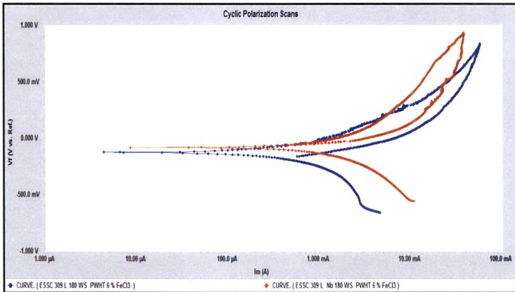
**Fig. 4.124 : Cyclic polarization scans of 309 L & 309 L Nb cladded weld overlay develop with 180 mm / min. welding speed at cladded region after PWHT in 6 % FeCl<sub>3</sub> Solution**
