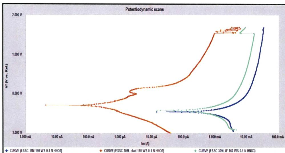
Fig. 4.1: Potentiodynamic scans of 309 L cladded weld overlay develop with 160mm / min. welding speed at different locations in 0.1 N  $\text{HNO}_3$  Solution
