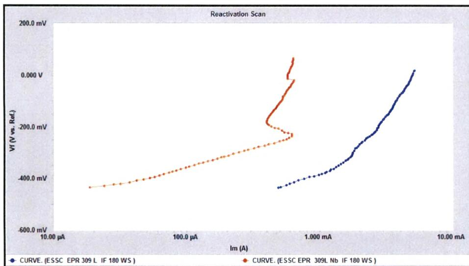
Fig. 4.133 : EPR scans of interface region of 309 L & 309 L Nb clad weld overlays developed with 180 mm / min. welding speed in 0.1 H<sub>2</sub>SO<sub>4</sub> + 0.01 M NaCl Solution
