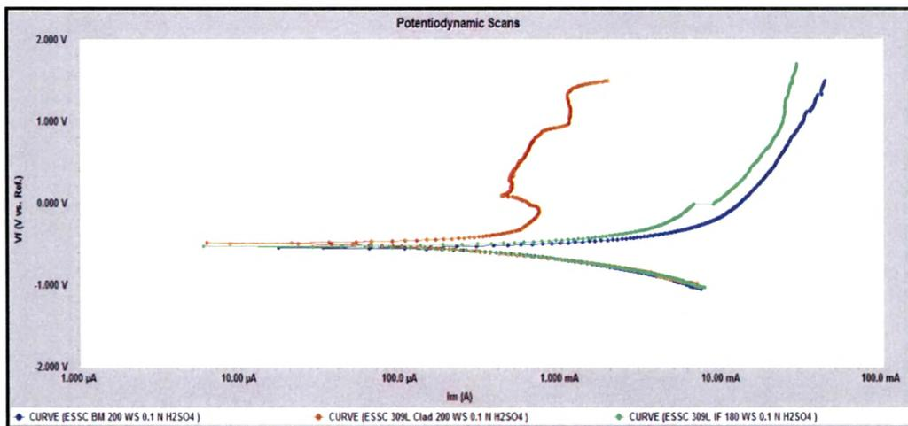
**Fig. 4.15: Potentiodynamic scans of 309 L cladded weld overlay develop with 200 mm / min. welding speed at different location in 0.1 N H<sub>2</sub>SO<sub>4</sub> Solution**
