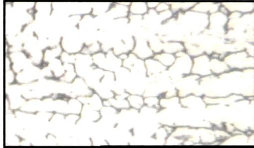
**Fig.4.144 (b) Cladded region of 309 L Nb Clad at 160 WS after PWHT**
