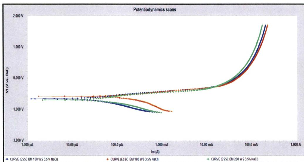
Fig. 4.73: Potentiodynamic scans of Base Metal at different WS in 3.5 % NaCl solution
