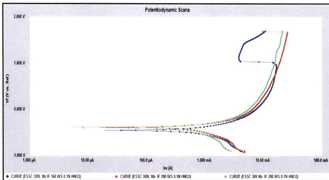
Fig.4.62 : Potentiodynamic scans of interface of 309L Nb cladded weld overlays at different welding speed in 0.1N HNO<sub>3</sub> solution
