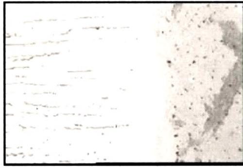
**Fig.4.29 (b) Interface region of 309 L Clad 200 WS**
