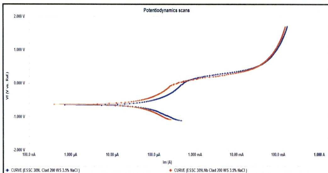
Fig. 4.113: Potentiodynamic scans of cladded region of 309 L & 309 L Nb cladded weld overlay develop with 200 mm / min. welding speed in 3.5 % NaCl solution
