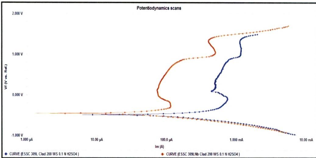
**Fig. 4.101 : Potentiodynamic scans of cladded region of 309 L & 309 L Nb cladded weld overlay develop with 200 mm / min. welding speed in 0.1 N H<sub>2</sub>SO<sub>4</sub> solution**
