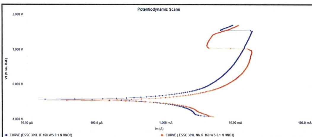
Fig. 4.96 Potentiodynamic scans of Interface region of 309 L & 309 L Nb cladded weld overlay develop with 160 mm / min. welding speed in 0.1 N HHO<sub>3</sub> Solution
