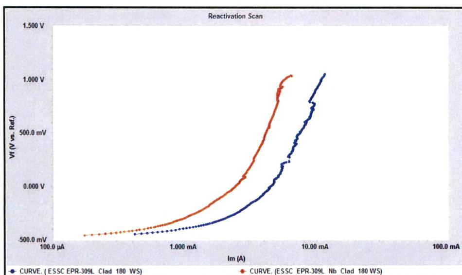
Fig. 4.130 : EPR scans of clad region of 309 L & 309 L Nb clad weld overlays developed with 180 mm / min. welding speed in 0.1  $\text{H}_2\text{SO}_4$  + 0.01 M NaCl Solution
