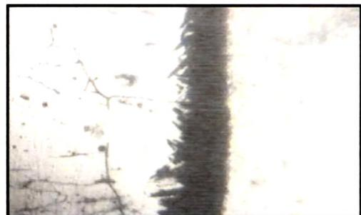
**Fig.4.148 (b) Interface region of 309 L Clad at 180 WS after PWHT**
