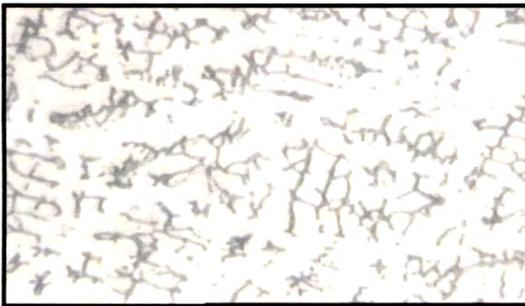
Fig.4.142 (a) Cladded region of 309 L Clad at 180 WS as welded condition
