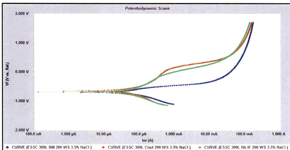
**Fig. 4.24: Potentiodynamic scans of 309 L Nb cladded weld overlay develop with 200 mm / min. welding speed at different location in .5 % NaCl Solution**
