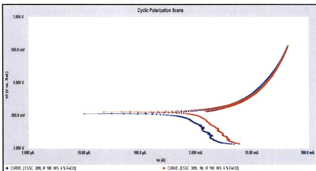
Fig. 4.121 : Cyclic polarization scans of 309 L & 309 L Nb cladded weld overlay develop with 180 mm / min. welding speed at interface region in 6 % FeCl<sub>3</sub> Solution
