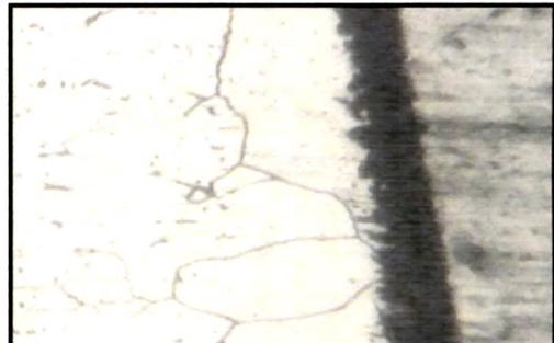
**Fig.4.150 (b)** Interface region of 309 L Nb Clad at 160 WS after PWHT
