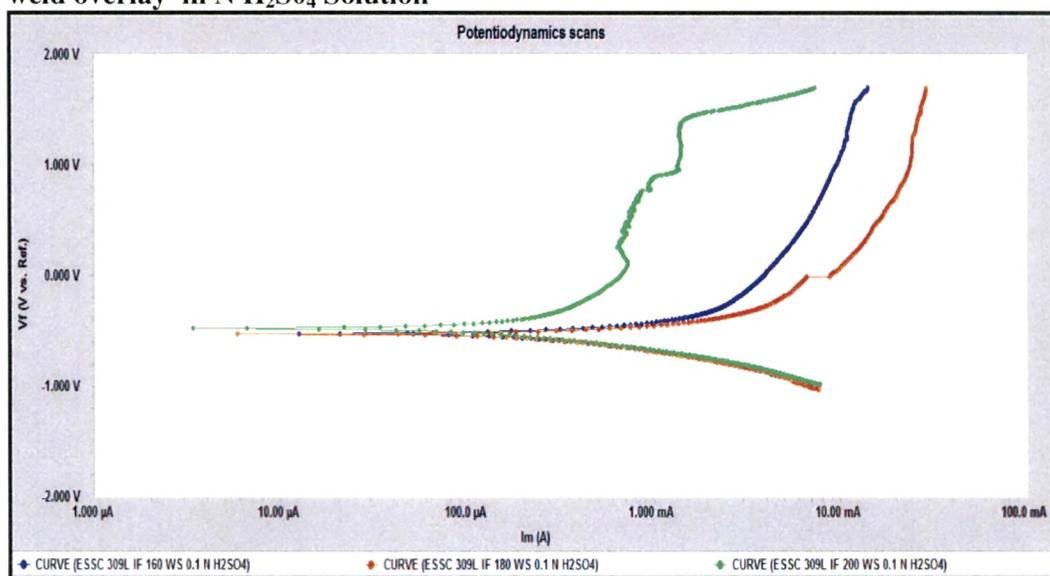
Fig. 4.70 : Potentiodynamic scans of interface of 309L cladded weld overlays at different welding speed in 0.1N H<sub>2</sub>SO<sub>4</sub> solution
