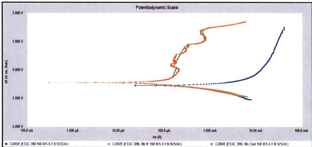
Fig. 4.16: Potentiodynamic scans of 309 L Nb cladded weld overlay develop with 160mm / min. welding speed at different location in 0.1 N H<sub>2</sub>SO<sub>4</sub> Solution
