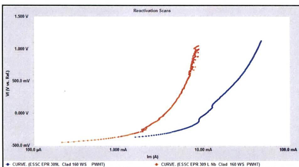
Fig. 4.135 : EPR scans of clad region of 309 L & 309 L Nb clad weld overlay developed with 160 mm / min. welding speed in 0.1 H<sub>2</sub>SO<sub>4</sub> + 0.01 M NaCl Solution after PWHT
