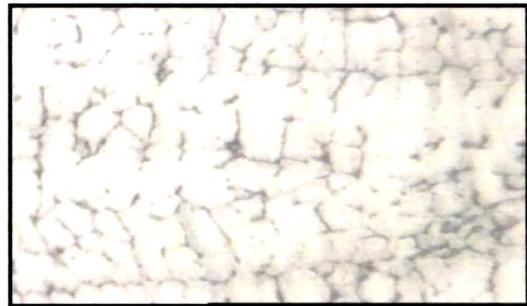
Fig. 4.142 (b) Cladded region of 309 L Clad at 180 WS after PWHT
