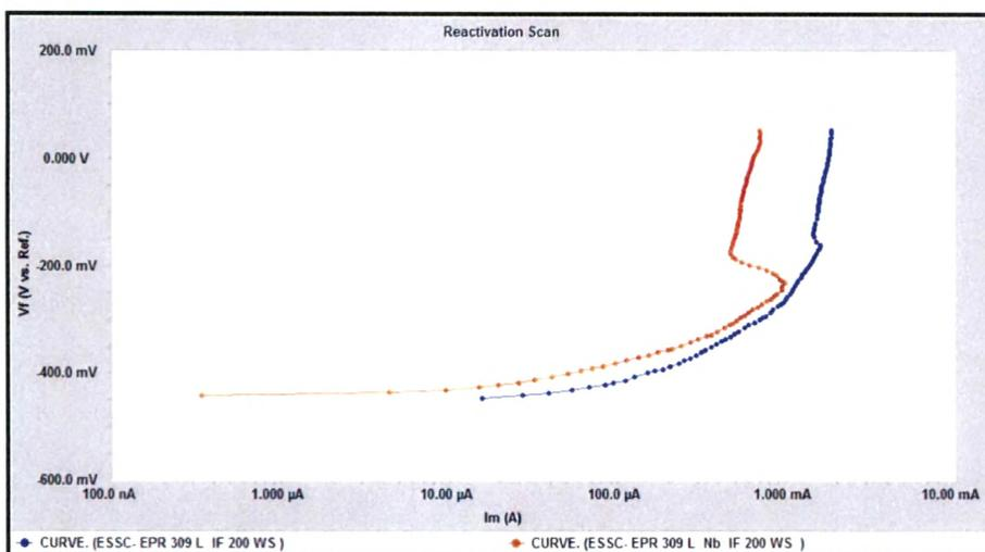
Fig.4.134 : EPR scans of interface region of 309 L & 309 L Nb cladded weld overlays developed with 200 mm / min. welding speed in 0.1 H<sub>2</sub>SO<sub>4</sub> + 0.01 M NaCl Solution
