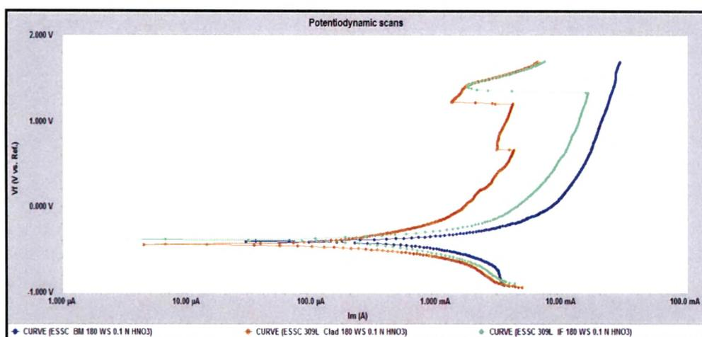
Fig. 4.2: Potentiodynamic scans of 309 L cladded weld overlay develop with 180mm / min. welding speed at different location in 0.1 N HHO<sub>3</sub> Solution
