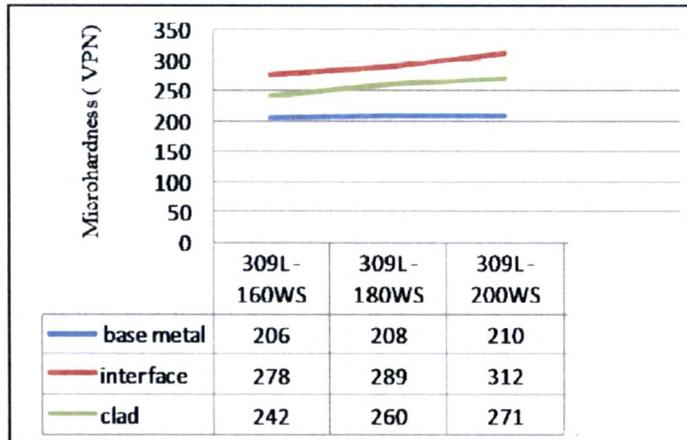
Fig-4.56 Effect of welding speed on Hardness Value of 309 L cladded weld overlay
