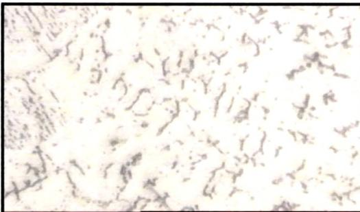
Fig.4.143 (a) Cladded region of 309 L Clad at 200 WS as welded condition
