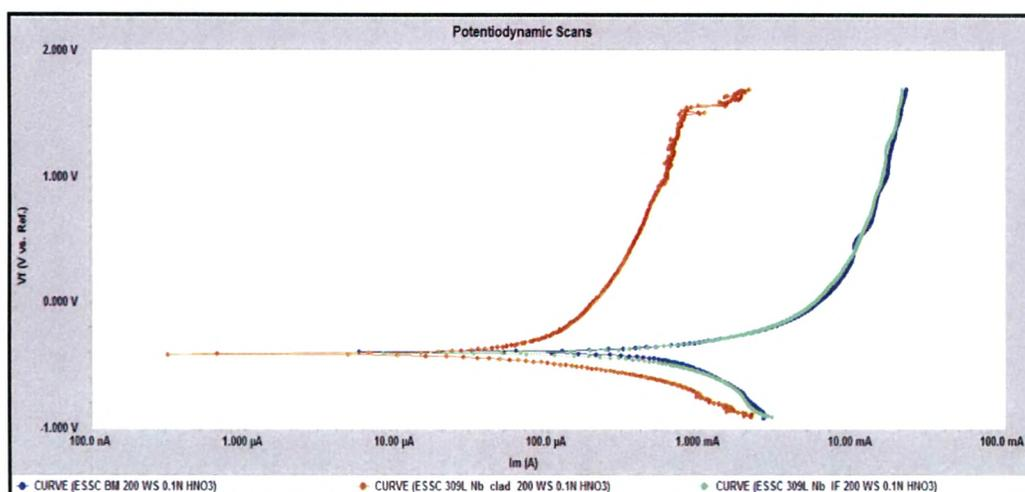
Fig. 4.6: Potentiodynamic scans of 309 L Nb cladded weld overlay develop with 200 mm / min. welding speed at different location in 0.1 N HHO<sub>3</sub> Solution
