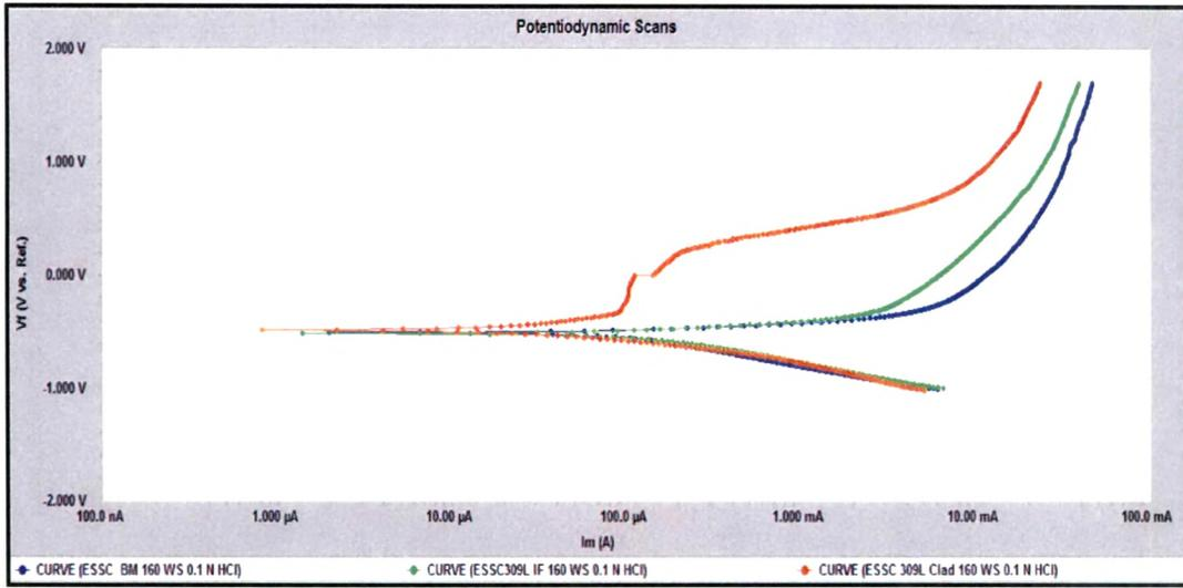
**Fig. 4.7 Potentiodynamic scans of 309 L cladded weld overlay develop with 160mm / min. welding speed at different location in 0.1 N HCl Solution**
