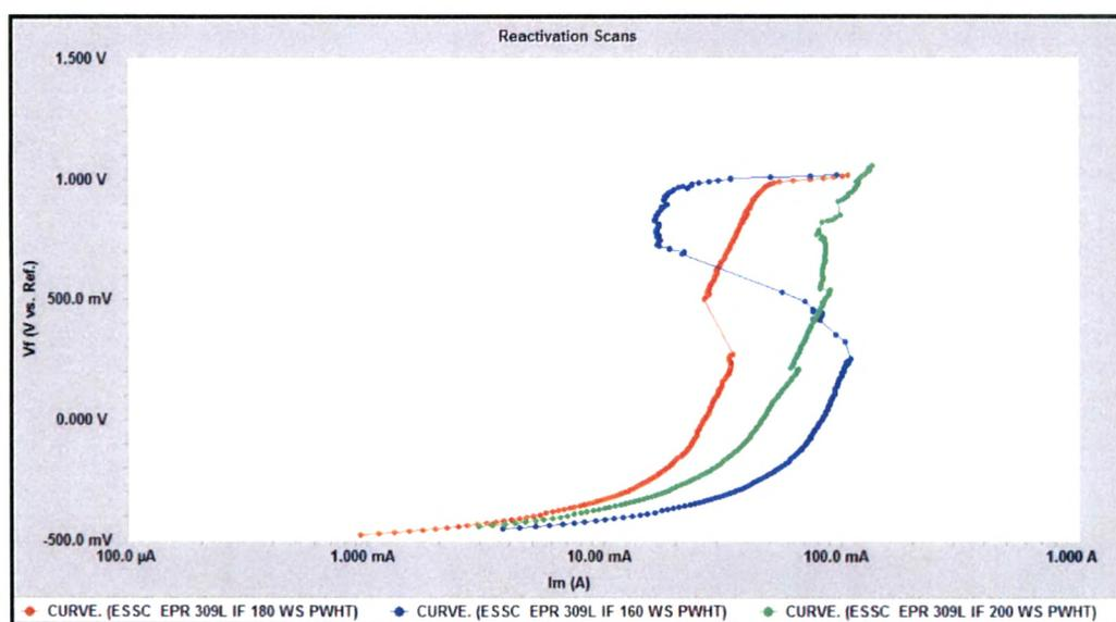
Fig. 4.160 : EPR scans of interface of 309L cladded weld overlays after PWHT at different welding speed in 0.1 H<sub>2</sub>SO<sub>4</sub> + 0.01 M NaCl Solution
