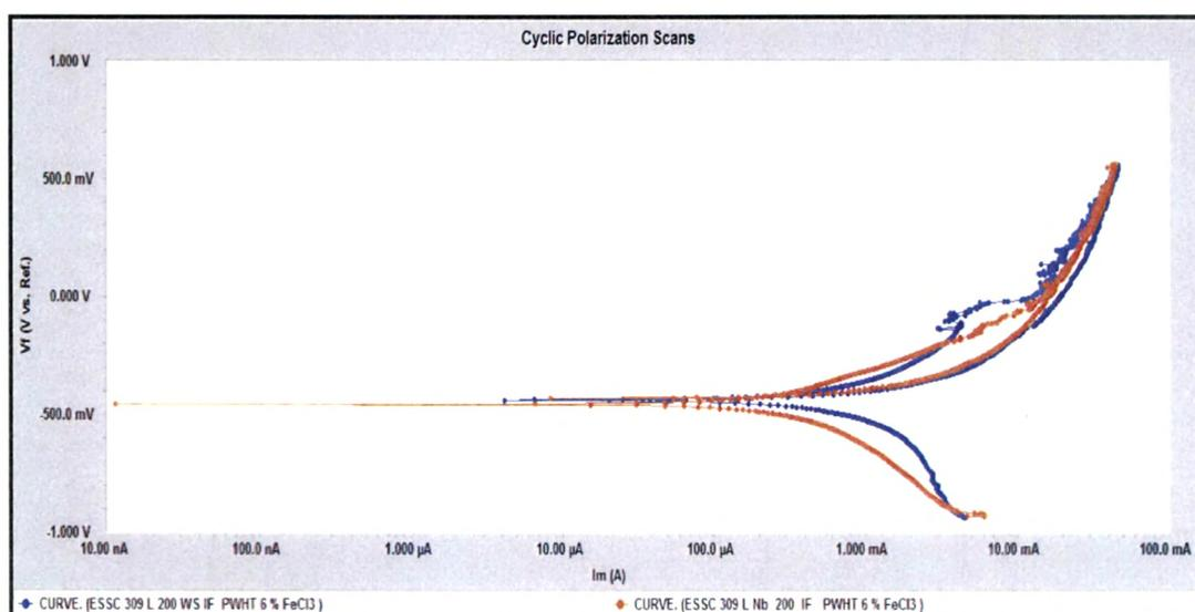
**Fig. 4.128 : Cyclic polarization scans of 309 L & 309 L Nb cladded weld overlay develop with 200 mm / min. welding speed at interface region after PWHT in 6 % FeCl<sub>3</sub> Solution**
