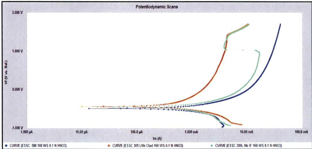
**Fig. 4.5: Potentiodynamic scans of 309 L Nb cladded weld overlay develop with 180mm / min. welding speed at different location in 0.1 N HHO<sub>3</sub>Solution**
