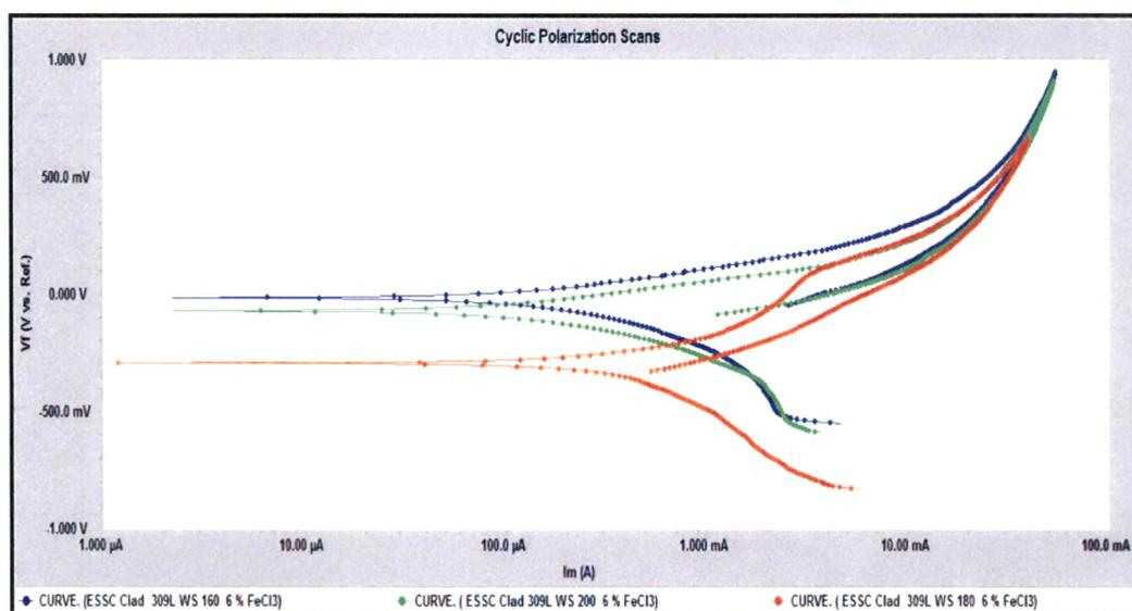
Fig. 4.79 : cyclic polarization scans of 309L clad weld overlays at different welding speed in 6% FeCl<sub>3</sub> Solution
