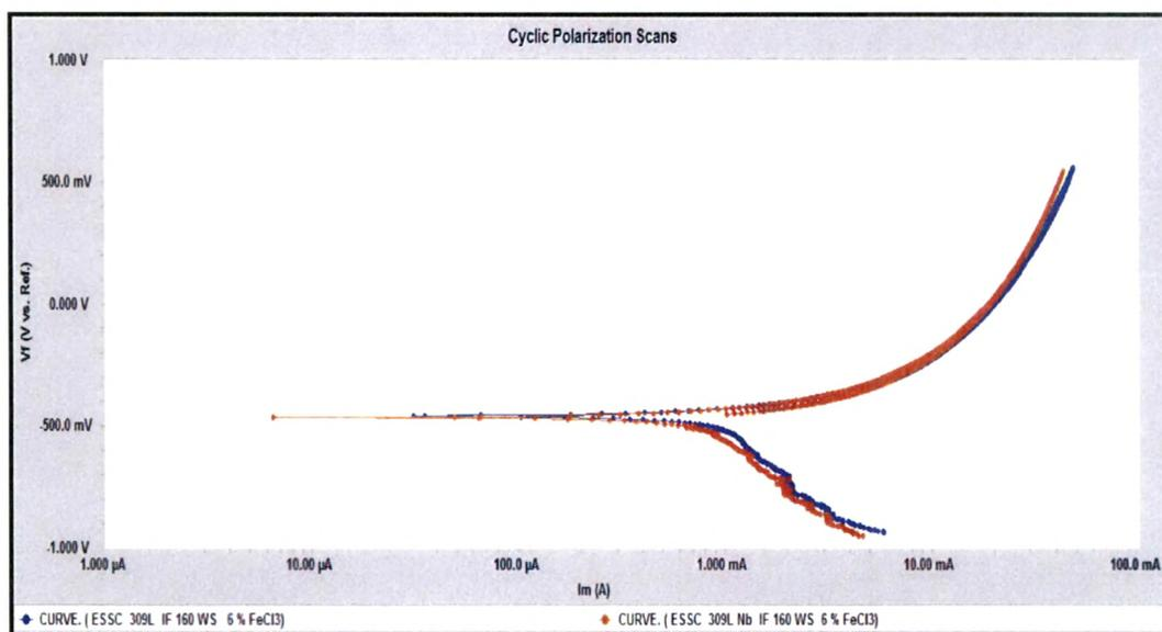
Fig. 4.120 : Cyclic polarization scans of 309 L & 309 L Nb cladded weld overlay develop with 160 mm / min. welding speed at interface region in 6 % FeCl<sub>3</sub> Solution
