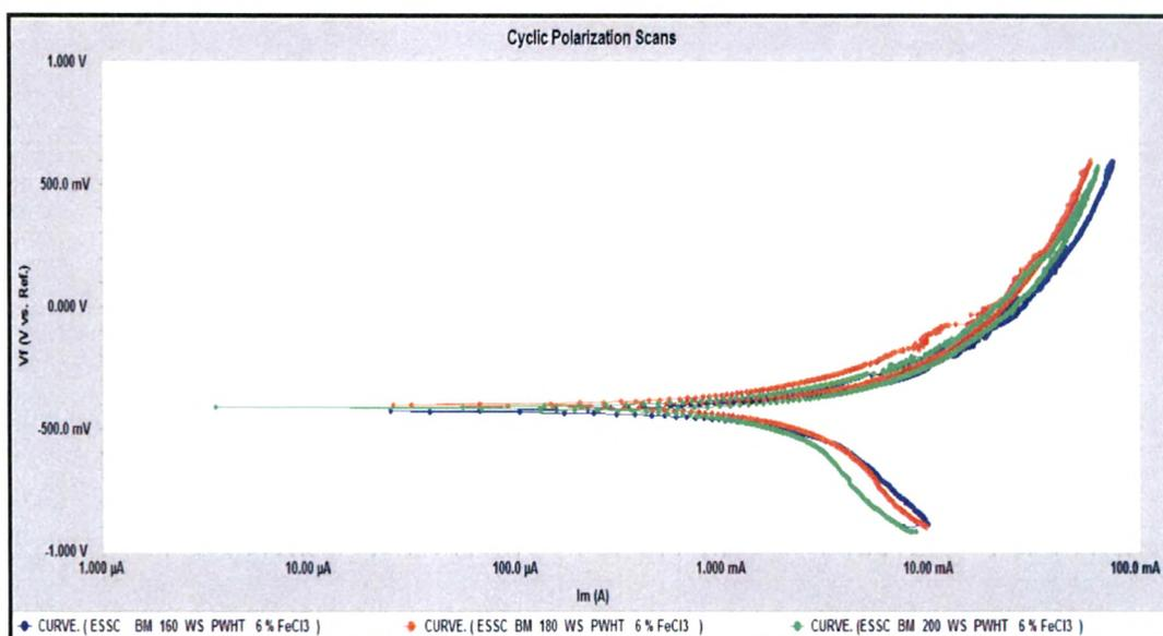
Fig. 4.153 Cyclic polarization scans of base metal at different welding speed after PWHT in 6% FeCl<sub>3</sub> Solution
