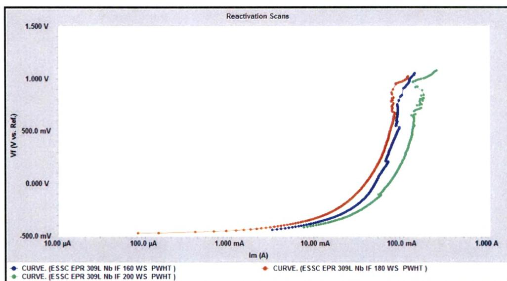
Fig. 4.161 : EPR scans of interface of 309LNb cladded weld overlays after PWHT at different welding speeds in 0.1 H<sub>2</sub>SO<sub>4</sub> + 0.01 M NaCl Solution
