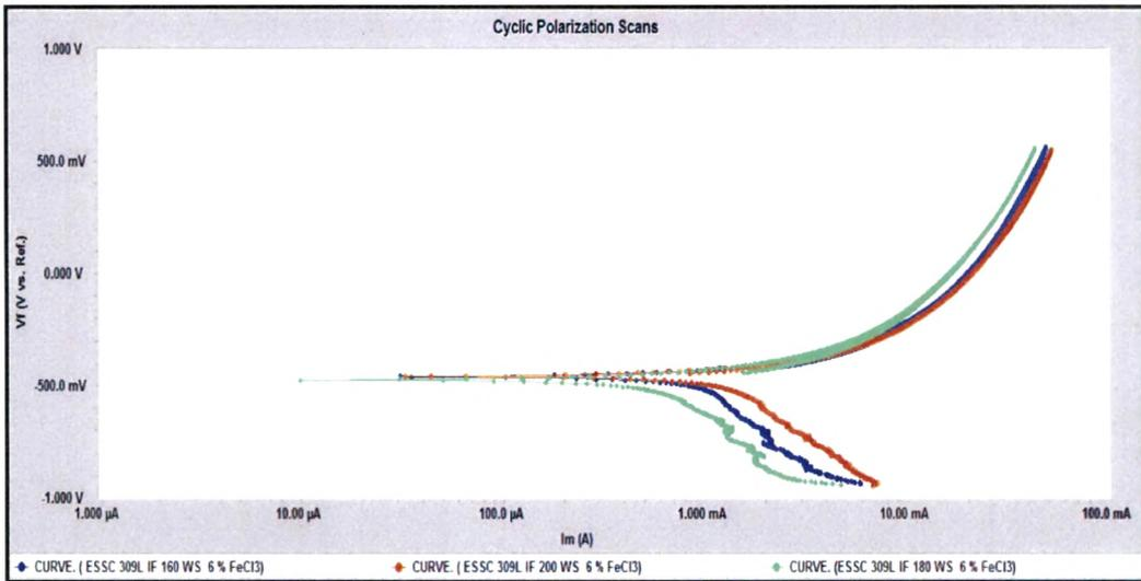
**Fig. 4.81 : cyclic polarization scans of Interface 309L cladded weld overlays at different welding speed in 6% FeCl<sub>3</sub> Solution**
