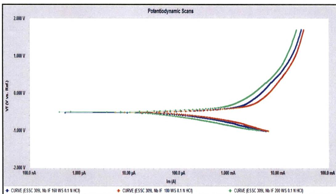
Fig. 4.67 : Potentiodynamic scans of interface of 309L Nb cladded weld overlays at different welding speed in 0.1N HCl solution
