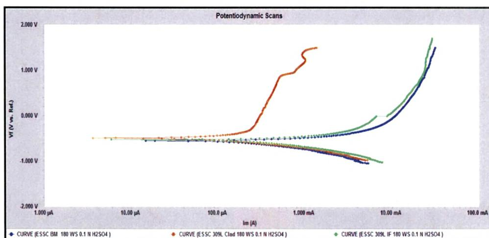
Fig. 4.14: Potentiodynamic scans of 309 L cladded weld overlay develop with 180mm / min. welding speed at different location in 0.1 N H<sub>2</sub>SO<sub>4</sub> Solution
