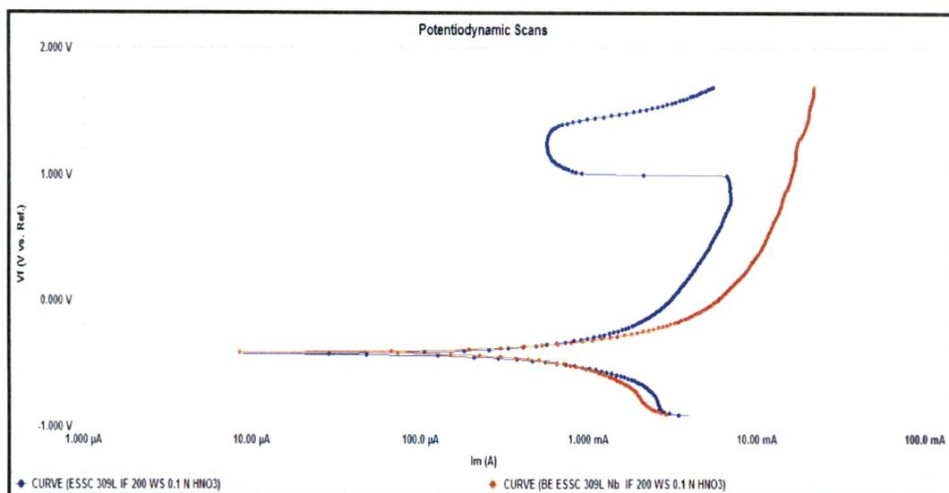
**Fig. 4.98** Potentiodynamic scans of Interface region of 309 L & 309 L Nb cladded weld overlay develop with 200 mm / min. welding speed in 0.1 N HHO<sub>3</sub> Solution
