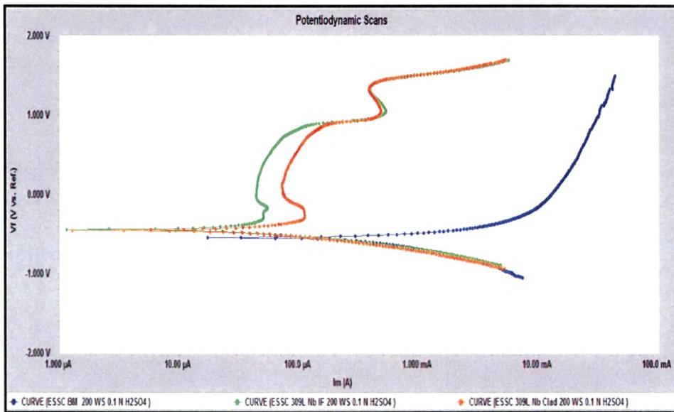
Fig. 4.18: Potentiodynamic scans of 309 L Nb cladded weld overlay develop with 200 mm / min. welding speed at different location in 0.1 N H<sub>2</sub>SO<sub>4</sub> Solution
