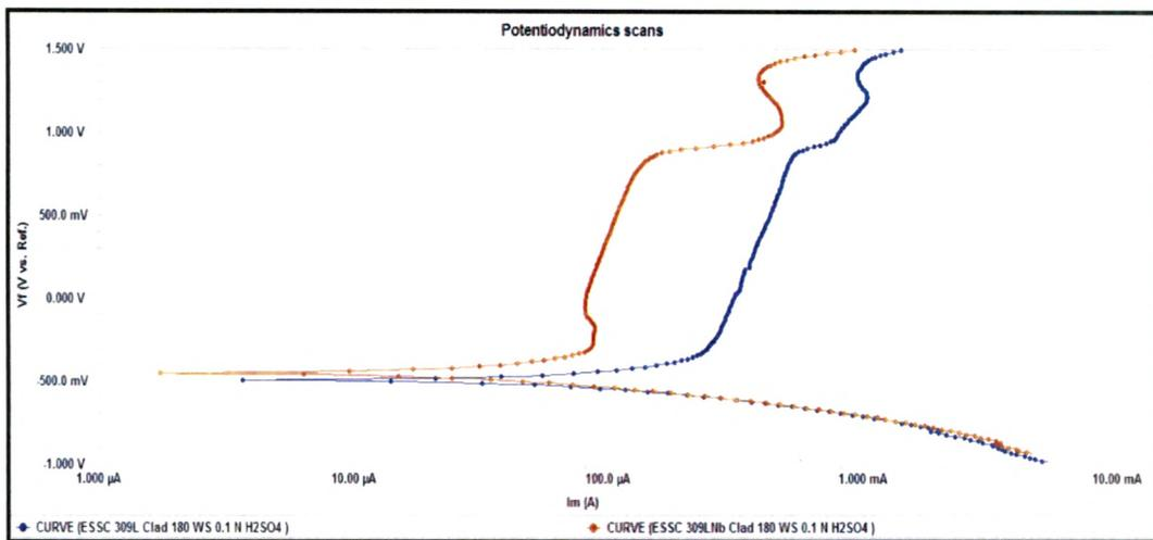
**Fig. 4.100 Potentiodynamic scans of cladded region of 309 L & 309 L Nb cladded weld overlay develop with 180 mm / min. welding speed in 0.1 N H<sub>2</sub>SO<sub>4</sub> solution**
