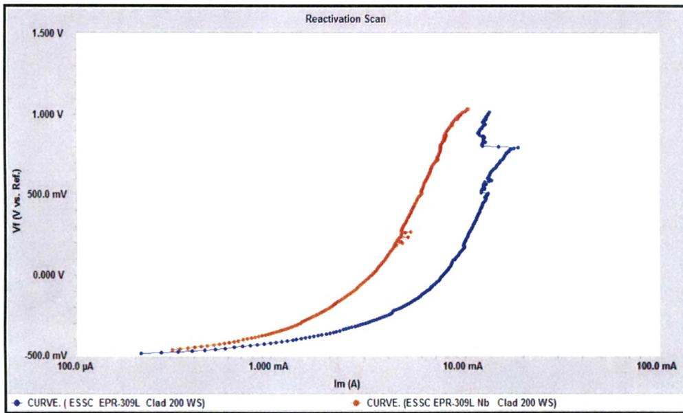
**Fig. 4.131 : EPR scans of cladded region of 309 L & 309 L Nb cladded weld overlays developed with 200 mm / min. welding speed in 0.1 H<sub>2</sub>SO<sub>4</sub> + 0.01 M NaCl Solution**
