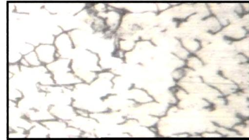
**Fig.4.145 (b) Cladded region of 309 L Nb Clad at 180 WS after PWHT**
