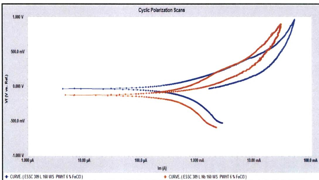
Fig. 4.123 : Cyclic polarization scans of 309 L & 309 L Nb clad weld overlay develop with 160 mm / min. welding speed at clad region after PWHT in 6 % FeCl<sub>3</sub> Solution
