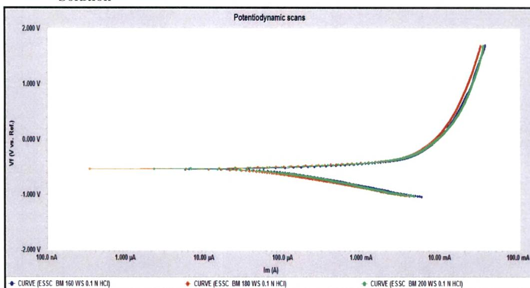
Fig. 4.63: Potentiodynamic scans of Base metal at different welding speed in 0.1N HCl solution
