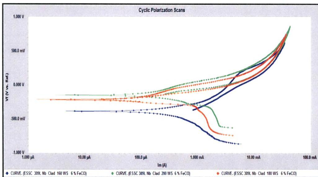
**Fig. 4.80 : cyclic polarization scans of 309LNb Cladded weld overlays at different welding speed in 6% FeCl<sub>3</sub> Solution**
