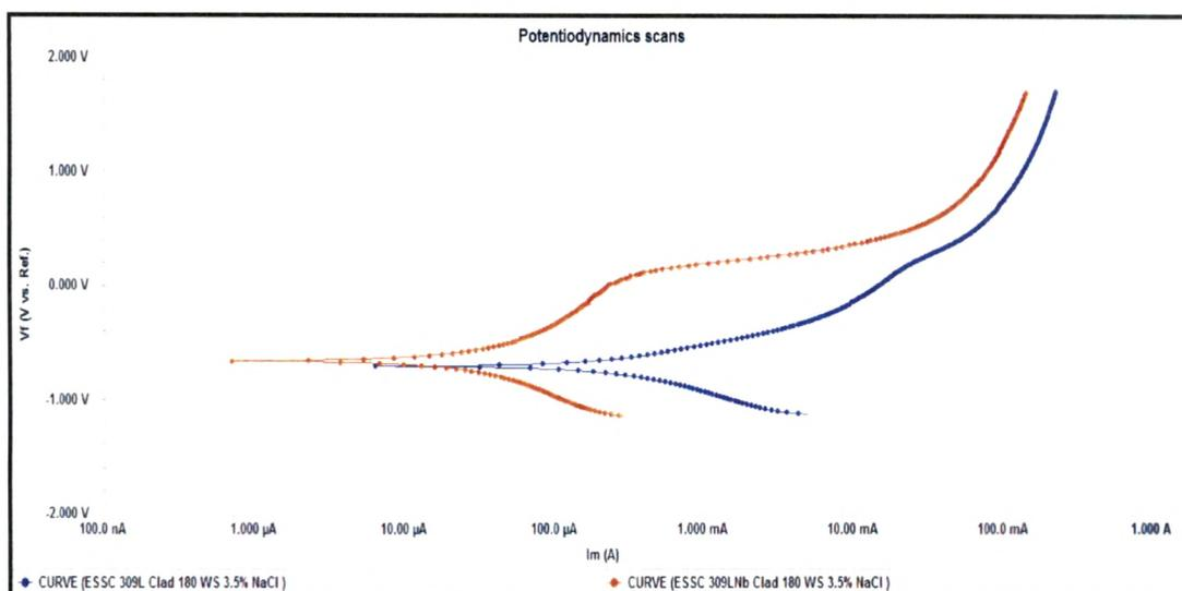
Fig. 4.112 : Potentiodynamic scans of cladded region of 309 L & 309 L Nb cladded weld overlay develop with 180 mm / min. welding speed in 3.5 % NaCl solution
