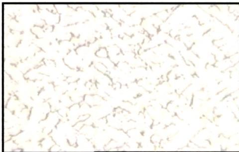
Fig. 4.89 (b) Cladded region of 309 L Nb Clad 200 WS
