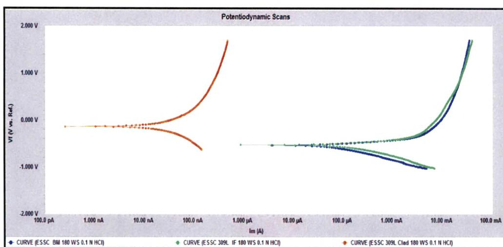
Fig.4.8 Potentiodynamic scans of 309 L clad weld overlay develop with 180mm / min. welding speed at different location in 0.1 N HCl Solution
