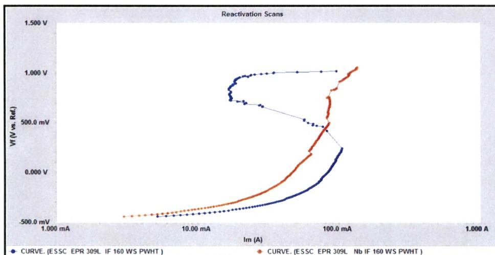
Fig. 4.138 : EPR scans of interface region of 309 L & 309 L Nb cladded weld overlay developed with 160 mm / min. welding speed in 0.1 H<sub>2</sub>SO<sub>4</sub> + 0.01 M NaCl Solution after PWHT
