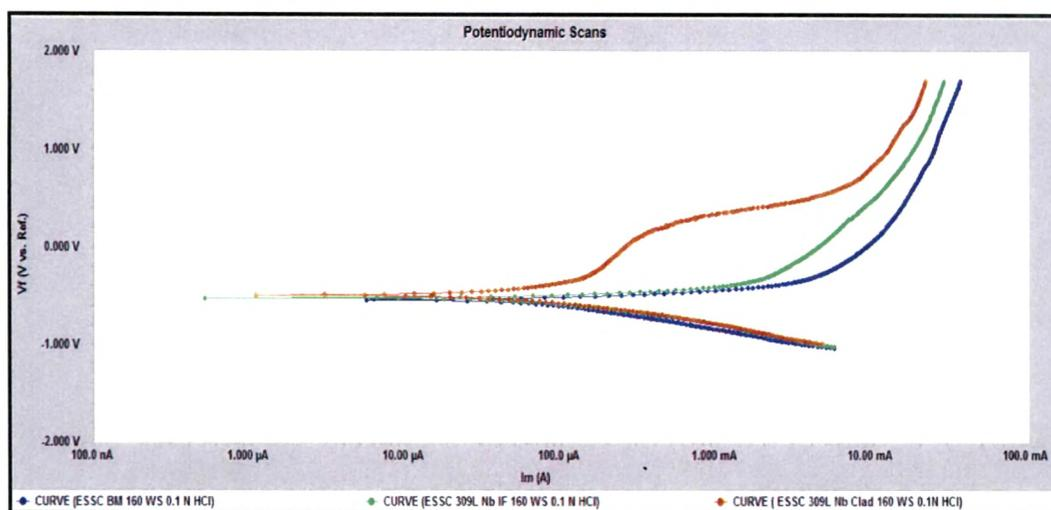
Fig. 4.10: Potentiodynamic scans of 309 L Nb cladded weld overlay develop with 160mm / min. welding speed at different location in 0.1 N HCl Solution
