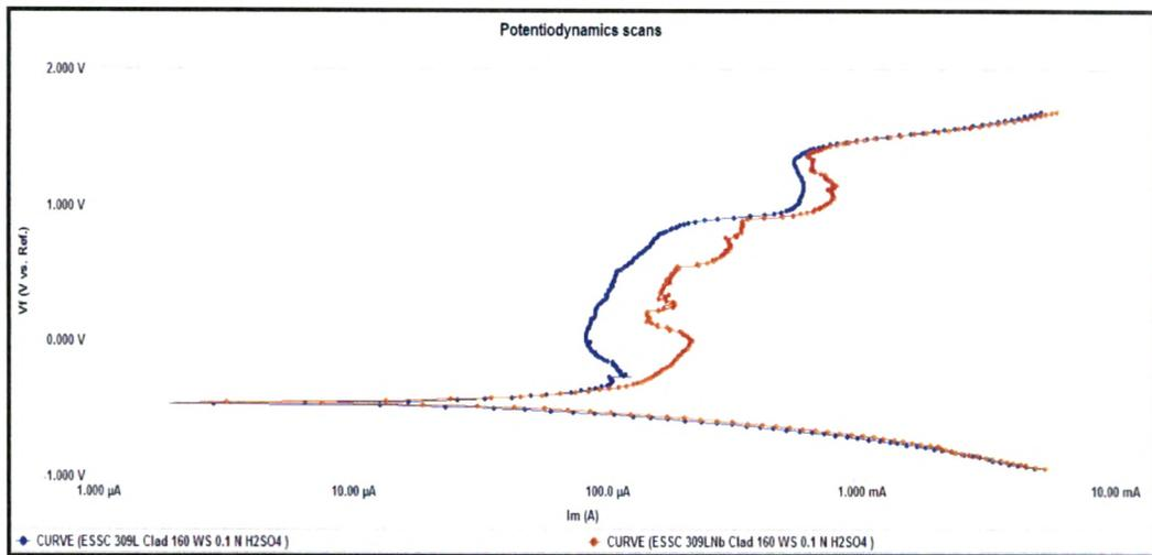
Fig. 4.99 Potentiodynamic scans of cladded region of 309 L & 309 L Nb cladded weld overlay develop with 160 mm / min. welding speed in 0.1 N H<sub>2</sub>SO<sub>4</sub> solution
