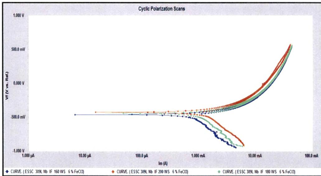
**Fig. 4.82 : cyclic polarization scans of interface 309LNb Cladded weld overlays at different welding speed in 6% FeCl<sub>3</sub> Solution**
