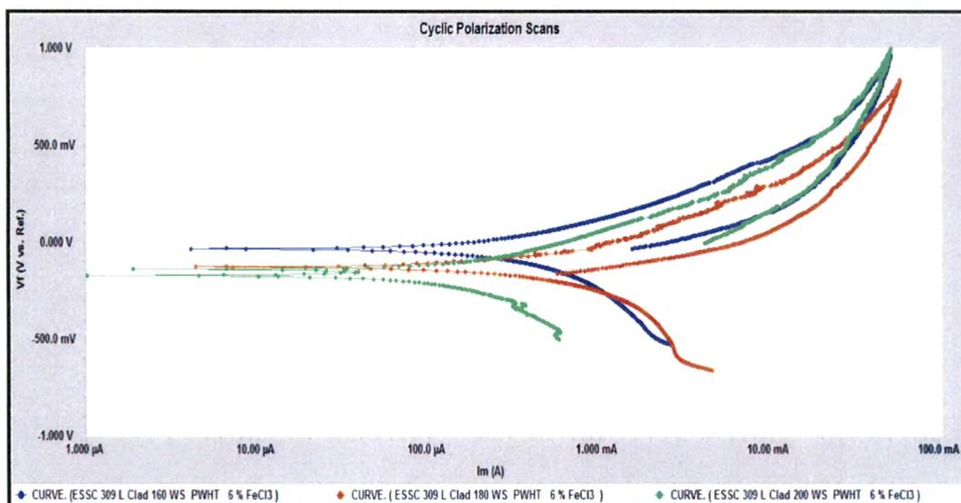
Fig. 4.154 : Cyclic polarization scans of cladded region of 309L cladded weld overlays at different welding speed after PWHT in 6% FeCl<sub>3</sub> Solution
