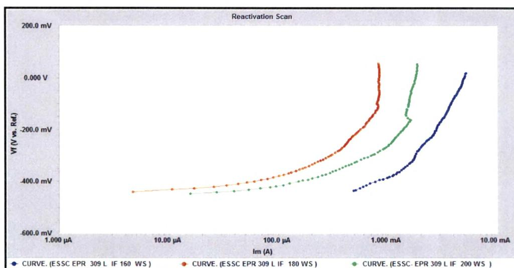
Fig. 4.84 EPR scans of interface of 309L cladded weld overlays at different welding speed in 0.1 H<sub>2</sub>SO<sub>4</sub>+ 0.01 M NaCl Solution
