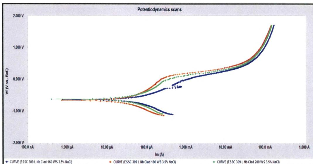
**Fig. 4.76: Potentiodynamic scans of 309L Nb cladded weld overlays at different welding speed in 3.5 % NaCl solution**
