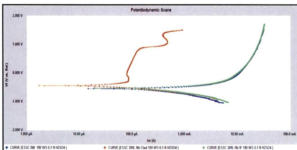
Fig. 4.17: Potentiodynamic scans of 309 L Nb cladded weld overlay develop with 180mm / min. welding speed at different location in 0.1 N H<sub>2</sub>SO<sub>4</sub> Solution
