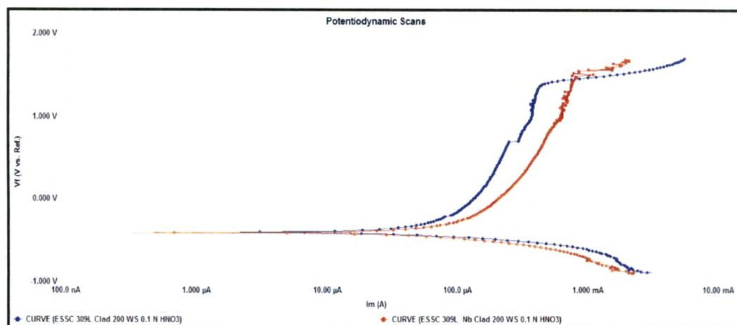
Fig. 4.95 Potentiodynamic scans of cladded region of 309 L & 309 L Nb cladded weld overlay develop with 200 mm / min. welding speed in 0.1 N HHO<sub>3</sub> Solution
