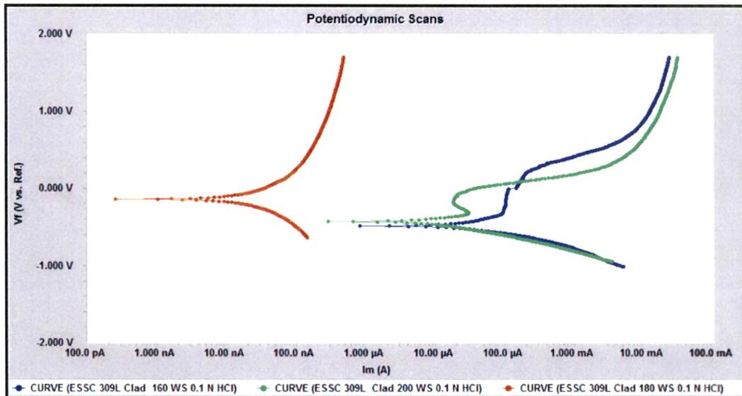
**Fig. 4.64: Potentiodynamic scans of 309L cladded weld overlays at different WS in 0.1N HCl Solution**
