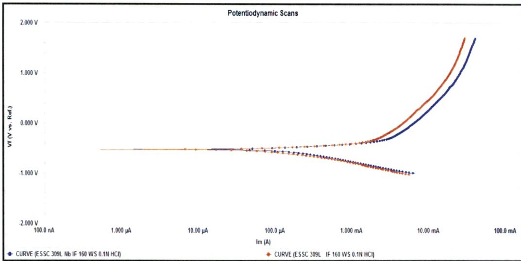
**Fig. 4.108 : Potentiodynamic scans of Interface region of 309 L & 309 L Nb cladded weld overlay develop with 160 mm / min. welding speed in 0.1 N HCl solution**
