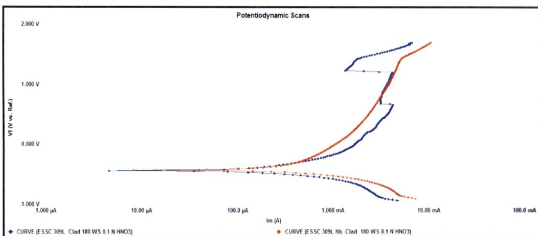
**Fig. 4.94 Potentiodynamic scans of cladded region of 309 L & 309 L Nb cladded weld overlay develop with 180 mm / min. welding speed in 0.1 N HHO<sub>3</sub> Solution**
