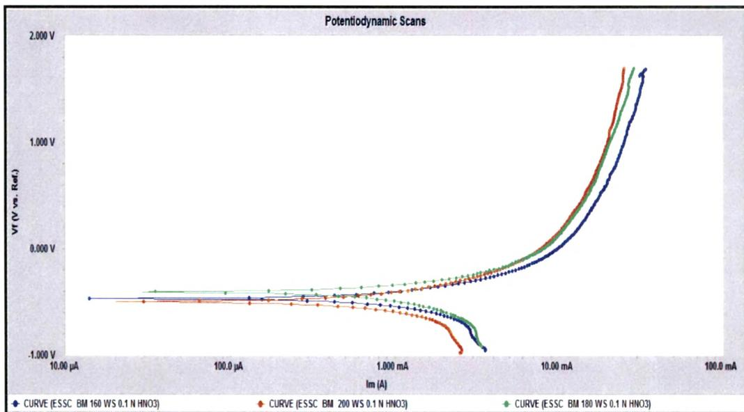
Fig. 4.58 : Potentiodynamic scans of Base Metal at different WS in 0.1N HNO<sub>3</sub> solution
