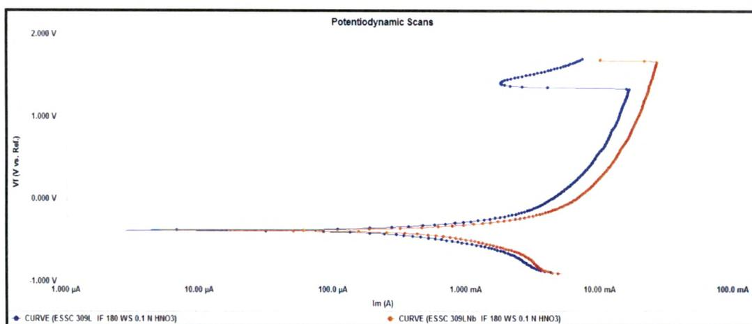
Fig. 4.97 Potentiodynamic scans of Interface region of 309 L & 309 L Nb cladded weld overlay develop with 180 mm / min. welding speed in 0.1 N HHO<sub>3</sub> Solution
