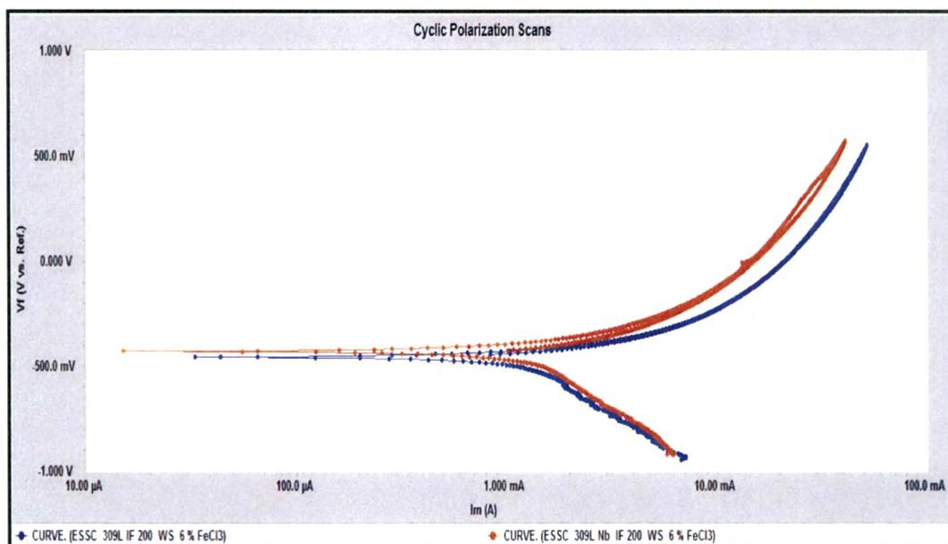
Fig. 4.122 : Cyclic polarization scans of 309 L & 309 L Nb cladded weld overlay develop with 200 mm / min. welding speed at interface region in 6 % FeCl<sub>3</sub> Solution
