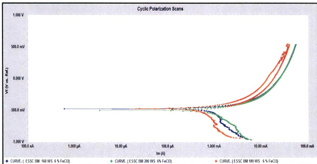
Fig. 4.78 : Cyclic polarization scans of base metal at different welding speed in 6% FeCl<sub>3</sub> Solution
