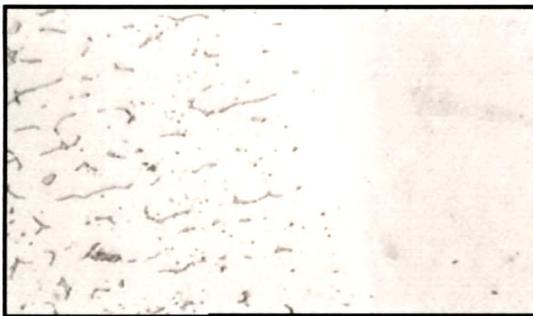
**Fig.4.147 (a) Interface region of 309 L Clad at 160 WS as welded condition**
