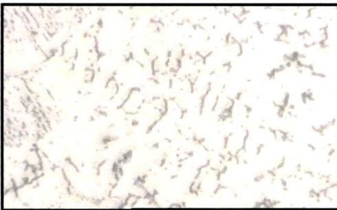
Fig. 4.89 (a) Cladded region of 309 L Clad 200 WS
