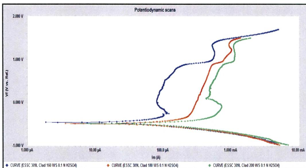
Fig. 4.69 : Potentiodynamic scans of 309L cladded weld overlays at different welding speed in 0.1N H<sub>2</sub>S<sub>0</sub><sub>4</sub> solution
