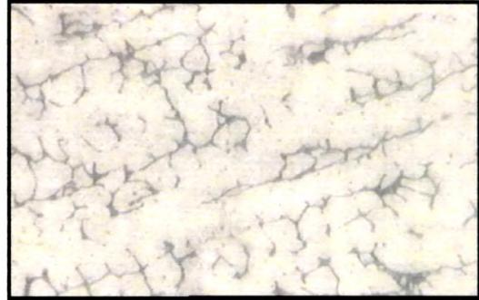
Fig.4.141 (b) Cladded region of 309 L Clad at 160 WS after PWHT
