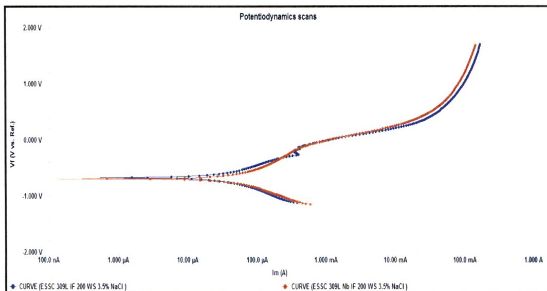
Fig. 4.116 : Potentiodynamic scans of Interface region of 309 L & 309 L Nb cladded weld overlay develop with 200 mm / min. welding speed in 3.5 % NaCl solution
