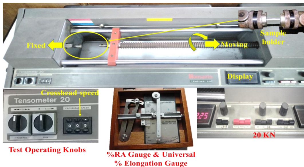
Figure 3.18 Table top tensometer for tensile testing (“MONSANTO” make Tensometer 20) with specimen holder for round samples and %RA & %EL. Gauges.
