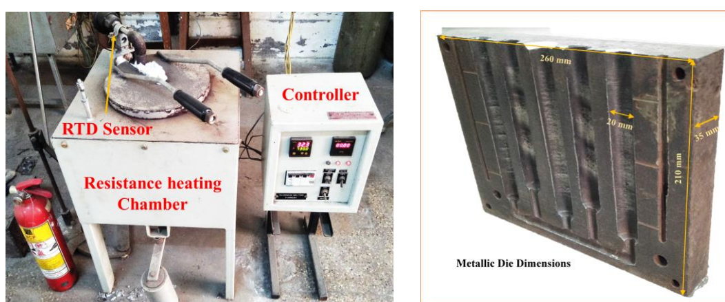
Figure 3.3 Experimental set-up for melting Al7075 (left), and metallic die with dimensions to pour liquid melt.
