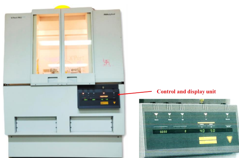
Figure 3.15 XRD analysis Malvern PANalytical X'Pert Pro machine.
