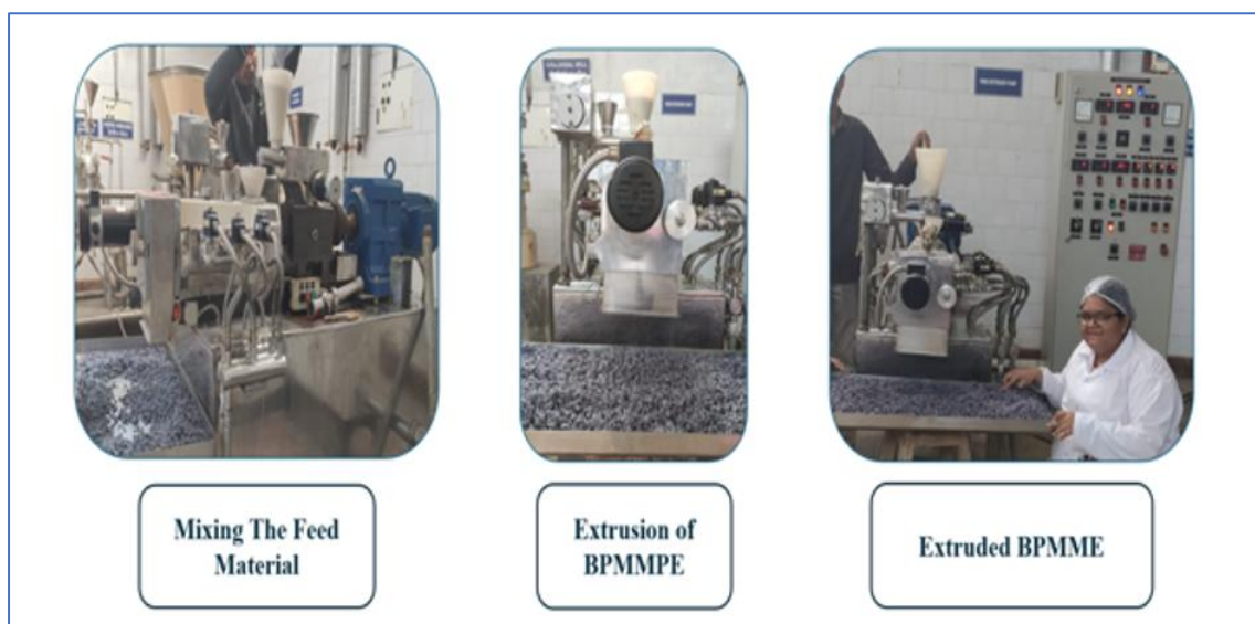
Figure 3.4 Extrusion of BPMMPPE
