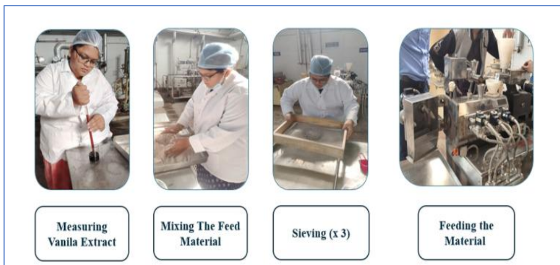
Figure 3.3 Preparation of Feed Material for Extrusion of BPMMPPE
